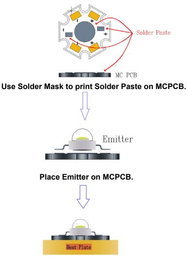
Put MCPCB on Heat Plate until Solder Paste melt. Put Emitter on MCPCB. Take the MCPCB out The Solder Paste sould be melted within 10 seconds. from Heat Plate within 10 seconds. Take out MCPCB out from Heat Plate within 10 seconds.
