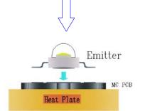
Put Emitter on MCPCB. Take the MCPCB out from Heat Plate within 10 seconds.
