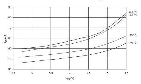
Figure 259. Programming Current vs.  $V_{CC}$
