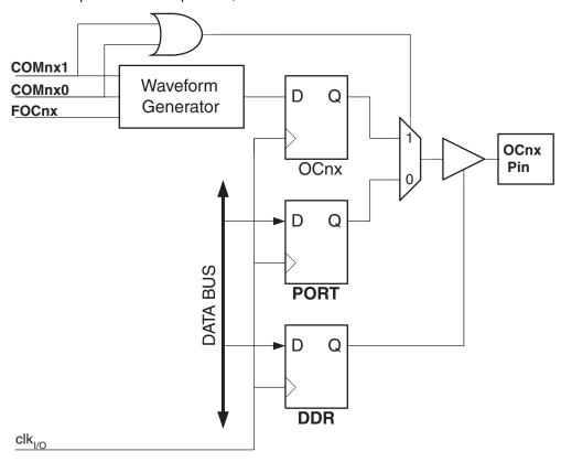
Figure 50. Compare Match Output Unit, Schematic
