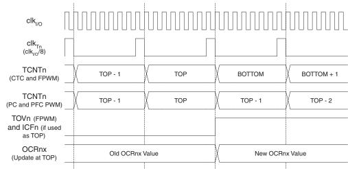
Figure 58. Timer/Counter Timing Diagram, with Prescaler ( $f_{\text{clk\_I/O}}/8$ )
