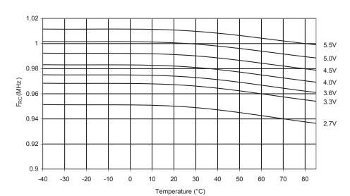
Figure 202. Calibrated 1 MHz RC Oscillator Frequency vs. Temperature
