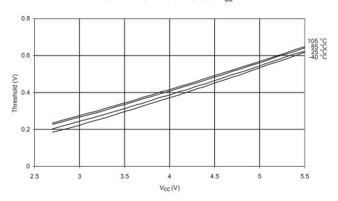
**Figure 244.** Reset Input Threshold Voltage vs.  $V_{CC}$  ( $V_{IH}$ , Reset Pin Read as '1')
