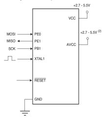
Notes: 1. If the device is clocked by the internal Oscillator, it is no need to connect a clock source to the XTAL1 pin.
