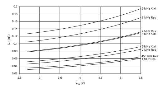
Figure 181. Standby Supply Current vs.  $V_{CC}$  (CKOPT Programmed)
