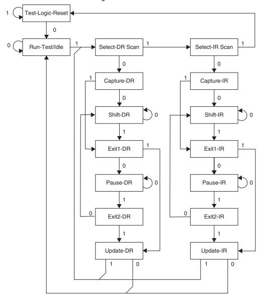
Figure 124. TAP Controller State Diagram
