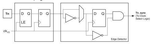
The synchronization and edge detector logic introduces a delay of 2.5 to 3.5 system clock cycles from an edge has been applied to the Tn pin to the counter is updated.
