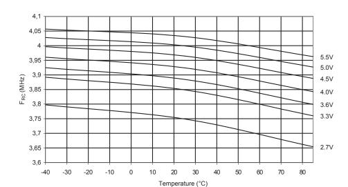
Figure 208. Calibrated 4 MHz RC Oscillator Frequency vs. Temperature
