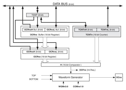
Figure 49. Output Compare Unit, Block Diagram
