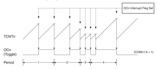
An interrupt can be generated each time the counter value reaches the TOP value by using the OCF0 flag. If the interrupt is enabled, the interrupt handler routine can be used for updating the TOP value. However, changing the TOP to a value close to BOTTOM when the counter is running with none or a low prescaler value must be done with care since the CTC mode does not have the double buffering feature. If the new value written to OCR0 is lower than the current
