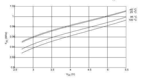
Figure 250. 1 kHz RC Oscillator Frequency vs. Oscillator
