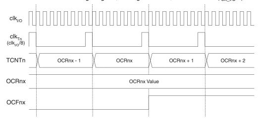
Figure 57 shows the count sequence close to TOP in various modes. When using phase and frequency correct PWM mode the OCRnx Register is updated at BOTTOM. The timing diagrams will be the same, but TOP should be replaced by BOTTOM, TOP-1 by BOTTOM+1 and so on. The same renaming applies for modes that set the TOVn flag at BOTTOM.
