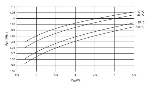
Figure 248. 8 MHz RC Oscillator Frequency vs.  $V_{\rm CC}$
