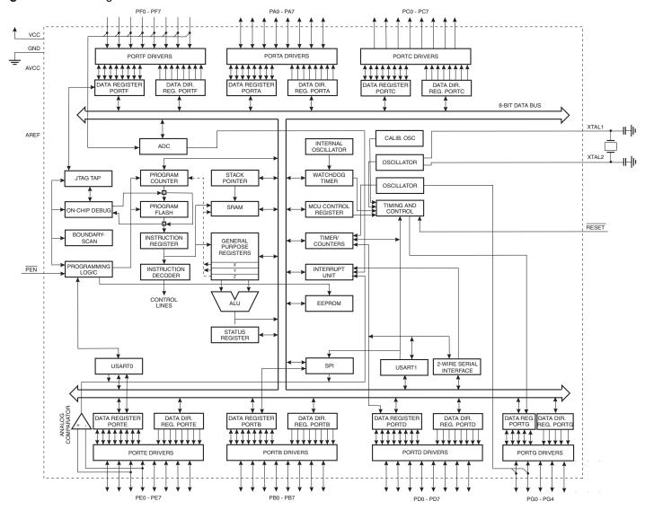
The AVR core combines a rich instruction set with 32 general purpose working registers. All the 32 registers are directly connected to the Arithmetic Logic Unit (ALU), allowing two independent registers to be accessed in one single instruction executed in one clock cycle. The resulting architecture is more code efficient while achieving throughputs up to ten times faster than conventional CISC microcontrollers.
