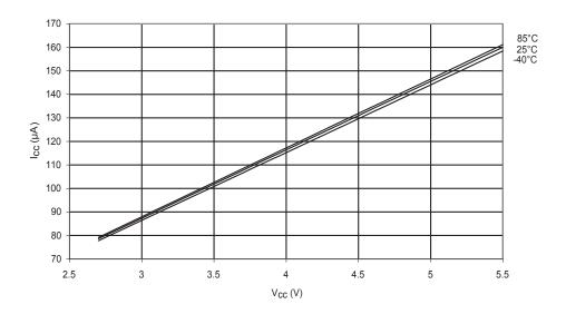
Figure 217. Analog Comparator Current vs.  $V_{\rm CC}$
