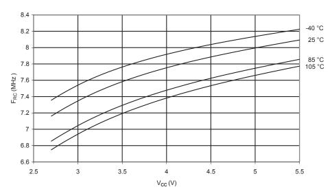
Figure 249. 1 MHz RC Oscillator Frequency vs. Vcc
