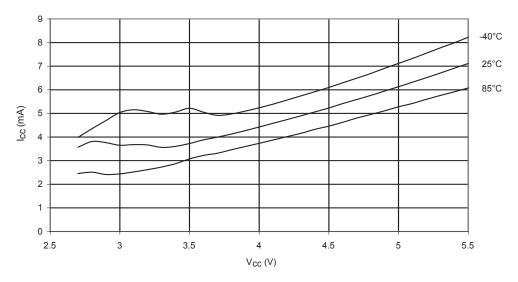
Current Consumption in Reset and Reset Pulse width
