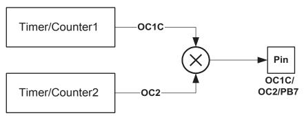
When the modulator is enabled, the two Output Compare channels are modulated together as shown in the block diagram (Figure 72).
