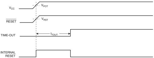
Figure 24. MCU Start-up, RESET Extended Externally
