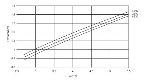
Figure 194. I/O Pin Input Hysteresis vs.  $V_{\text{CC}}$
