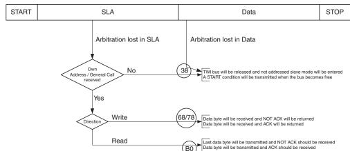
Figure 106. Possible Status Codes Caused by Arbitration
