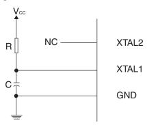
The Oscillator can operate in four different modes, each optimized for a specific frequency range. The operating mode is selected by the fuses CKSEL3..0 as shown in Table 11.
