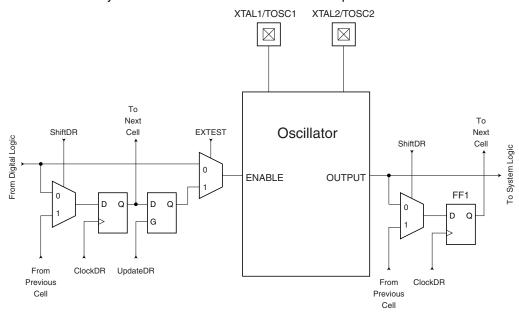
Table 102 summaries the scan registers for the external clock pin XTAL1, oscillators with XTAL1/XTAL2 connections as well as 32 kHz Timer Oscillator.
