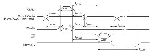
Figure 145. Parallel Programming Timing, Loading Sequence with Timing Requirements<sup>(1)</sup>
