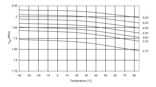
Figure 206. Calibrated 2 MHz RC Oscillator Frequency vs.  $V_{\rm CC}$
