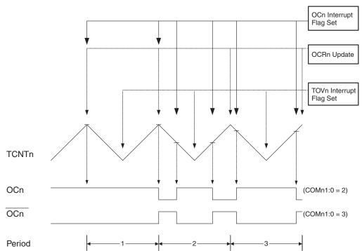
Figure 67. Phase Correct PWM Mode, Timing Diagram
