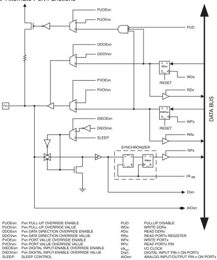
Note: 1. WPx, WDx, RLx, RPx, and RDx are common to all pins within the same port. clk<sub>I/O</sub>, SLEEP, and PUD are common to all ports. All other signals are unique for each pin.
