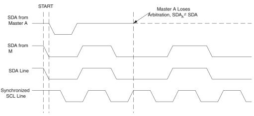
Figure 93. Arbitration between Two Masters
