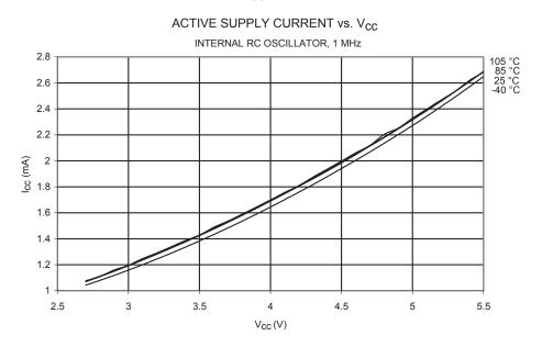
Figure 226. Active Supply Current vs.  $V_{\text{CC}}$  (Internal RC Oscillator, 1 kHz)
