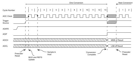
Figure 114. ADC Timing Diagram, Free Running Conversion
