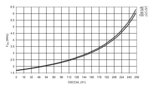
Figure 254. 8 MHz RC Oscillator Frequency vs. Osccal
