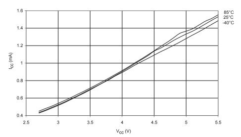
Figure 172. Idle Supply Current vs.  $V_{\text{CC}}$  (Internal RC Oscillator, 1 MHz)
