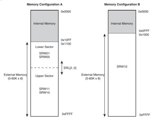
Note: 1. ATmega64 in non ATmega103 compatibility mode: Memory Configuration A is available (Memory Configuration B N/A).
