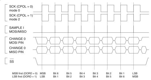
Figure 78. SPI Transfer Format with CPHA = 1
