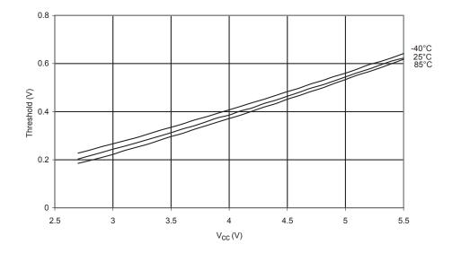
Figure 195. Reset Input Threshold Voltage vs. V<sub>CC</sub> (VIH, Reset Pin Read as '1')
