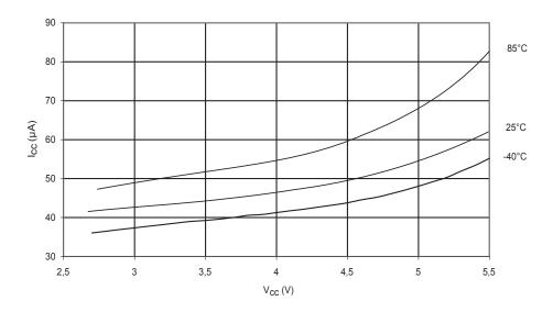
Figure 218. Programming Current vs.  $V_{\rm CC}$
