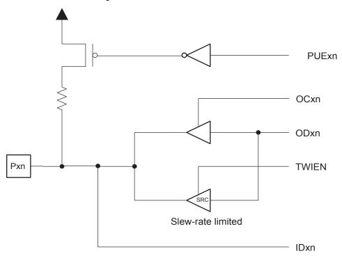
Figure 129. Additional Scan Signal for the Two-wire Interface
