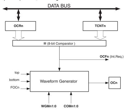
Figure 63. Output Compare Unit, Block Diagram
