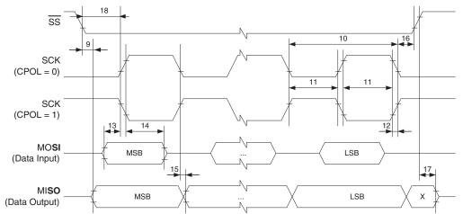
Figure 158. SPI Interface Timing Requirements (Slave Mode)
