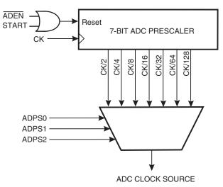
By default, the successive approximation circuitry requires an input clock frequency between 50 kHz and 200 kHz to get maximum resolution. If a lower resolution than 10 bits is needed, the input clock frequency to the ADC can be higher than 200 kHz to get a higher sample rate.
