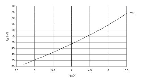
Figure 176. Idle Supply Current vs.  $V_{\text{CC}}$  (32 kHz External Oscillator)
