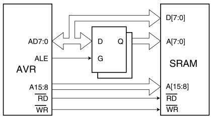
Pull-up and Bus Keeper The pull-ups on the AD7:0 ports may be activated if the corresponding Port Register is written to one. To reduce power consumption in sleep mode, it is recommended to disable the pull-ups by writing the Port Register to zero before entering sleep.
