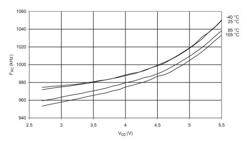
Figure 247. Calibrated 4 MHz RC Oscillator Frequency vs.  $V_{\rm CC}$
