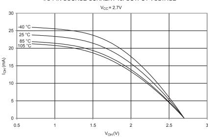
I/O PIN SOURCE CURRENT vs. OUTPUT VOLTAGE
