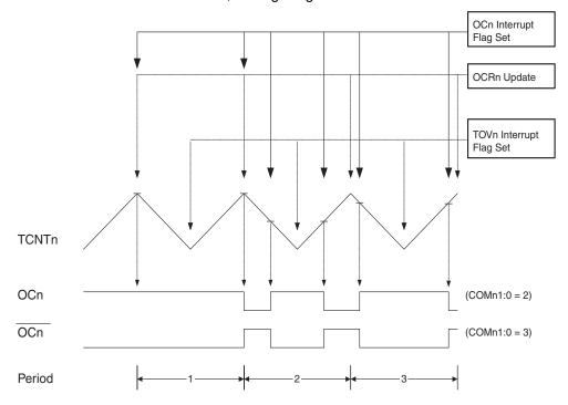
Figure 40. Phase Correct PWM Mode, Timing Diagram
