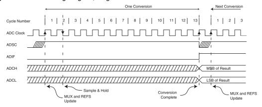
Figure 113. ADC Timing Diagram, Auto Triggered Conversion
