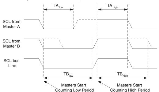
Figure 92. SCL Synchronization between Multiple Masters
