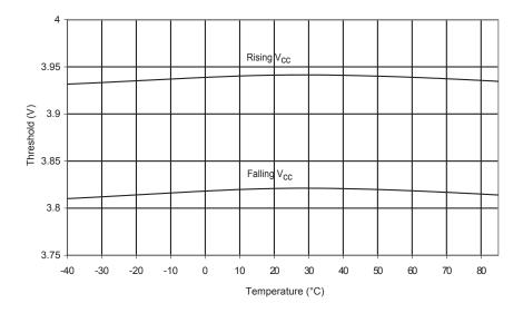
Figure 199. BOD Thresholds vs. Temperature (BODLEVEL is 2.7V)
