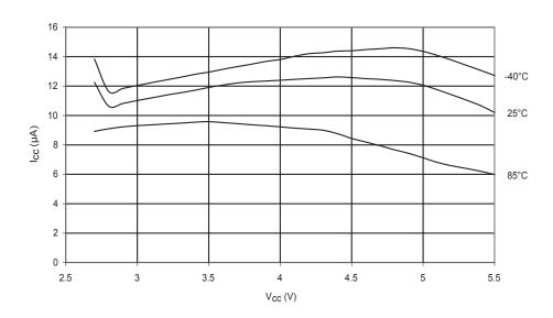
Figure 215. ADC Current vs.  $V_{CC}$  (ADC CLK = 50 kHz)
