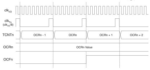
Figure 71 shows the setting of OCF2 and the clearing of TCNT2 in CTC mode.
