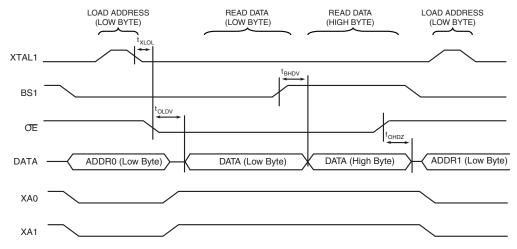
Note: 1. The timing requirements shown in Figure 144 (that is, t<sub>DVXH</sub>, t<sub>XHXL</sub>, and t<sub>XLDX</sub>) also apply to reading operation.
