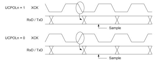
The UCPOLn bit UCRSnC selects which XCK clock edge is used for data sampling and which is used for data change. As Figure 81 shows, when UCPOLn is zero the data will be changed at rising XCK edge and sampled at falling XCK edge. If UCPOLn is set, the data will be changed at falling XCK edge and sampled at rising XCK edge.
