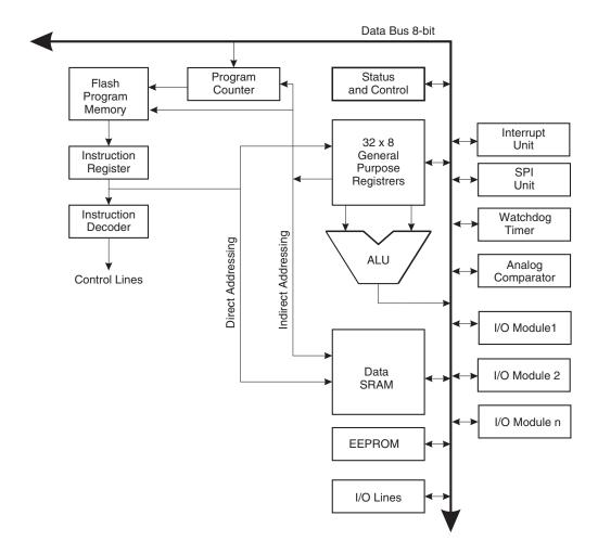
In order to maximize performance and parallelism, the AVR uses a Harvard architecture – with separate memories and buses for program and data. Instructions in the program memory are executed with a single level pipelining. While one instruction is being executed, the next instruction is pre-fetched from the program memory. This concept enables instructions to be executed in every clock cycle. The program memory is In-System Reprogrammable Flash memory.
