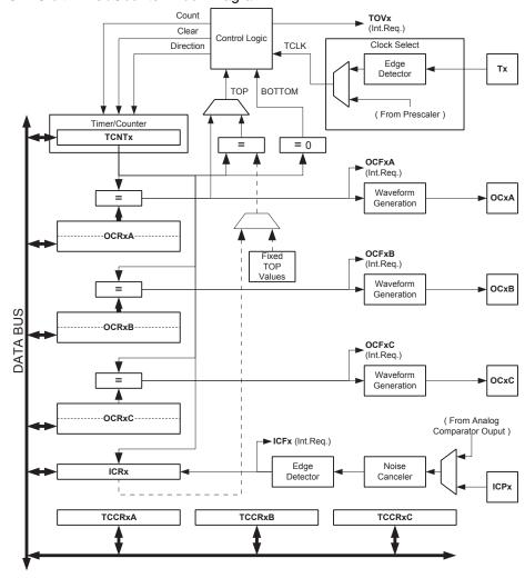
Figure 46. 16-bit Timer/Counter Block Diagram<sup>(1)</sup>
