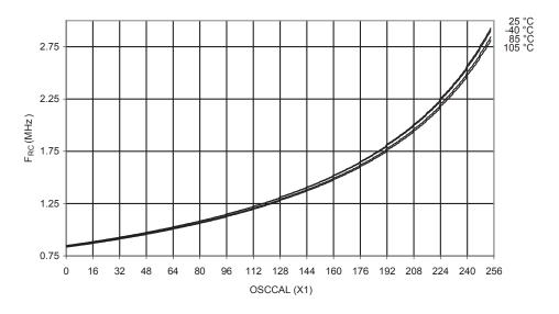
Figure 253. 4 MHz RC Oscillator Frequency vs. Osccal
