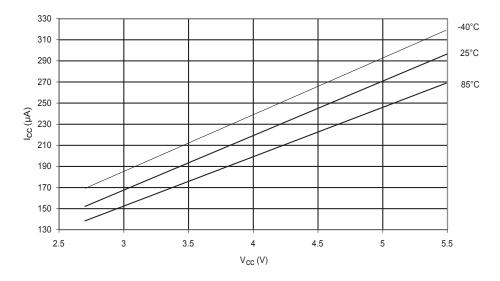
Figure 216. Aref Current vs.  $V_{\text{CC}}$
