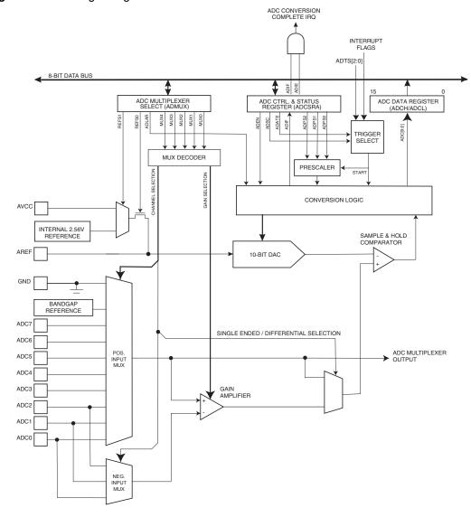
Figure 108. Analog to Digital Converter Block Schematic
