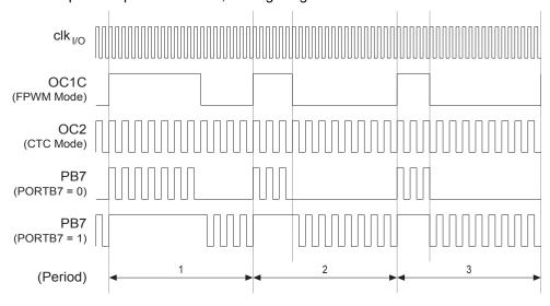
Figure 74. Output Compare Modulator, Timing Diagram
