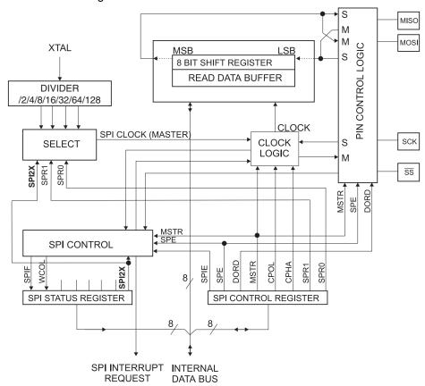
Note: 1. Refer to Figure 1 on page 2, and Table 30 on page 74 for SPI pin placement.
