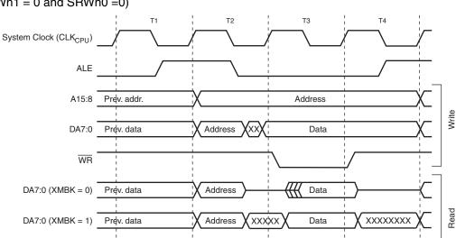
**Figure 13.** External Data Memory Cycles without Wait State<sup>(1)</sup> (SRWn1 = 0 and SRWn0 =0)
