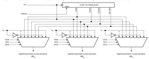
Note: 1. The synchronization logic on the input pins (T3/T2/T1) is shown in Figure 59.
