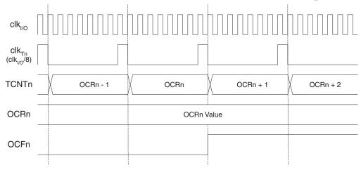
Figure 44 shows the setting of OCF0 and the clearing of TCNT0 in CTC mode.
