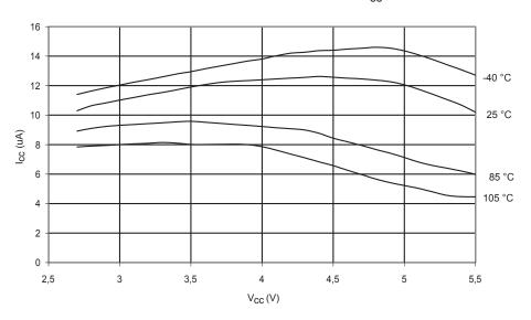
Figure 257. ADC Current vs. V<sub>CC</sub>
