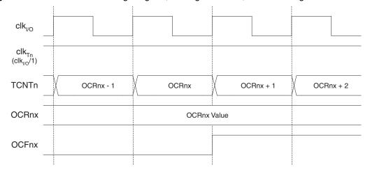
Figure 56 shows the same timing data, but with the prescaler enabled.
