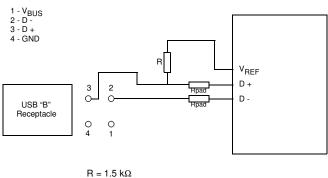
$R = 1.5 \text{ k}\Omega$  $R_{pad} = 27\Omega$
