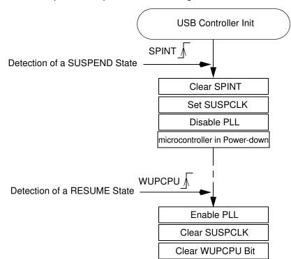
Figure 66. Example of a Suspend/Resume Management
