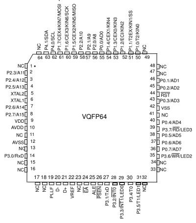
Figure 2. AT89C5131A-L 64-pin VQFP Pinout
