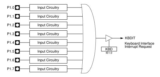
Figure 41. Keyboard Input Circuitry
