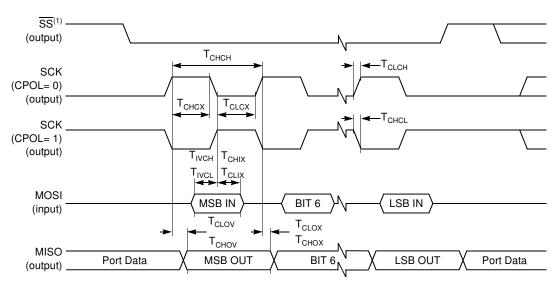
SS handled by software using general purpose port pin.
