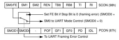
When this feature is enabled, the receiver checks each incoming data frame for a valid stop bit. An invalid stop bit may result from noise on the serial lines or from simultaneous transmission by two CPUs. If a valid stop bit is not found, the Framing Error bit (FE) in SCON register (See Table 56) bit is set.
