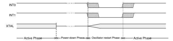
Exit from power-down by reset redefines all the SFRs, exit from power-down by external interrupt does no affect the SFRs.
