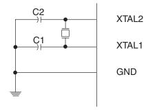
The Low Power Oscillator can operate in three different modes, each optimized for a specific frequency range. The operating mode is selected by the fuses CKSEL3..1 as shown in Table 8-3 on page 29.
