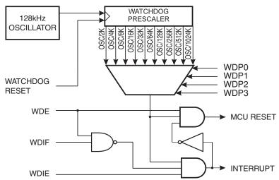
ATmega48/88/168 has an Enhanced Watchdog Timer (WDT). The WDT is a timer counting cycles of a separate on-chip 128 kHz oscillator. The WDT gives an interrupt or a system reset when the counter reaches a given time-out value. In normal operation mode, it is required that the system uses the WDR - Watchdog Timer Reset - instruction to restart the counter before the time-out value is reached. If the system doesn't restart the counter, an interrupt or system reset will be issued.
