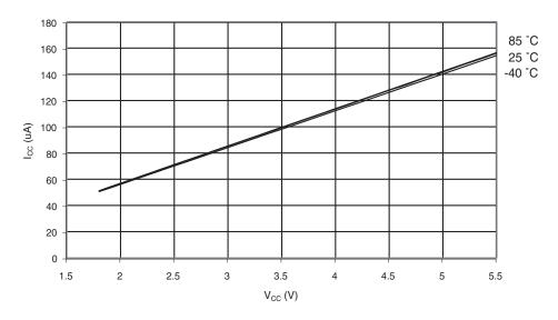
Figure 29-47. Analog Comparator Current vs.  $V_{\text{CC}}$
