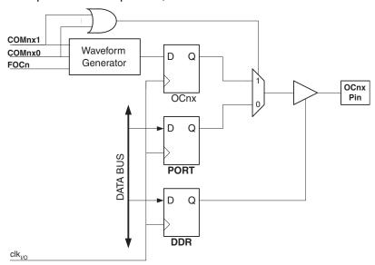
Figure 14-4. Compare Match Output Unit, Schematic
