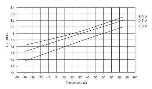
Figure 29-42. Calibrated 8 MHz RC Oscillator Frequency vs.  $V_{\rm CC}$
