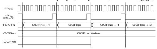
Figure 17-11 shows the setting of OCF2A and the clearing of TCNT2 in CTC mode.
