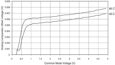
Figure 29-39. Analog Comparator Offset Voltage vs. Common Mode Voltage (V<sub>CC</sub>=2.7V)
