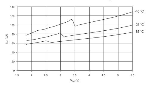
Figure 29-48. Programming Current vs.  $V_{CC}$
