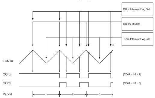
Figure 14-7. Phase Correct PWM Mode, Timing Diagram
