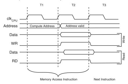
Figure 7-4. On-chip Data SRAM Access Cycles
