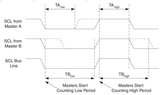
Figure 21-7. SCL Synchronization Between Multiple Masters
