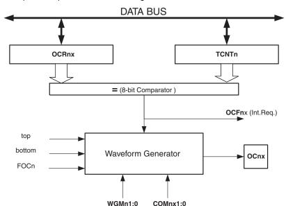
Figure 14-3. Output Compare Unit, Block Diagram
