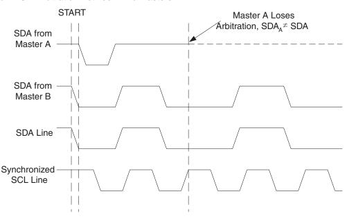
Figure 21-8. Arbitration Between Two Masters
