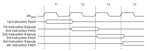
Figure 6-5 shows the internal timing concept for the Register File. In a single clock cycle an ALU operation using two register operands is executed, and the result is stored back to the destination register.
