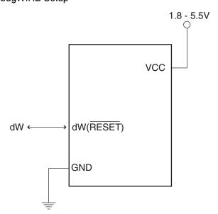
Figure 24-1 shows the schematic of a target MCU, with debugWIRE enabled, and the emulator connector. The system clock is not affected by debugWIRE and will always be the clock source selected by the CKSEL Fuses.
