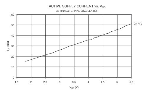
Figure 29-6. Active Supply Current vs.  $V_{CC}$  (32 kHz External Oscillator)
