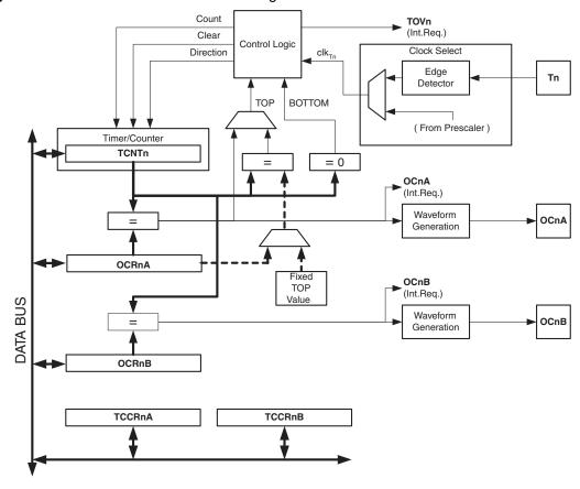
Figure 14-1. 8-bit Timer/Counter Block Diagram
