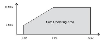
Figure 28-2. Maximum Frequency vs.  $V_{CC}$ , ATmega48/88/168
