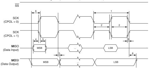
Figure 28-5. SPI Interface Timing Requirements (Master Mode)
