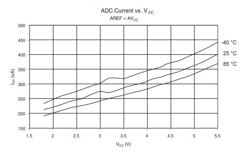
Figure 29-46. AREF External Reference Current vs.  $V_{\rm CC}$
