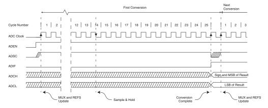
Figure 23-5. ADC Timing Diagram, Single Conversion
