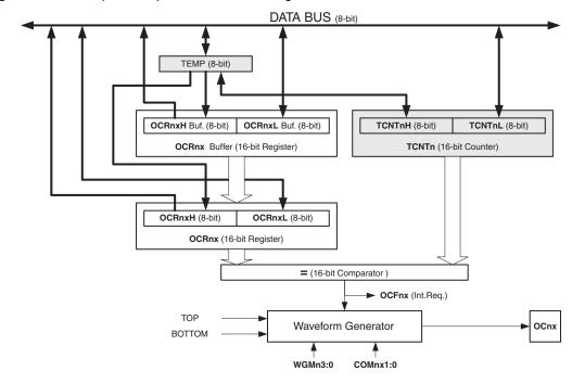
Figure 15-4. Output Compare Unit, Block Diagram
