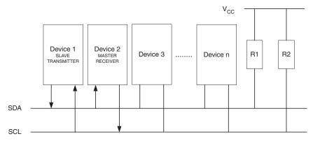
To initiate the Slave Transmitter mode, TWAR and TWCR must be initialized as follows:
