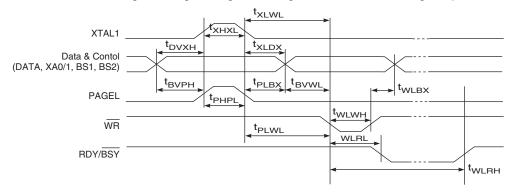
Figure 28-8. Parallel Programming Timing, Loading Sequence with Timing Requirements<sup>(1)</sup>
