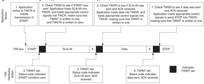
The first step in a TWI transmission is to transmit a START condition. This is done by writing a specific value into TWCR, instructing the TWI hardware to transmit a START
