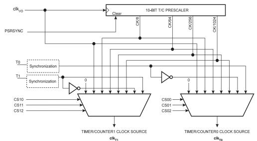
Figure 16-2. Prescaler for Timer/Counter0 and Timer/Counter1<sup>(1)</sup>
