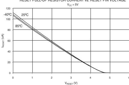
RESET PULL-UP RESISTOR CURRENT vs. RESET PIN VOLTAGE
