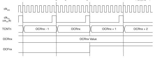
Figure 14-11 shows the setting of OCF0A and the clearing of TCNT0 in CTC mode and fast PWM mode where OCR0A is TOP.
