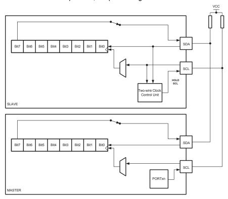
Figure 21-4. Two-wire Mode Operation, Simplified Diagram
