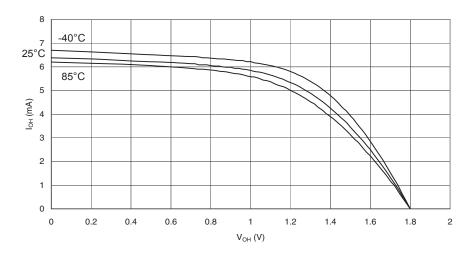
Figure 29-24. I/O Pin Source Current vs. Output Voltage, Port B ( $V_{CC}$ = 5V)
