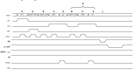
Figure 27-4. Programming the EEPROM Waveforms
