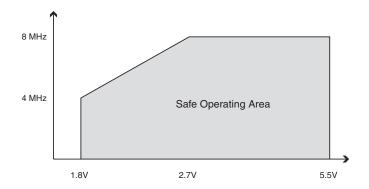
Figure 28-2. Maximum Frequency vs. V<sub>CC</sub> (8 - 16 MHz).
