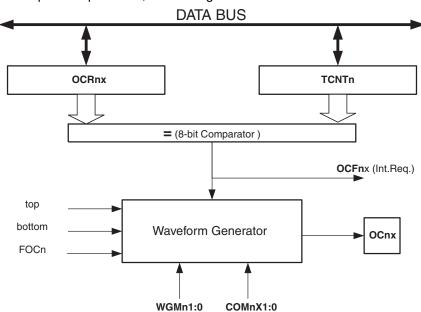
Figure 18-3. Output Compare Unit, Block Diagram
