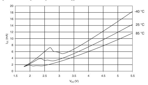
Figure 29-55. Programming Current vs. V<sub>CC</sub>
