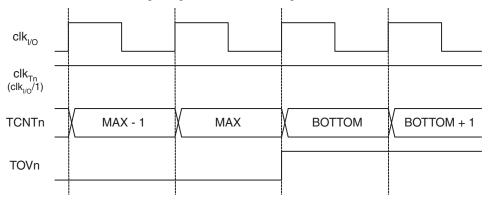
Figure 18-8 shows the same timing data, but with the prescaler enabled.
