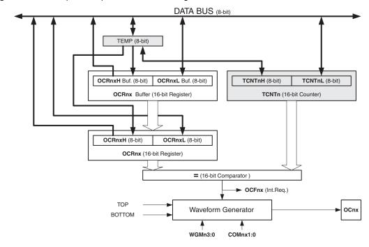
Figure 17-4. Output Compare Unit, Block Diagram
