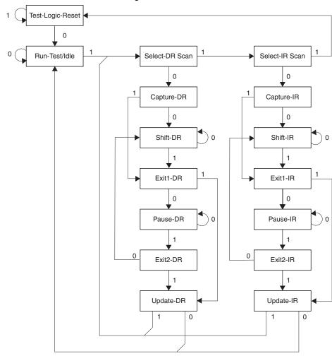
Figure 24-2. TAP Controller State Diagram
