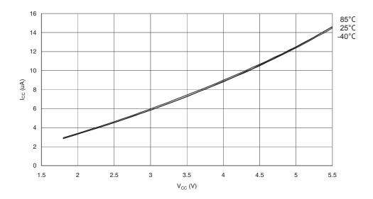
Figure 29-54. Analog Comparator Current vs.  $V_{\rm CC}$
