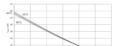
Figure 29-19. Reset Pull-up Resistor Current vs. Reset Pin Voltage ( $V_{CC} = 2.7V$ )
