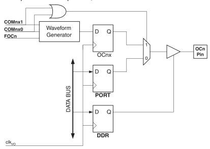
Figure 15-4. Compare Match Output Unit, Schematic
