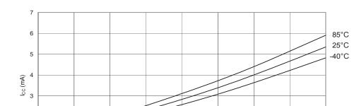
Figure 29-8. Idle Supply Current vs. V<sub>CC</sub> (Internal RC Oscillator, 8 MHz)
