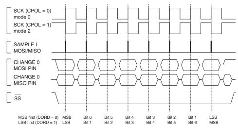
Figure 19-3. SPI Transfer Format with CPHA = 0
