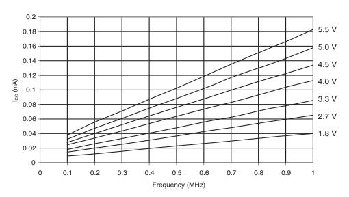
**Figure 29-57.** Reset Supply Current vs. V<sub>CC</sub> (1 - 16MHz, Excluding Current Through The Reset Pull-up)
