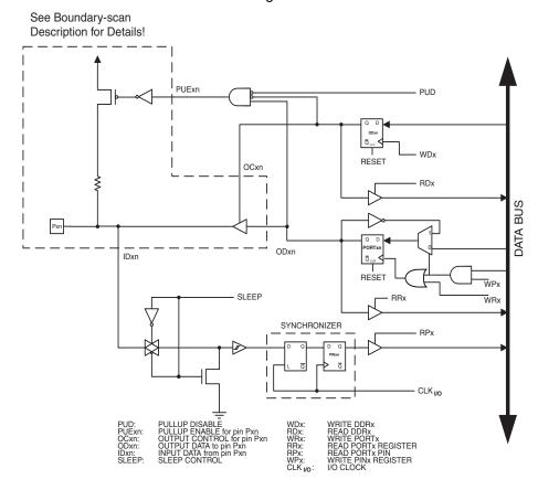
Figure 25-4. General Port Pin Schematic Diagram
