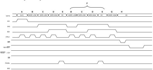
Figure 27-3. Programming the Flash Waveforms<sup>(1)</sup>
