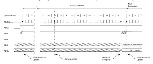
Figure 23-5. ADC Timing Diagram, Single Conversion
