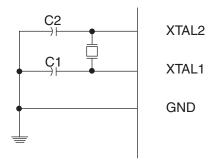
The Oscillator can operate in three different modes, each optimized for a specific frequency range. The operating mode is selected by the fuses CKSEL3..1 as shown in Table 9-3 on page 28.
