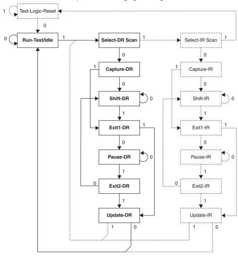
Figure 27-15. State Machine Sequence for Changing/Reading the Data Word
