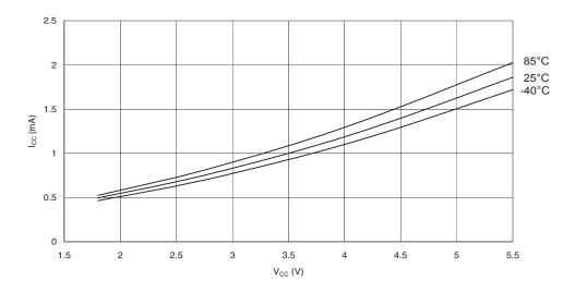
Figure 29-5. Active Supply Current vs. V<sub>CC</sub> (32kHz External Oscillator)
