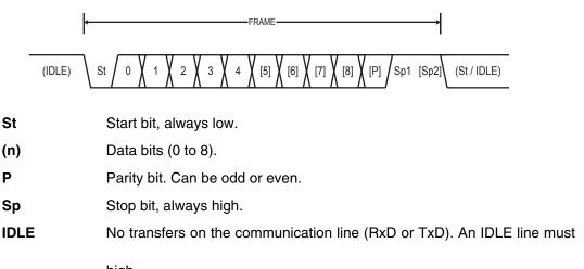
The frame format used by the USART is set by the UCSZn2:0, UPMn1:0 and USBSn bits in UCSRnB and UCSRnC. The Receiver and Transmitter use the same setting. Note that changing the setting of any of these bits will corrupt all ongoing communication for both the Receiver and Transmitter.
