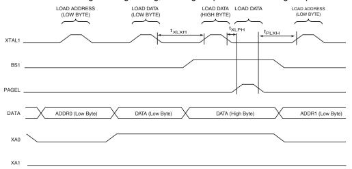
Note: 1. The timing requirements shown in Figure 27-7 (i.e., t<sub>DVXH</sub>, t<sub>XHXL</sub>, and t<sub>XLDX</sub>) also apply to loading operation.
