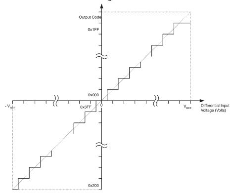
Figure 23-14. Differential Measurement Range
