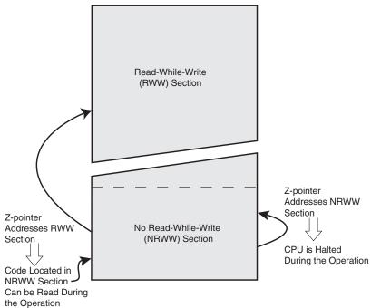
Figure 26-1. Read-While-Write vs. No Read-While-Write
