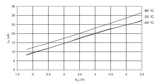
Figure 29-10. Idle Supply Current vs. V<sub>CC</sub> (32kHz External Oscillator)
