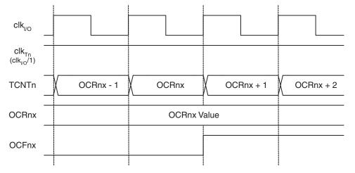
Figure 17-11 shows the same timing data, but with the prescaler enabled.
