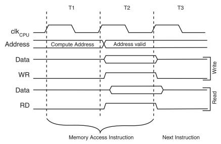
Figure 8-3. On-chip Data SRAM Access Cycles
