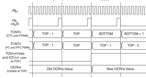
Figure 17-13. Timer/Counter Timing Diagram, with Prescaler (f<sub>clk 1/O</sub>/8)
