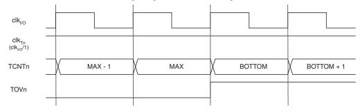
Figure 15-9 shows the same timing data, but with the prescaler enabled.
