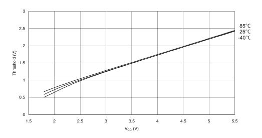
Figure 29-35. I/O Pin Input Hysteresis vs.  $V_{\text{CC}}$
