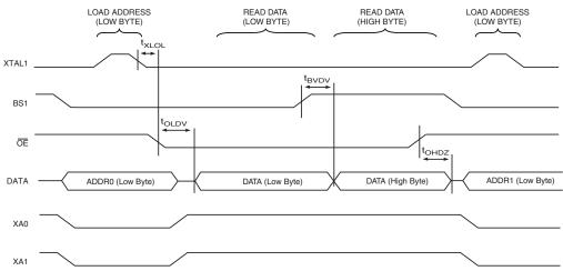
Note: 1. The timing requirements shown in Figure 27-7 (i.e., t<sub>DVXH</sub>, t<sub>XHXL</sub>, and t<sub>XLDX</sub>) also apply to reading operation.
