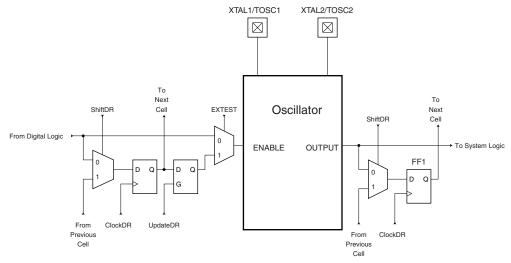
Table 25-3 summaries the scan registers for the external clock pin XTAL1, oscillators with XTAL1/XTAL2 connections as well as 32kHz Timer Oscillator.
