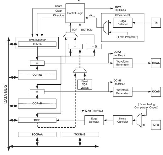
Figure 17-1. 16-bit Timer/Counter Block Diagram<sup>(1)</sup>
