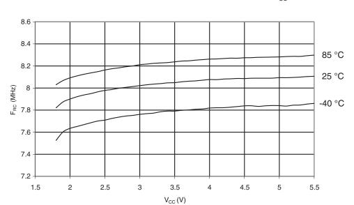
Figure 29-47. Calibrated 8MHz RC Oscillator Frequency vs.  $V_{\text{CC}}$
