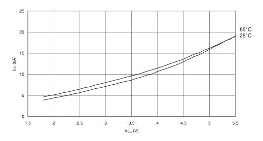
Figure 29-53. Watchdog Timer Current vs.  $V_{\text{CC}}$
