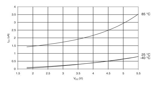
Figure 29-12. Power-down Supply Current vs. V<sub>CC</sub> (Watchdog Timer Enabled)
