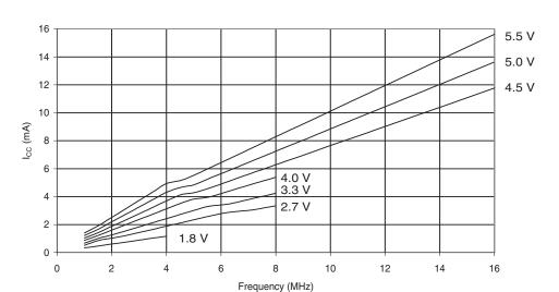
Figure 29-2. Active Supply Current vs. Frequency (1 - 16MHz))
