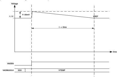
Figure 8-2. Voltage Reference Spike
