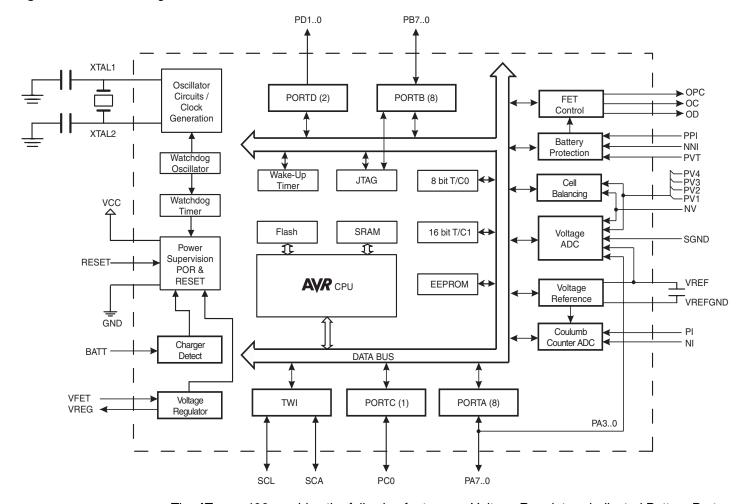
The ATmega406 provides the following features: a Voltage Regulator, dedicated Battery Protection Circuitry, integrated cell balancing FETs, high-voltage analog front-end, and an MCU with two ADCs with On-chip voltage reference for battery fuel gauging.
