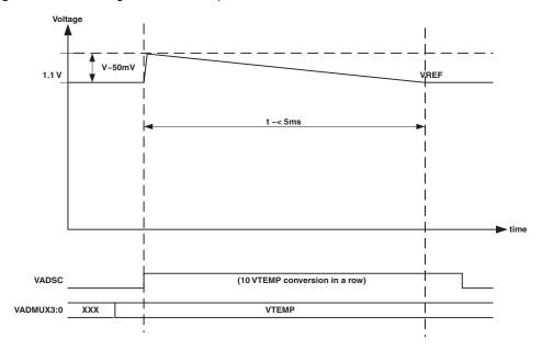
If the CC-ADC is doing current accumulation while the V-ADC is doing temperature measurement, both the Instantaneous and the Accumulated conversion results will be affected. The spike on VREF will be visible on 1 Accumulated Current (CADAC3...0) and 2 Instantaneous Current (CADIC1...0) conversion results.
