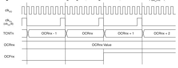
Figure 11-11 on page 69 shows the setting of OCF0A and the clearing of TCNT0 in CTC mode and fast PWM mode where OCR0A is TOP.
