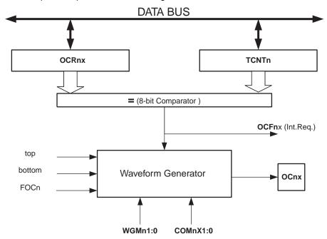
Figure 11-3. Output Compare Unit, Block Diagram
