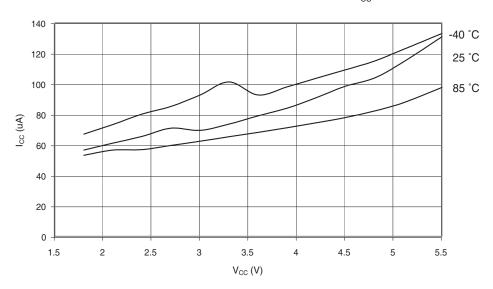
Figure 19-61. Programming Current vs.  $V_{\text{CC}}$
