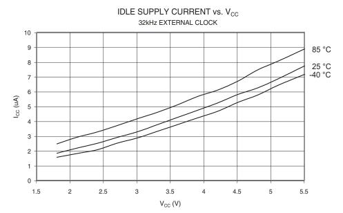
Figure 19-12. Idle Supply Current vs.  $V_{\text{CC}}$  (32 kHz External Clock)
