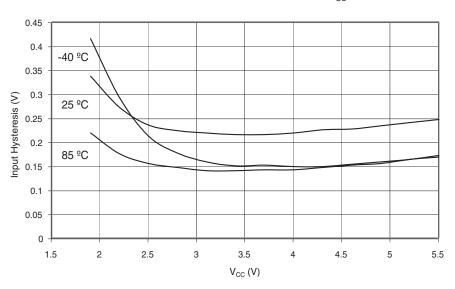
$\textbf{Figure 19-40.} \ \ \text{Reset Pin as I/O - Input Threshold Voltage vs. V}_{\text{CC}} \ \ (\text{VIH, Reset Pin Read as '1'})$
