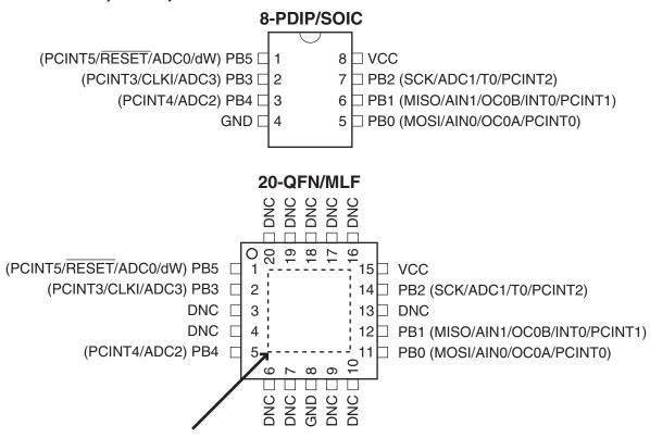
NOTE: Bottom pad should be soldered to ground.
