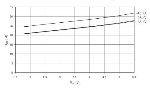
Figure 19-59. ADC Current vs. V<sub>CC</sub>
