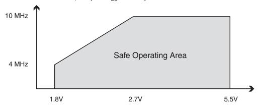
**Figure 18-2.** Maximum Frequency vs. V<sub>CC</sub> for ATtiny13
