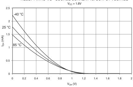
RESET PIN AS I/O - SOURCE CURRENT vs. OUTPUT VOLTAGE
