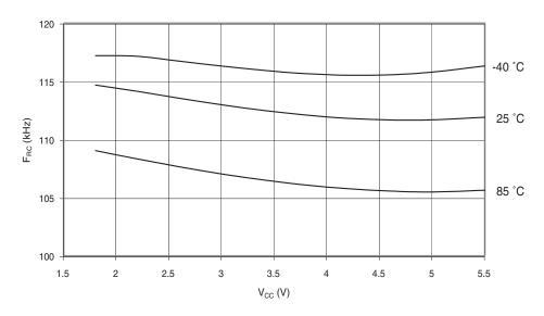
Figure 19-57. 128 kHz Watchdog Oscillator Frequency vs. Temperature
