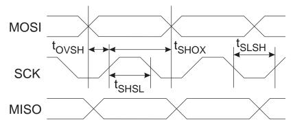
Figure 18-5. Serial Programming Waveform
