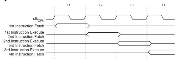
Figure 4-5 on page 12 shows the internal timing concept for the Register File. In a single clock cycle an ALU operation using two register operands is executed, and the result is stored back to the destination register.
