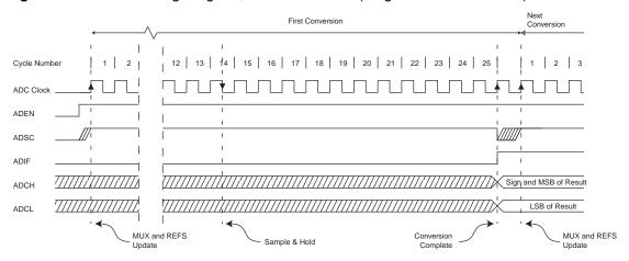
When the bandgap reference voltage is used as input to the ADC, it will take a certain time for the voltage to stabilize. If not stabilized, the first value read after the first conversion may be wrong.
