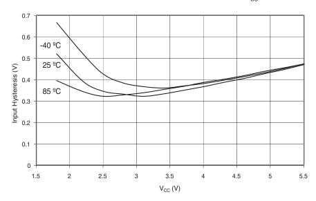
Figure 19-43. Reset Input Threshold Voltage vs.  $V_{CC}$  (VIH, Reset Pin Read as '1')
