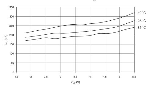
Figure 19-60. Analog Comparator Current vs.  $V_{\rm CC}$
