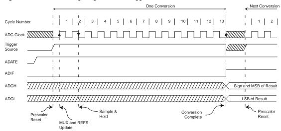
Figure 14-6. ADC Timing Diagram, Auto Triggered Conversion
