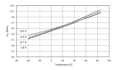
Figure 19-51. Calibrated 9.6 MHz RC Oscillator Frequency vs.  $V_{CC}$
