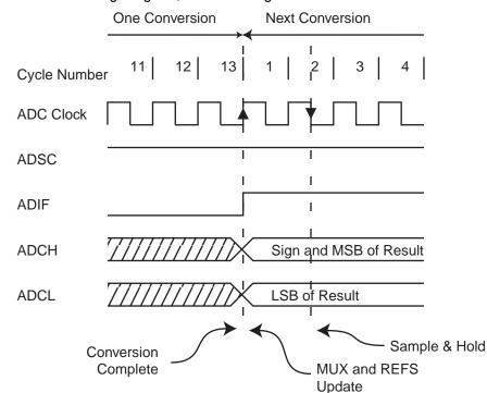
Figure 14-7. ADC Timing Diagram, Free Running Conversion
