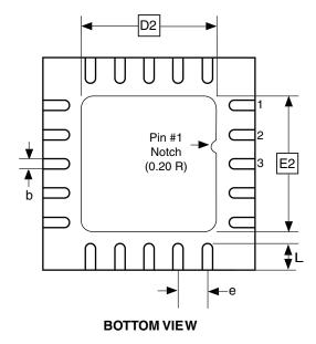
Note: Reference JEDEC Standard MO-220, Fig. 1 (SAW Singulation) WGGD-5.
