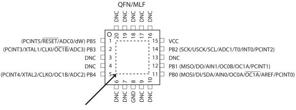
NOTE: Bottom pad should be soldered to ground.
