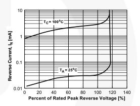
Figure 4. Reverse Current vs. Reverse Voltage
