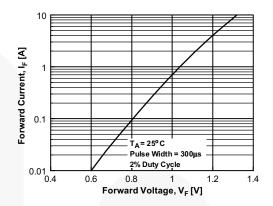
Figure 2. Forward Voltage Characteristics
