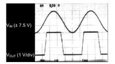
Figure 46. A ±7.5V Input Signal Greatly Exceeds the 3-V Supply in Figure 47 Causing No Phase Inversion Due to R<sub>1</sub>
