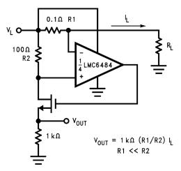
Figure 69. Positive Supply Current Sense
