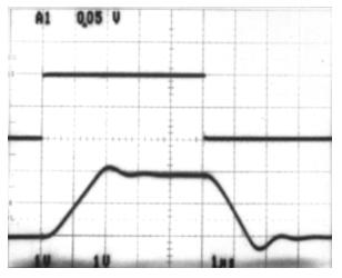
Figure 52. Pulse Response of LMC6484 Circuit in Figure 51
