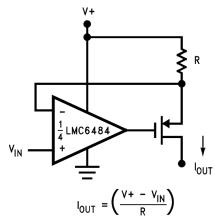
Figure 68. Large Compliance Range Current Source
