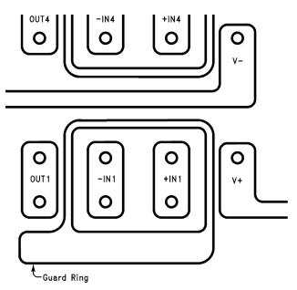
Figure 78. Example of Guard Ring in PCB Layout
