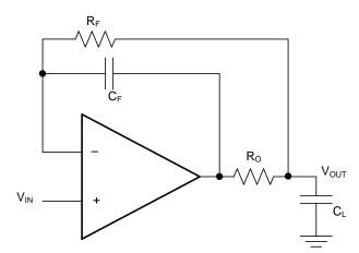
Figure 48. Unity Gain Buffer for High-Capacitive Loads
