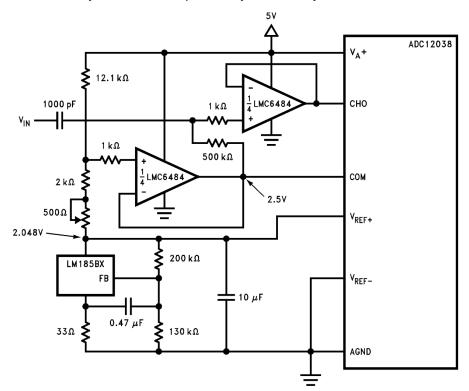
Figure 73. Operating from the Same Supply Voltage, the LMC6484 Buffers the ADC12038 Maintaining Excellent Accuracy
