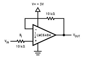
Figure 64. Half-Wave Rectifier with Input Current Protection (R<sub>I</sub>)
