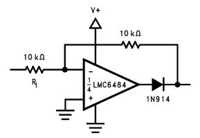
Figure 66. Full Wave Rectifier with Input Current Protection (R<sub>1</sub>)
