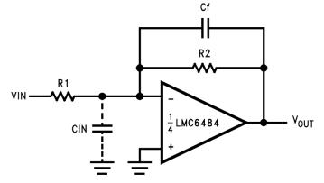
Figure 53. Canceling the Effect of Input Capacitance
