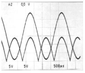
Figure 67. Full Wave Rectifier Waveform
