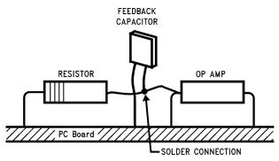
Note: (Input pins are lifted out of PC board and soldered directly to components. All other pins connected to PC board.)
