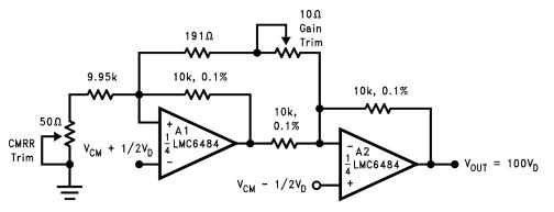
Figure 75. Low-Power 2-Opamp Instrumentation Amplifier
