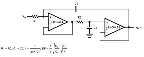
Figure 72. Rail-to-Rail Single Supply Low Pass Filter
