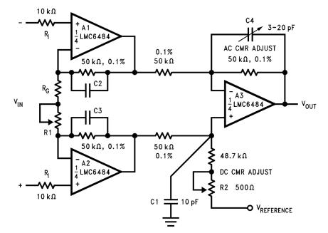
Figure 74. Low-Power 3-Opamp Instrumentation Amplifier
