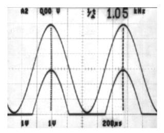
Figure 65. Half-Wave Rectifier Waveform
