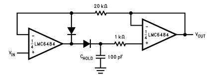
Figure 70. Low Voltage Peak Detector with Rail-to-Rail Peak Capture Range
