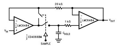
Figure 71. Rail-to-Rail Sample and Hold
