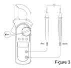
When DC voltage measurement has been completed, disconnect the connection between the testing leads and the circuit under test and remove testing leads from the input terminals
