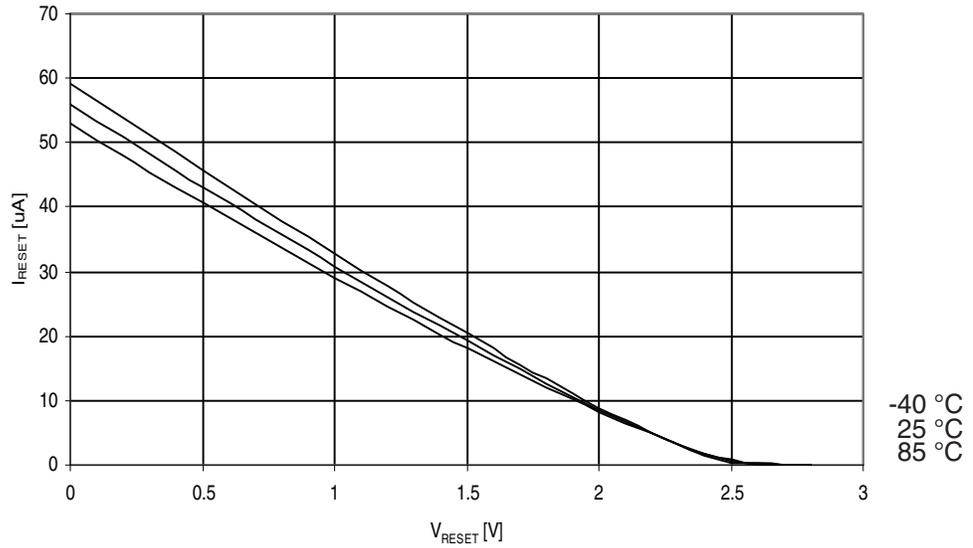
**Figure 30-325.** ATmega3290PA: Reset Pull-up Resistor Current vs. Reset Pin Voltage
