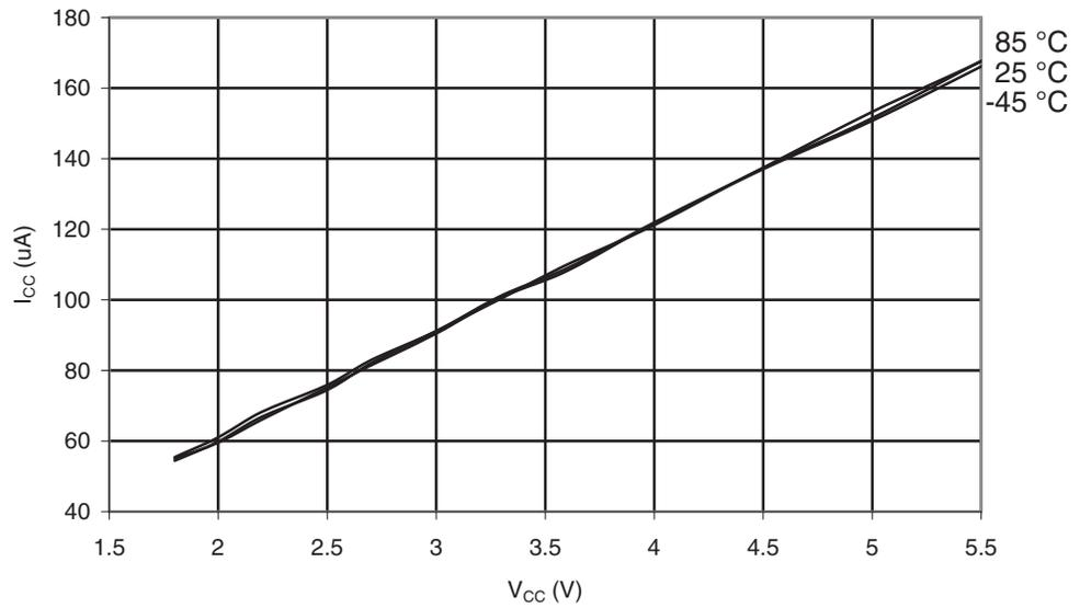
Figure 30-57. ATmega169A: Watchdog Timer Current vs.  $V_{CC}$
