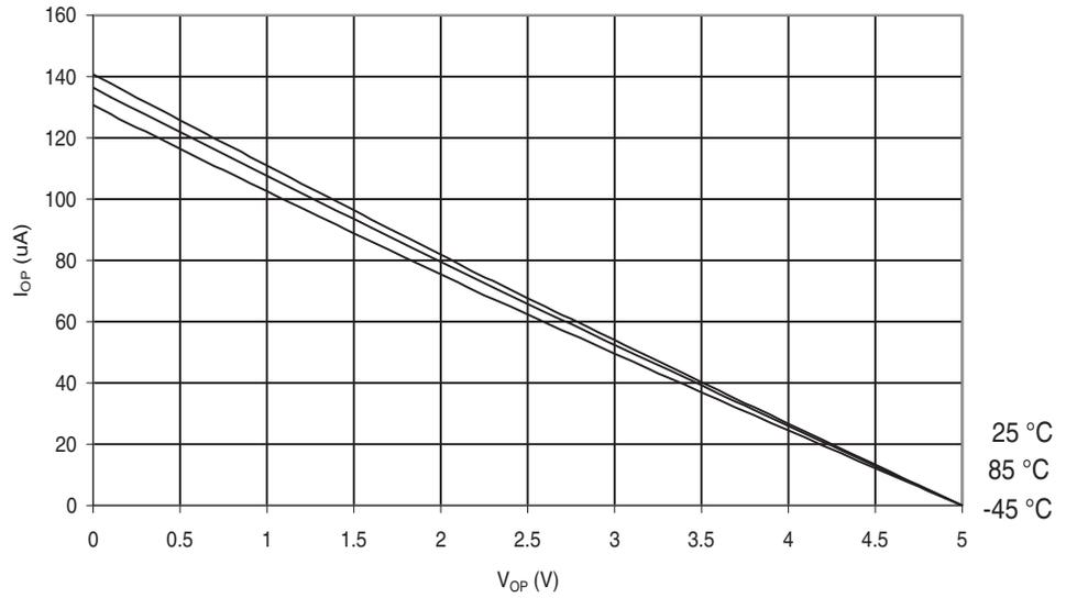
**Figure 30-565.** ATmega6490P: I/O Pin Pull-up Resistor Current vs. Input Voltage ( $V_{CC} = 2.7V$ )
