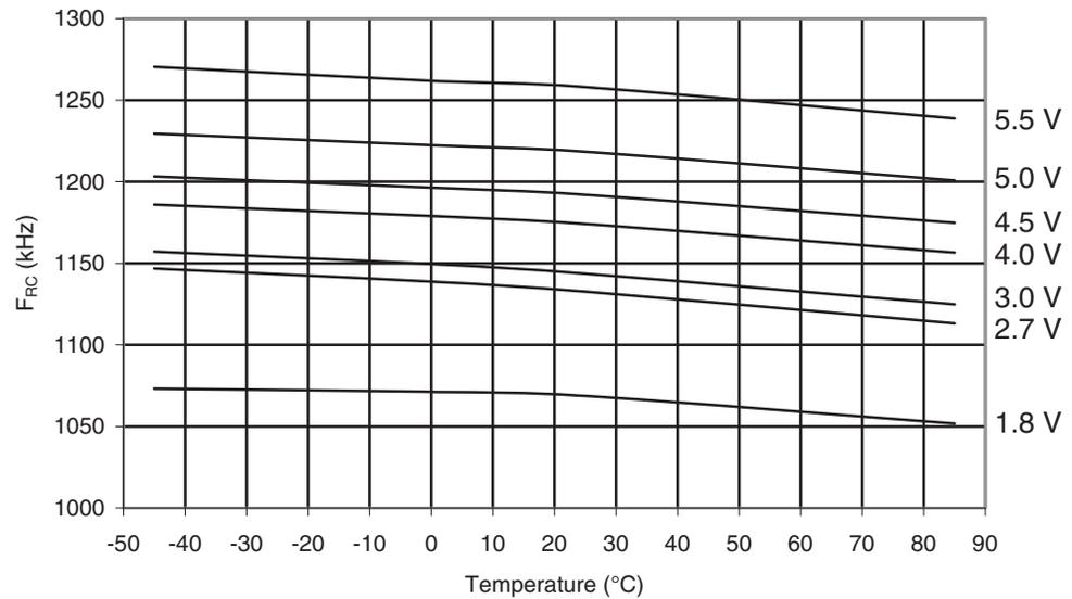
**Figure 30-111.** ATmega169PA: Calibrated 8MHz RC Oscillator Frequency vs. Temperature
