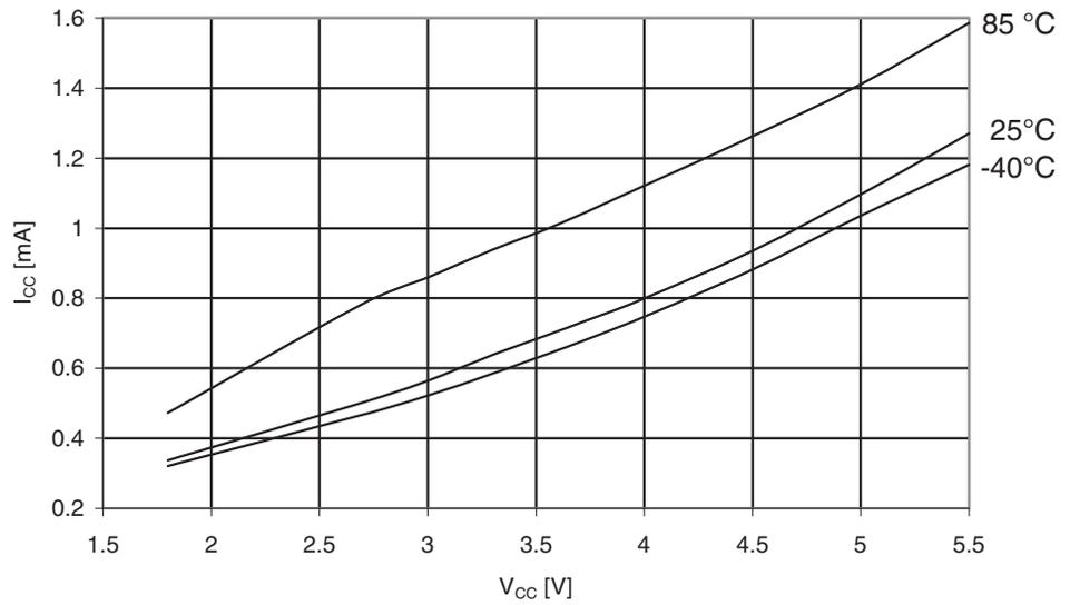
**Figure 30-249.** ATmega3290A: Active Supply Current vs.  $V_{CC}$  (32kHz Watch Crystal)
