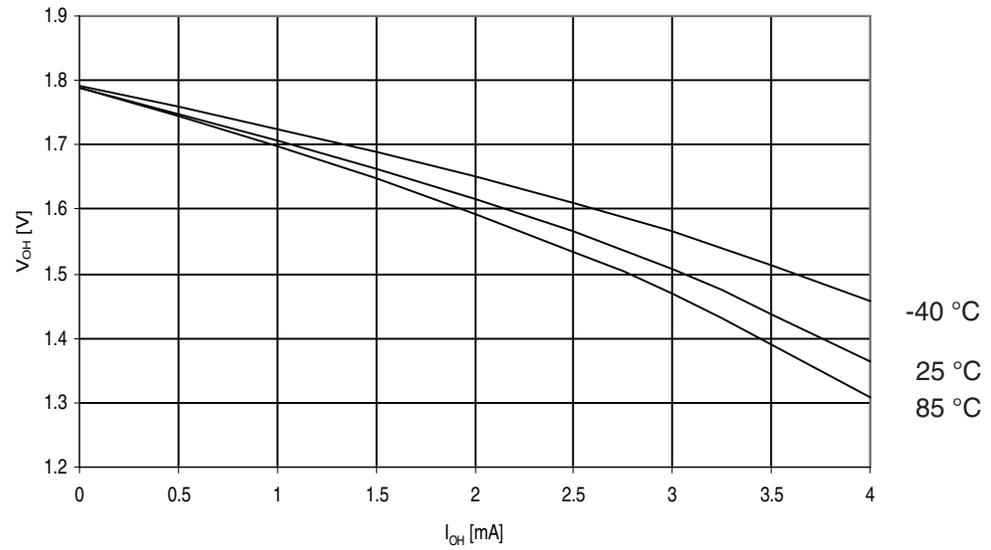
**Figure 30-269.** ATmega3290A: I/O Pin Output Voltage vs. Source Current, Port B ( $V_{CC} = 5V$ )
