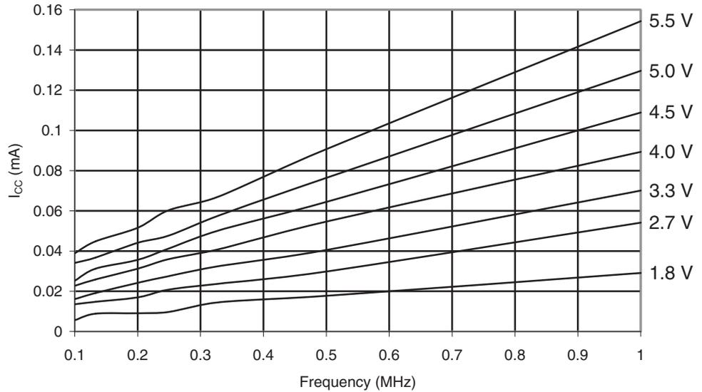
**Figure 30-61.** ATmega169A: Reset Supply Current vs.  $V_{CC}$  (1 - 16MHz, Excluding Current Through The Reset Pull-up)
