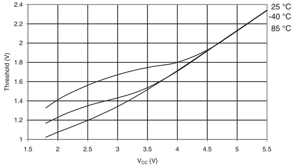
**Figure 30-282.** ATmega3290A: Reset Input Threshold Voltage vs.  $V_{CC}$  ( $V_{IL}$ , Reset Pin Read as "0")
