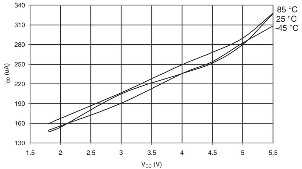
**Figure 30-541.** ATmega6490A: AREF External Reference Current vs.  $V_{CC}$
