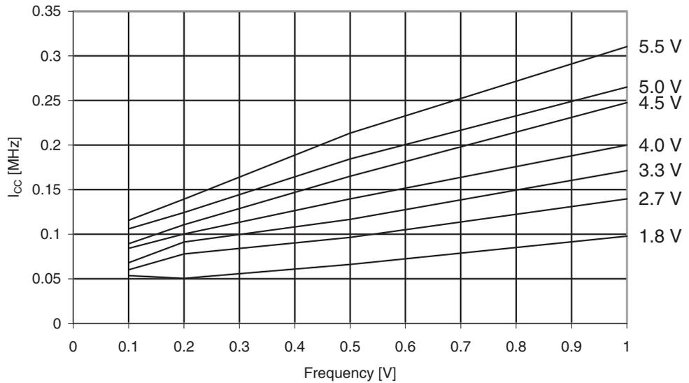
**Figure 30-251.** ATmega3290A: Idle Supply Current vs. Frequency (1 - 20MHz)
