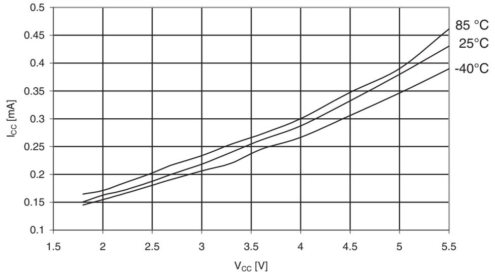
**Figure 30-254.** ATmega3290A: Idle Supply Current vs.  $V_{CC}$  (32kHz Watch Crystal)
