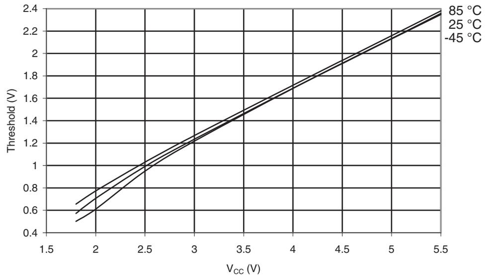
**Figure 30-584.** ATmega6490P: I/O Pin Input Hysteresis vs.  $V_{CC}$
