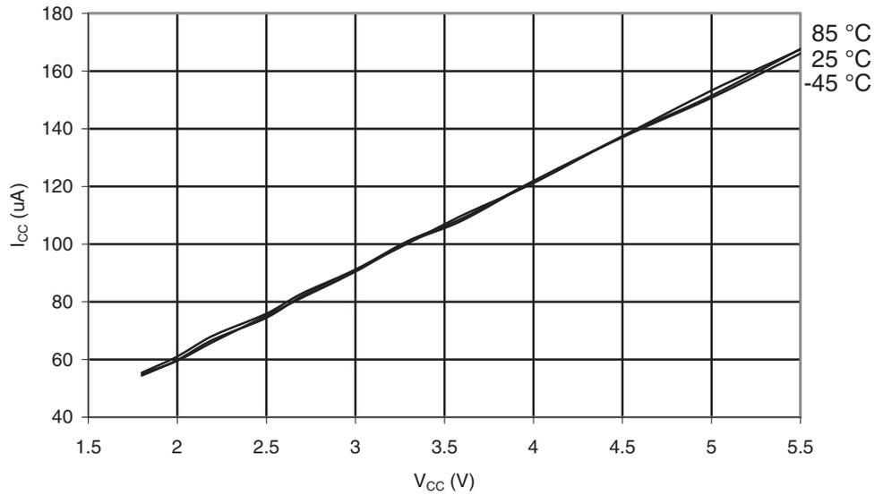
**Figure 30-119.** ATmega169PA: Watchdog Timer Current vs.  $V_{CC}$
