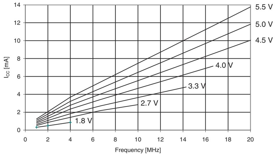
Figure 30-307. ATmega3290PA: Active Supply Current vs.  $V_{CC}$  (Internal RC Oscillator, 8MHz)
