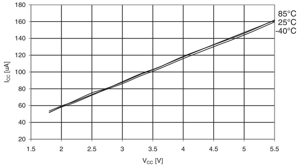
Figure 30-359. ATmega3290PA: Watchdog Timer Current vs.  $V_{CC}$
