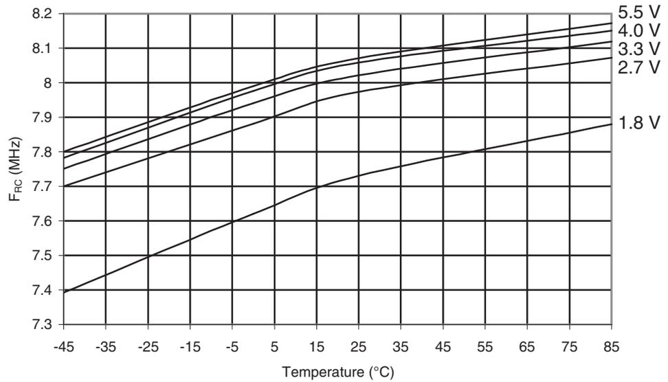
**Figure 30-535.** ATmega6490A: Calibrated 8MHz RC Oscillator Frequency vs.  $V_{CC}$
