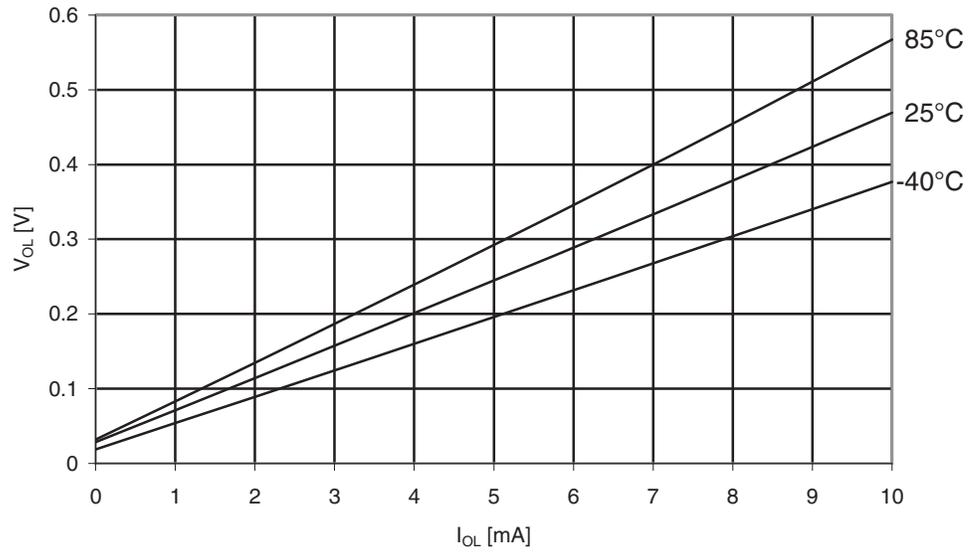
**Figure 30-153.** ATmega329A: I/O Pin Output Voltage vs. Sink Current, Ports A, C, D, E, F, G
