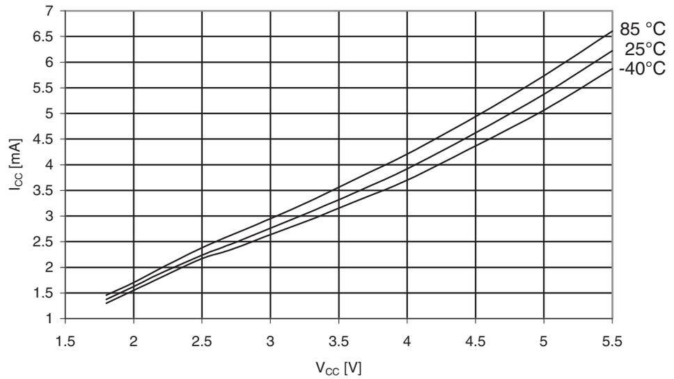
**Figure 30-188.** ATmega329PA: Active Supply Current vs.  $V_{CC}$  (Internal RC Oscillator, 1MHz)
