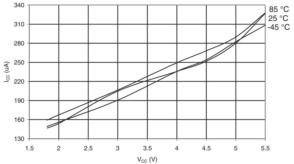
**Figure 30-480.** ATmega649P: AREF External Reference Current vs.  $V_{CC}$
