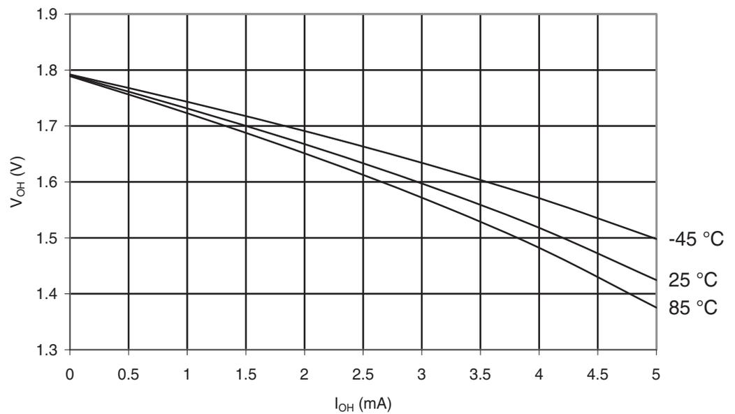
**Figure 30-28.** ATmega169A: I/O Pin Output Voltage vs. Sink Current, Ports A, C, D, E, F, G
