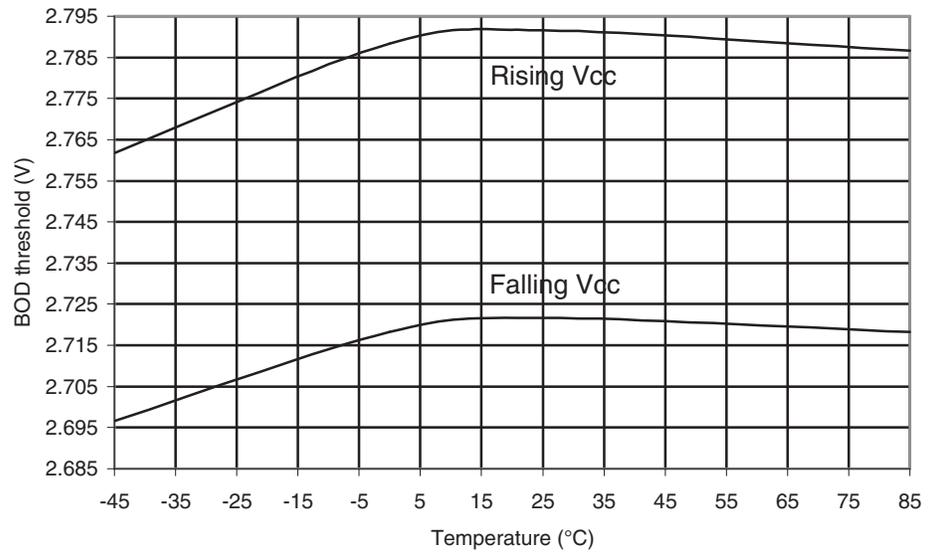
**Figure 30-407.** ATmega649A: BOD Thresholds vs. Temperature (BOD Level is 1.8V)
