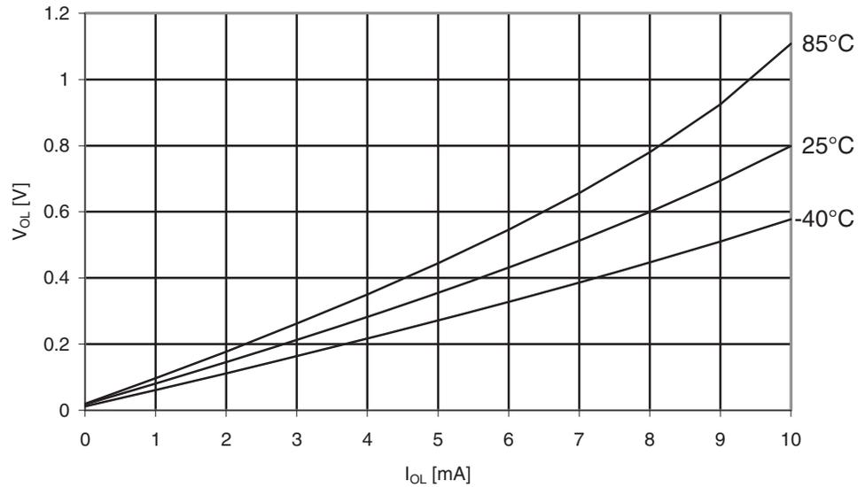
**Figure 30-214.** ATmega329PA: I/O Pin Output Voltage vs. Sink Current, Ports A, C, D, E, F, G ( $V_{CC} = 1.8V$ )
