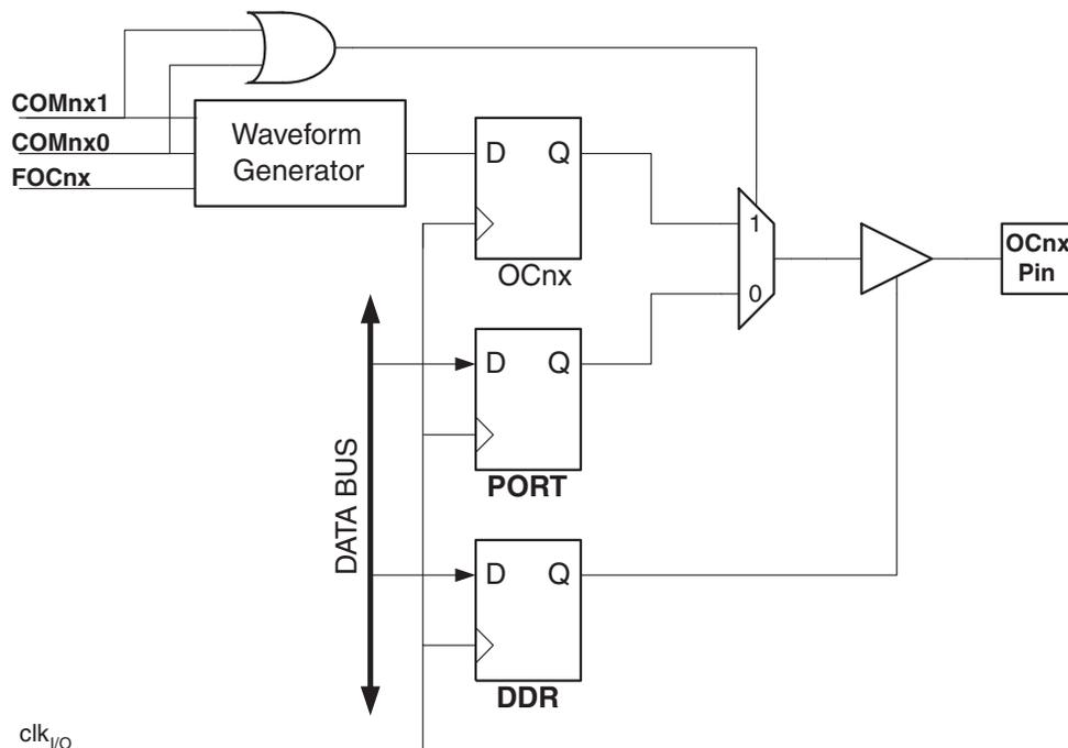
The general I/O port function is overridden by the Output Compare (OC2A) from the Waveform Generator if either of the COM2A[1:0] bits are set. However, the OC2A pin direction (input or output) is still controlled by the Data Direction Register (DDR) for the port pin. The Data Direc-
