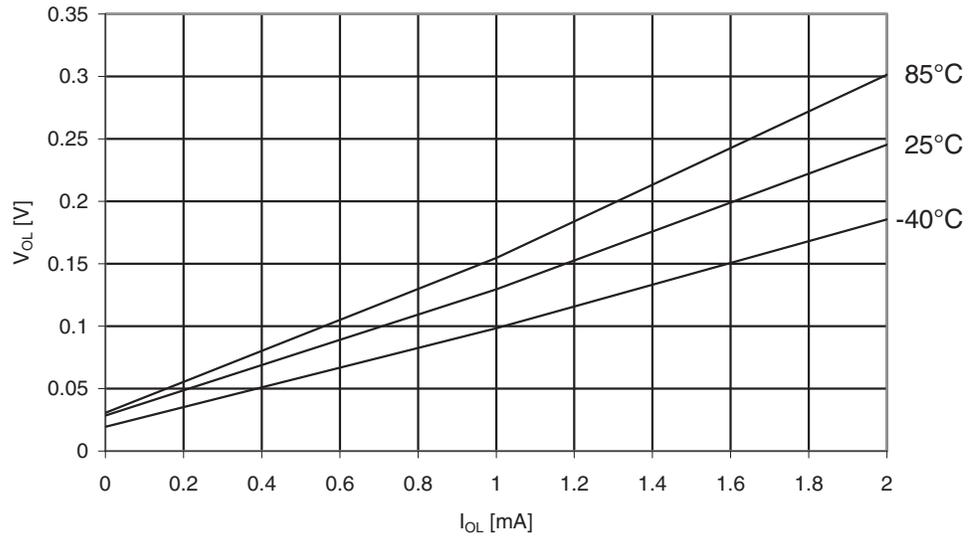
**Figure 30-155.** ATmega329A: I/O Pin Output Voltage vs. Sink Current, Port B ( $V_{CC} = 5V$ )
