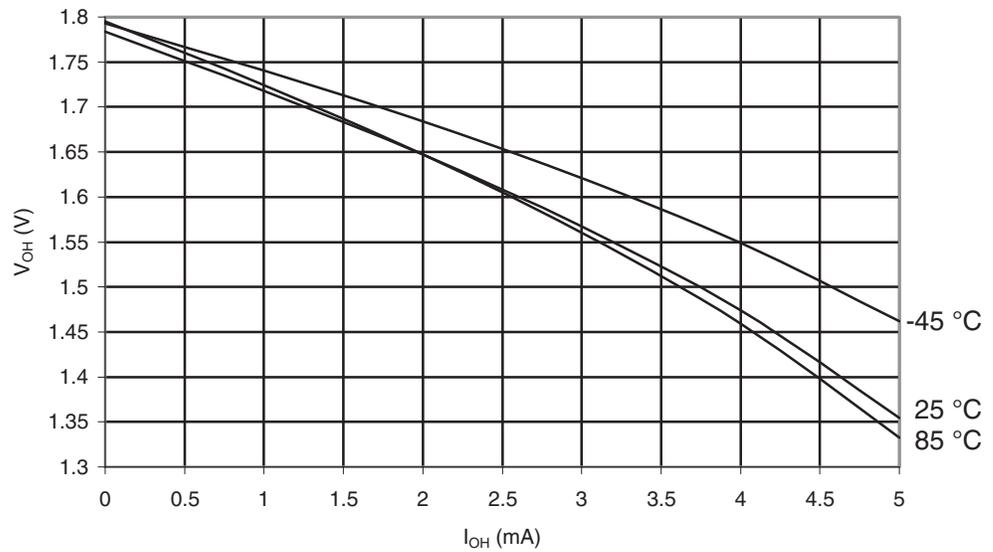
**Figure 30-515.** ATmega6490A: I/O Pin Output Voltage vs. Sink Current, Ports A, C, D, E, F, G ( $V_{CC} = 5V$ )
