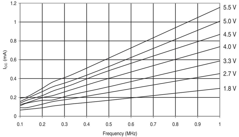
**Figure 30-549.** ATmega6490P: Active Supply Current vs. Frequency (1 - 20MHz)
