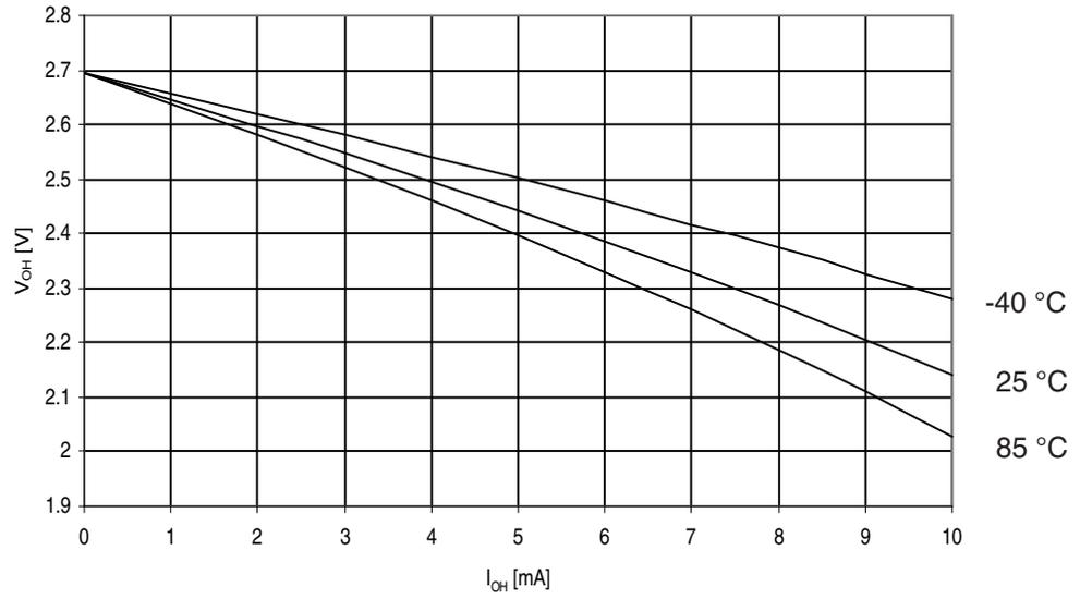
**Figure 30-268.** ATmega3290A: I/O Pin Output Voltage vs. Source Current, Ports A, C, D, E, F, G
