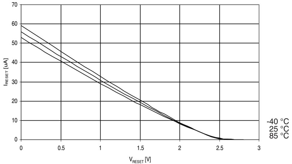
**Figure 30-265.** ATmega3290A: Reset Pull-up Resistor Current vs. Reset Pin Voltage ( $V_{CC}=1.8V$ )
