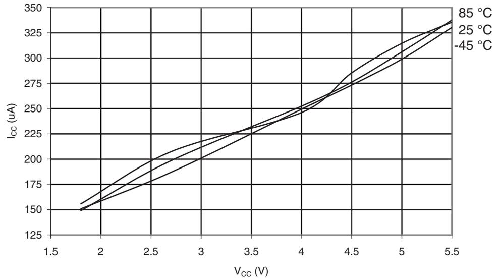
Figure 30-56. ATmega169A: AREF External Reference Current vs.  $V_{CC}$
