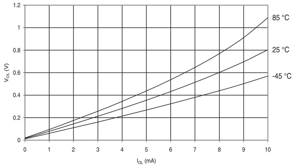
**Figure 30-578.** ATmega6490P: I/O Pin Output Voltage vs. Sink Current, Ports A, C, D, E, F, G ( $V_{CC} = 1.8V$ )
