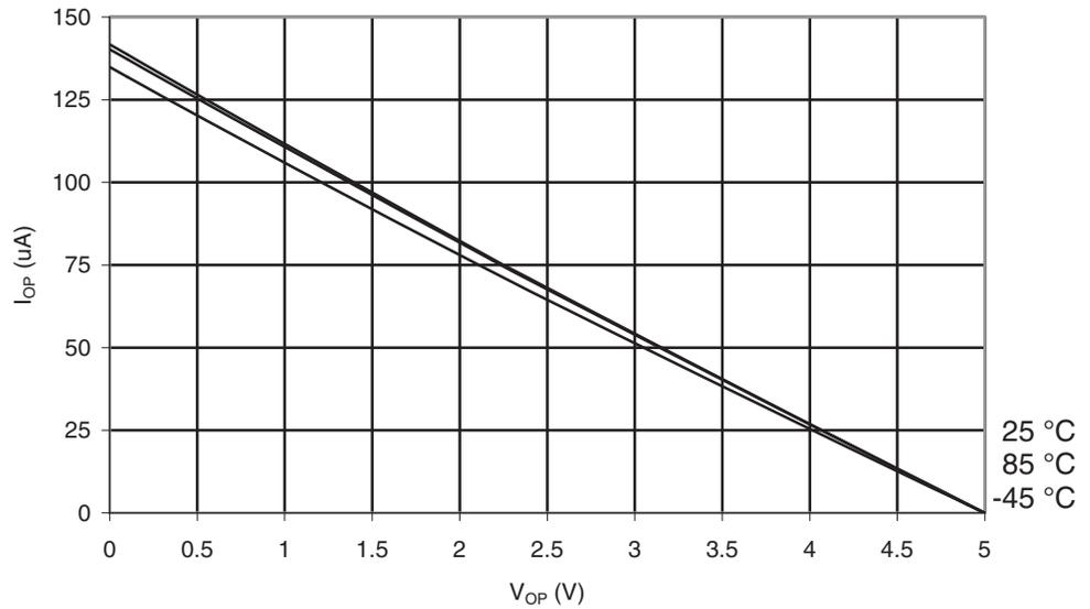
**Figure 30-79.** ATmega169PA: I/O Pin Pull-up Resistor Current vs. Input Voltage ( $V_{CC} = 2.7V$ )
