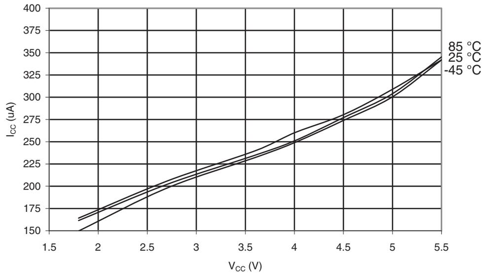
**Figure 30-116.** ATmega169PA: Active Supply Current with ADC at 200kHz vs.  $V_{CC}$
