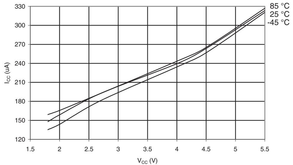
**Figure 30-478.** ATmega649P: Active Supply Current with ADC at 200kHz vs.  $V_{CC}$
