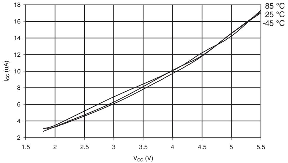
**Figure 30-604.** ATmega6490P: Analog Comparator Current vs.  $V_{CC}$
