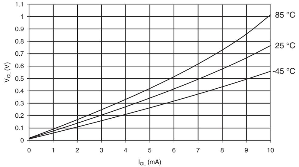
**Figure 30-29.** ATmega169A: I/O Pin Output Voltage vs. Sink Current, Ports A, C, D, E, F, G
