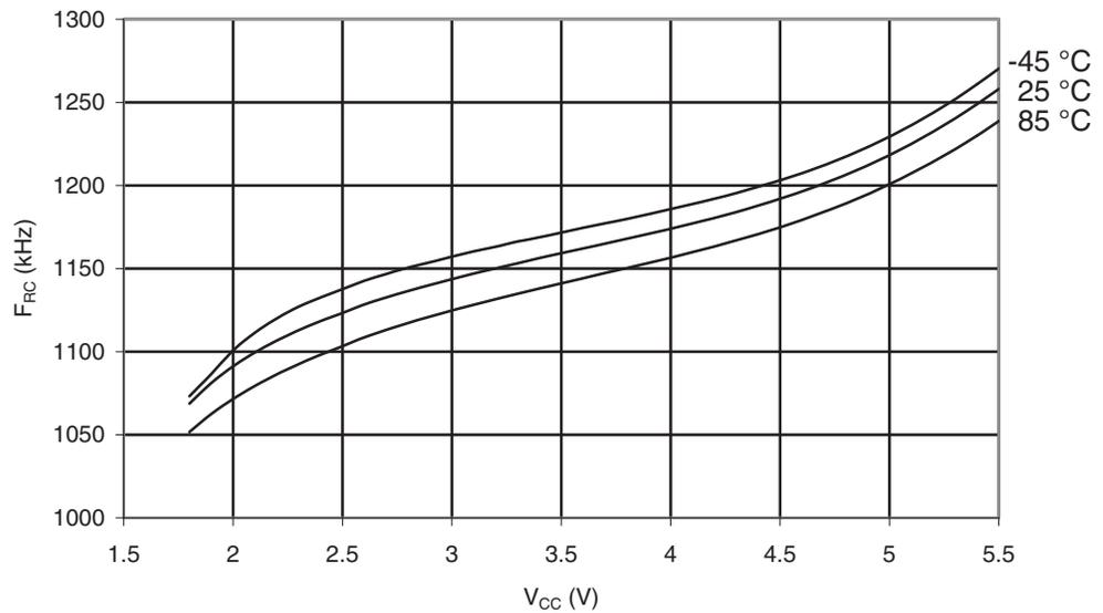
**Figure 30-48.** ATmega169A: Watchdog Oscillator Frequency vs. Temperature
