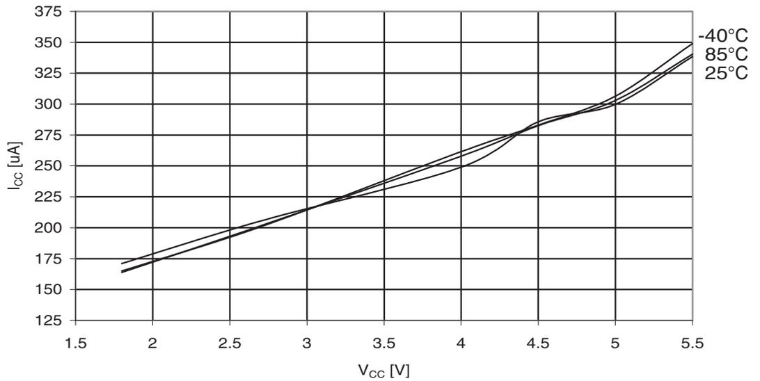
Figure 30-358. ATmega3290PA: AREF External Reference Current vs.  $V_{CC}$
