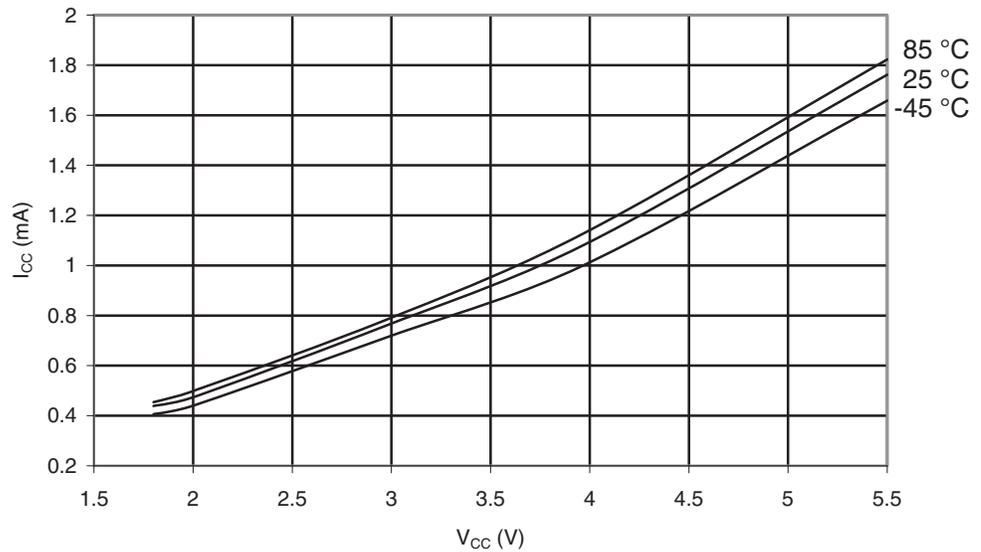
**Figure 30-373.** ATmega649A: Idle Supply Current vs.  $V_{CC}$  (Internal RC Oscillator, 1MHz)
