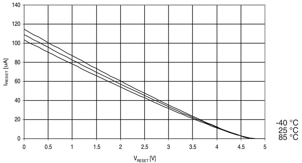
**Figure 30-324.** ATmega3290PA: Reset Pull-up Resistor Current vs. Reset Pin Voltage
