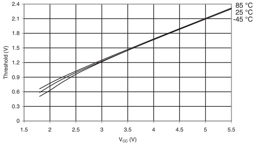
**Figure 30-98.** ATmega169PA: I/O Pin Input Hysteresis vs.  $V_{CC}$
