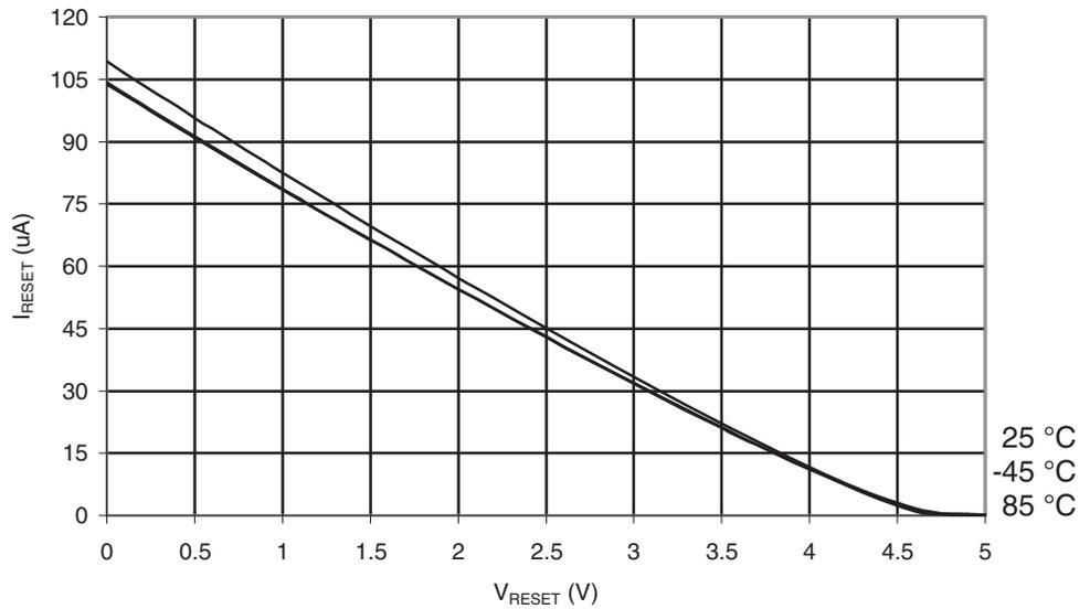
**Figure 30-385.** ATmega649A: Reset Pull-up Resistor Current vs. Reset Pin Voltage ( $V_{CC} = 2.7V$ )
