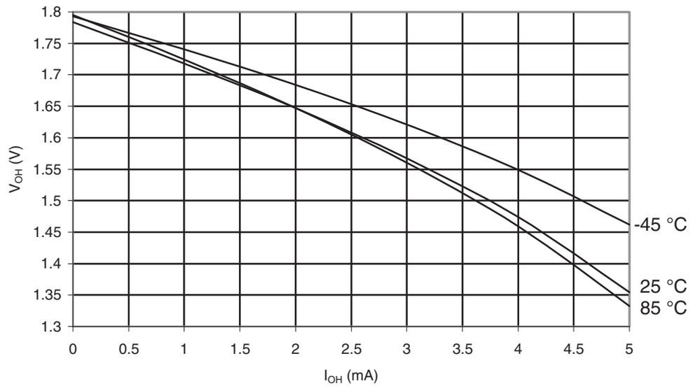
**Figure 30-454.** ATmega649P: I/O Pin Output Voltage vs. Sink Current, Ports A, C, D, E, F, G
