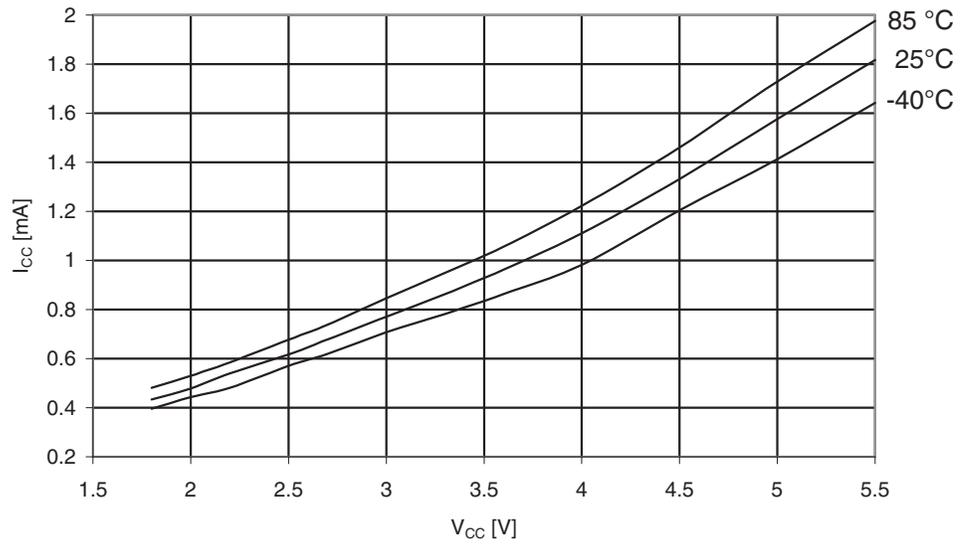
**Figure 30-193.** ATmega329PA: Idle Supply Current vs.  $V_{CC}$  (Internal RC Oscillator, 1MHz)
