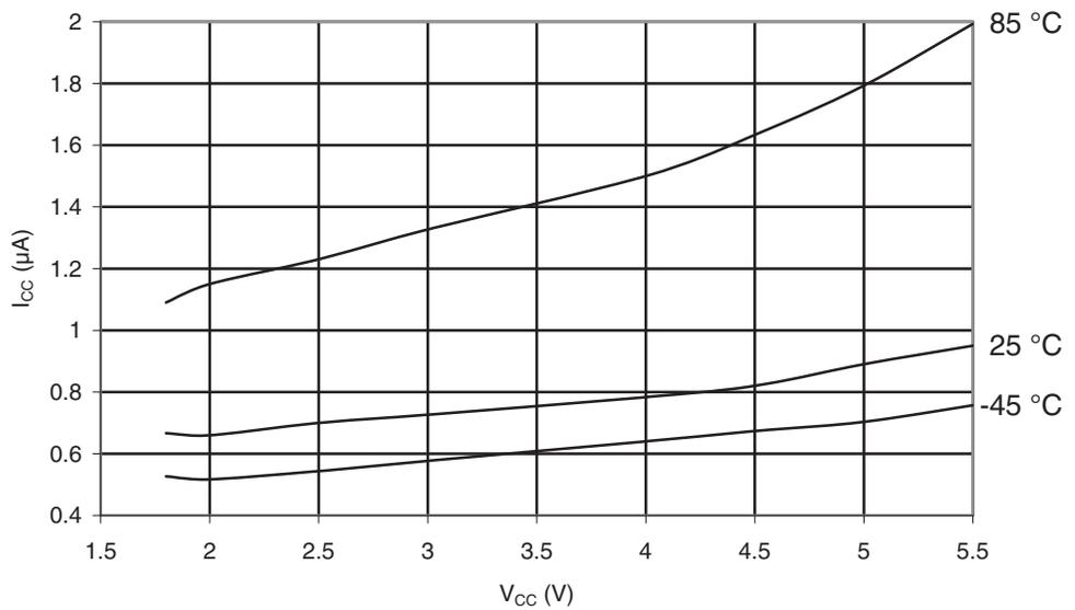
**Figure 30-77.** ATmega169PA: Standby Supply Current vs.  $V_{CC}$  (Xtall and Resonator, Watchdog Timer Disabled)
