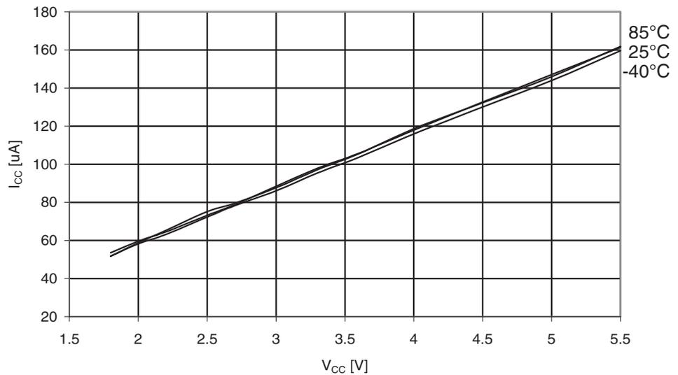
**Figure 30-299.** ATmega3290A: Watchdog Timer Current vs.  $V_{CC}$
