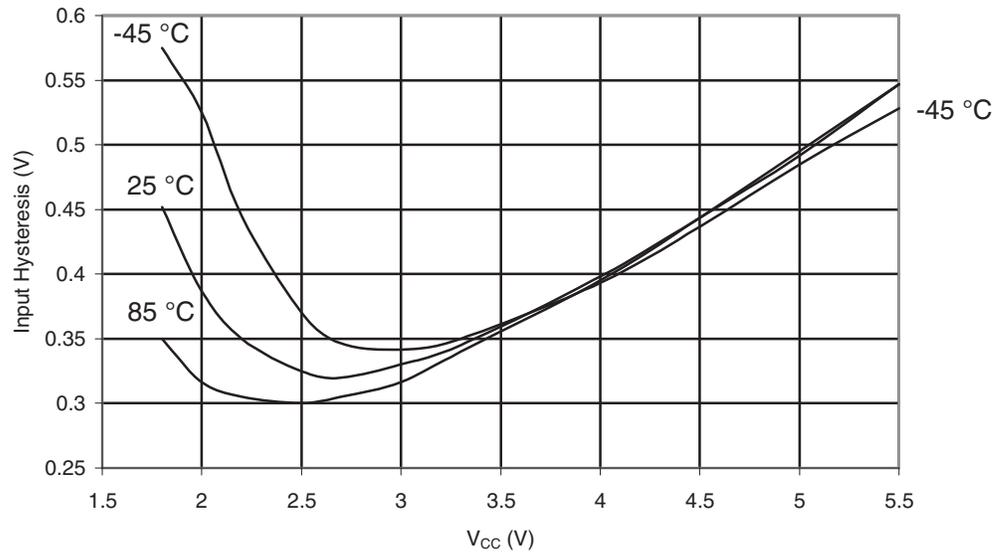
**Figure 30-402.** ATmega649A: Reset Input Threshold Voltage vs.  $V_{CC}$  ( $V_{IH}$ , Reset Pin Read as "1")
