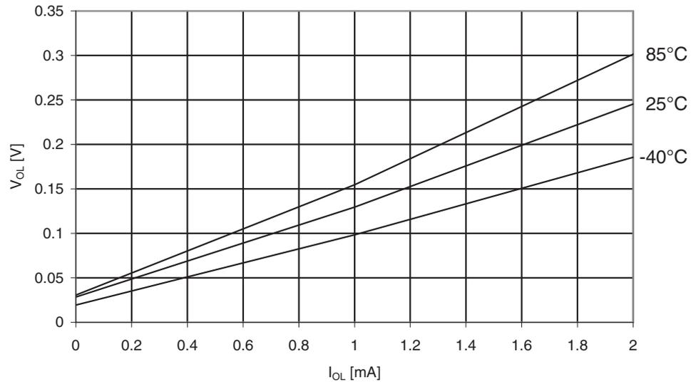
**Figure 30-215.** ATmega329PA: I/O Pin Output Voltage vs. Sink Current, Port B ( $V_{CC} = 5V$ )
