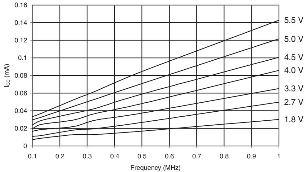
**Figure 30-424.** ATmega649A: Reset Supply Current vs.  $V_{CC}$  (1 - 20MHz, Excluding Current Through The Reset Pull-up)
