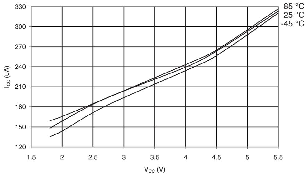
**Figure 30-600.** ATmega6490P: Active Supply Current with ADC at 200kHz vs.  $V_{CC}$
