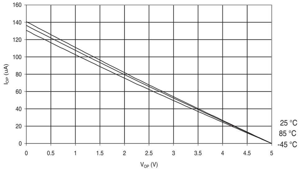
**Figure 30-382.** ATmega649A: I/O Pin Pull-up Resistor Current vs. Input Voltage ( $V_{CC} = 2.7V$ )
