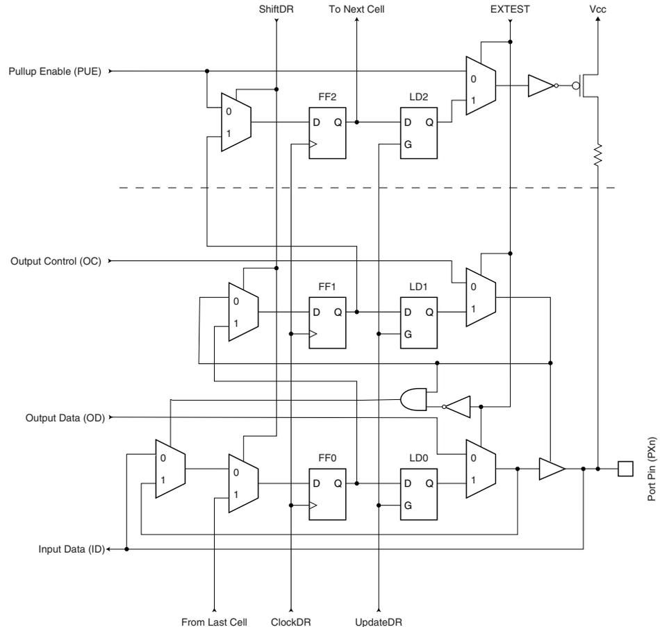
**Figure 26-3.** General Port Pin Schematic Diagram
