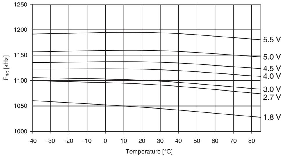
**Figure 30-171.** ATmega329A: Calibrated 8MHz RC Oscillator Frequency vs. Temperature
