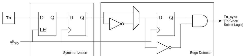
The synchronization and edge detector logic introduces a delay of 2.5 to 3.5 system clock cycles from an edge has been applied to the T1/T0 pin to the counter is updated.
