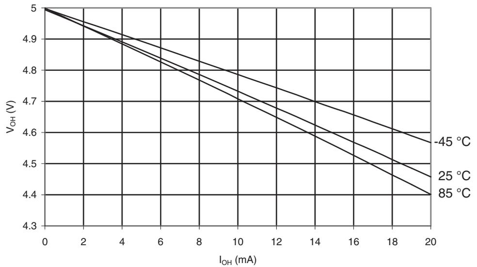
**Figure 30-574.** ATmega6490P: I/O Pin Output Voltage vs. Source Current, Port B ( $V_{CC} = 2.7V$ )
