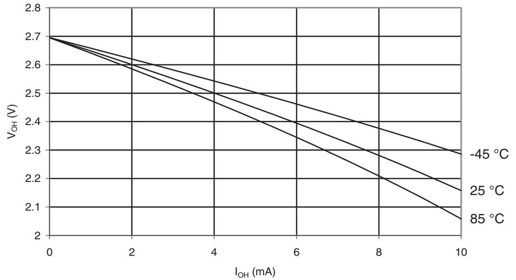
**Figure 30-86.** ATmega169PA: I/O Pin Output Voltage vs. Source Current, Ports A, C, D, E, F, G
