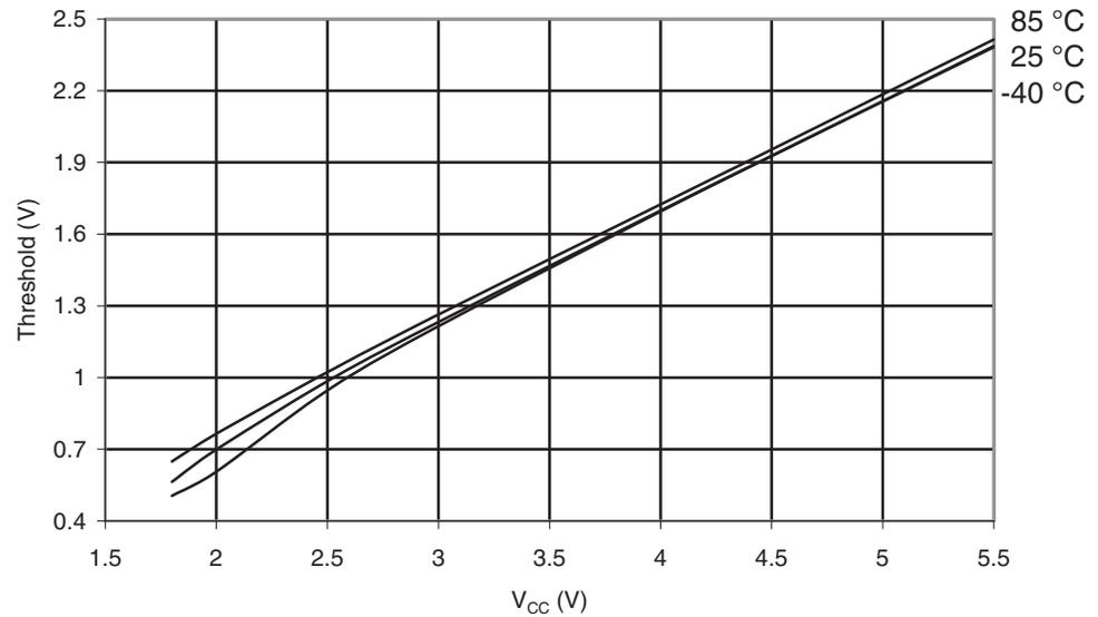
**Figure 30-340.** ATmega3290PA: I/O Pin Input Hysteresis vs.  $V_{CC}$
