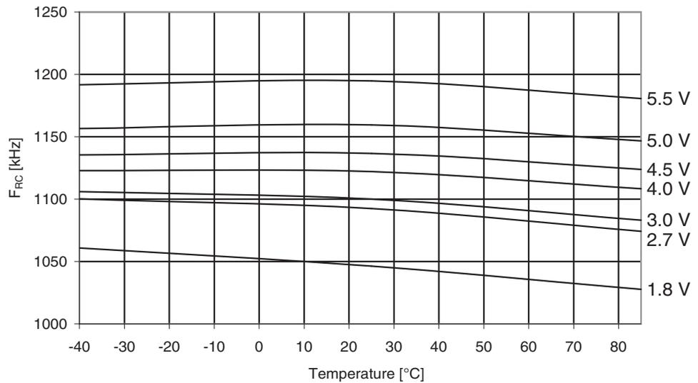
**Figure 30-291.** ATmega3290A: Calibrated 8MHz RC Oscillator Frequency vs. Temperature
