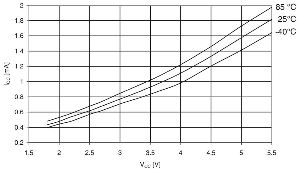
**Figure 30-133.** ATmega329A: Idle Supply Current vs.  $V_{CC}$  (Internal RC Oscillator, 1MHz)
