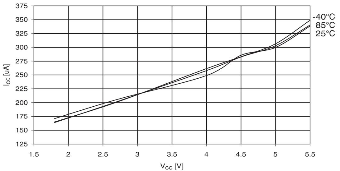
Figure 30-178. ATmega329A: AREF External Reference Current vs.  $V_{CC}$
