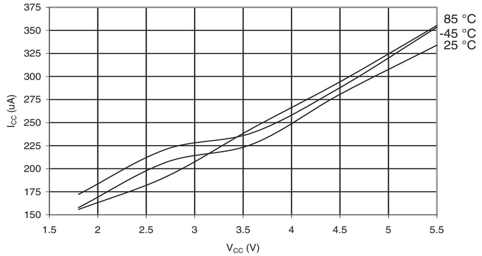
**Figure 30-55.** ATmega169A: Active Supply Current with ADC at 1MHz vs.  $V_{CC}$
