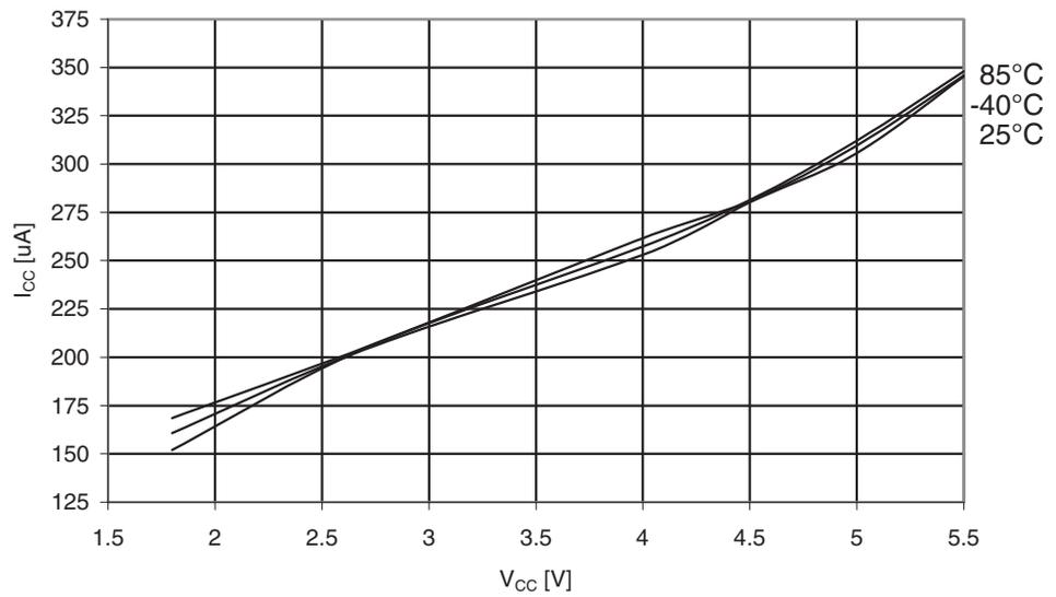
**Figure 30-177.** ATmega329A: Active Supply Current with ADC at 1MHz vs.  $V_{CC}$
