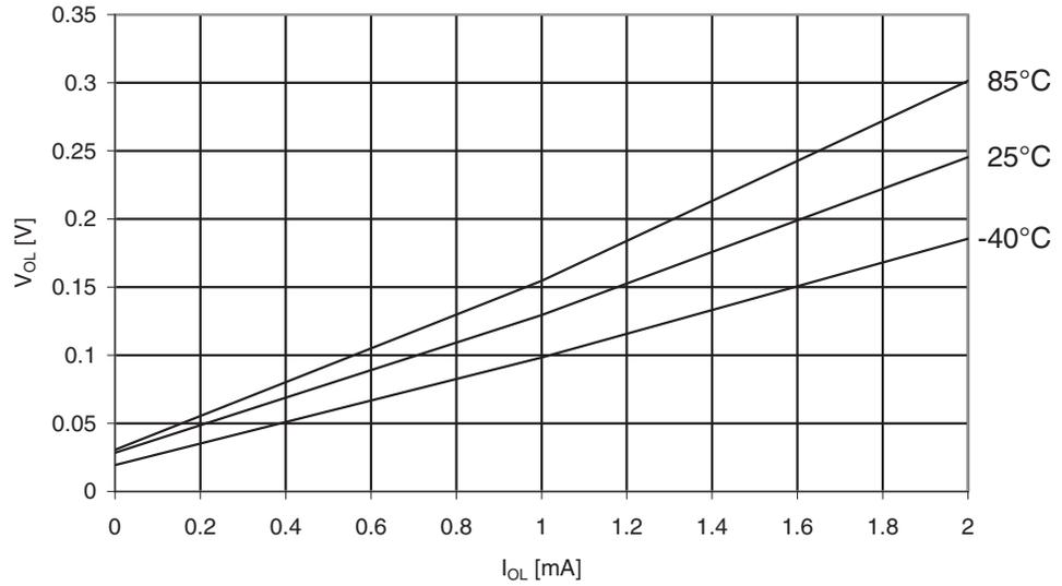
**Figure 30-335.** ATmega3290PA: I/O Pin Output Voltage vs. Sink Current, Port B ( $V_{CC} = 5V$ )
