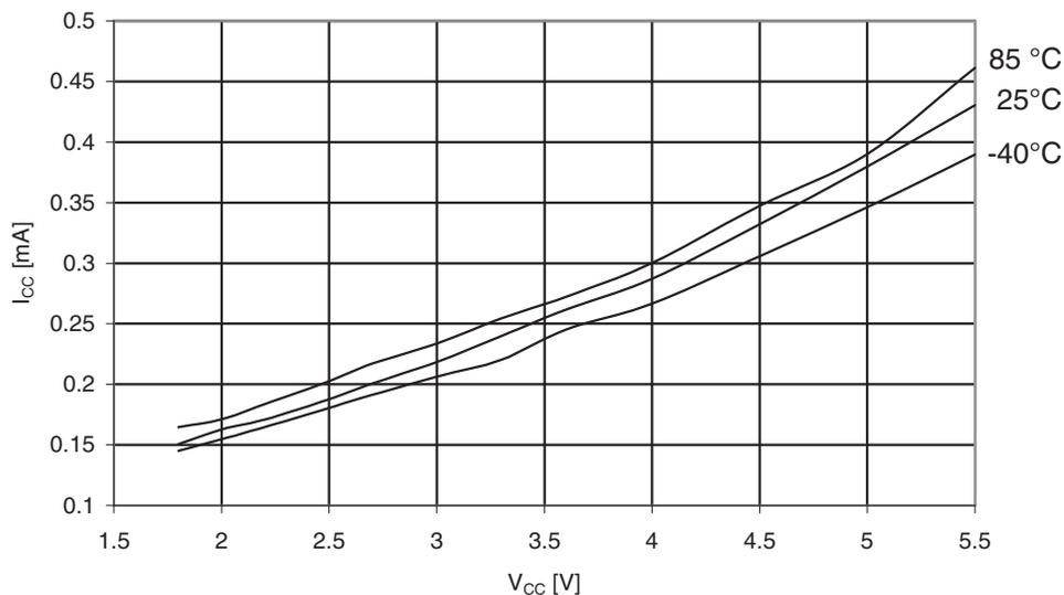
**Figure 30-314.** ATmega3290PA: Idle Supply Current vs.  $V_{CC}$  (32kHz Watch Crystal)
