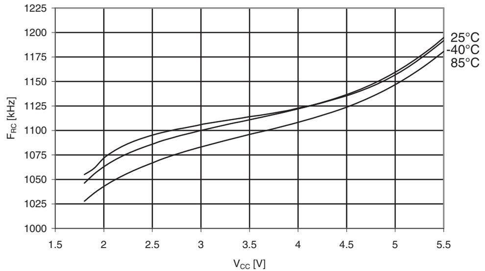
**Figure 30-170.** ATmega329A: Watchdog Oscillator Frequency vs. Temperature
