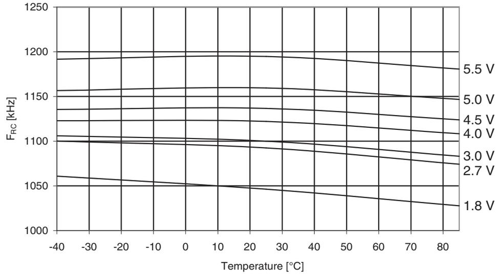
**Figure 30-231.** ATmega329PA: Calibrated 8MHz RC Oscillator Frequency vs. Temperature
