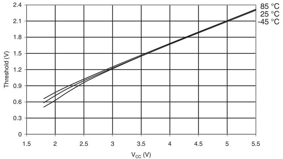
**Figure 30-36.** ATmega169A: I/O Pin Input Hysteresis vs.  $V_{CC}$
