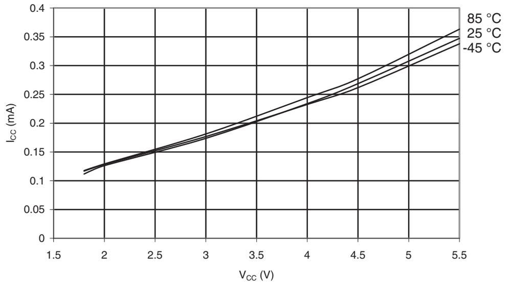
**Figure 30-10.** ATmega169A: Idle Supply Current vs.  $V_{CC}$  (32kHz Watch Crystal)
