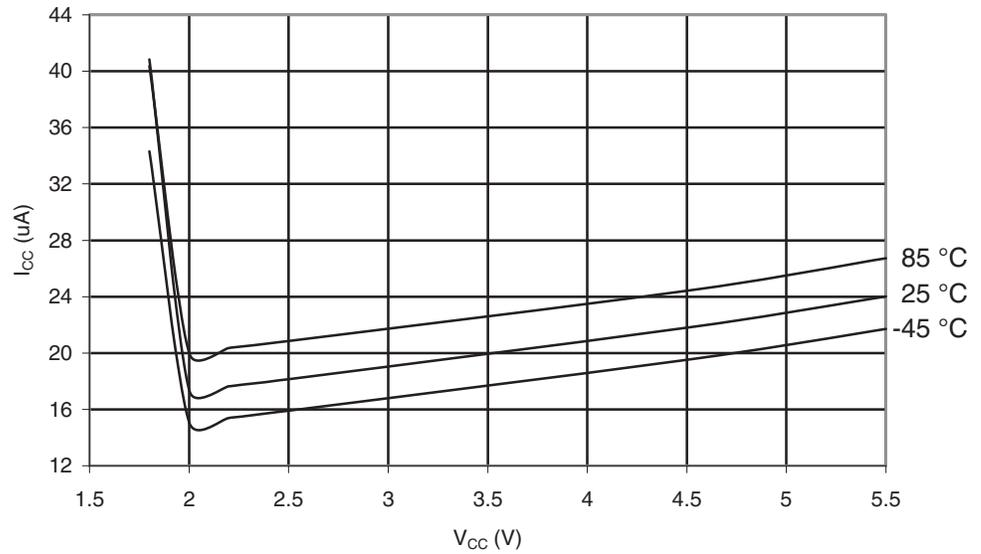
**Figure 30-53.** ATmega169A: Active Supply Current with ADC at 50kHz vs.  $V_{CC}$
