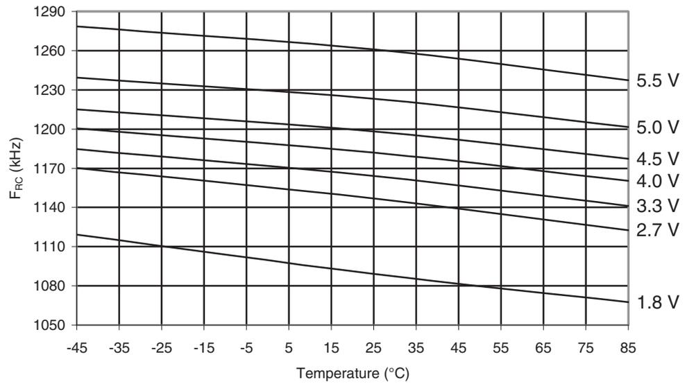
**Figure 30-412.** ATmega649A: Calibrated 8MHz RC Oscillator Frequency vs. Temperature
