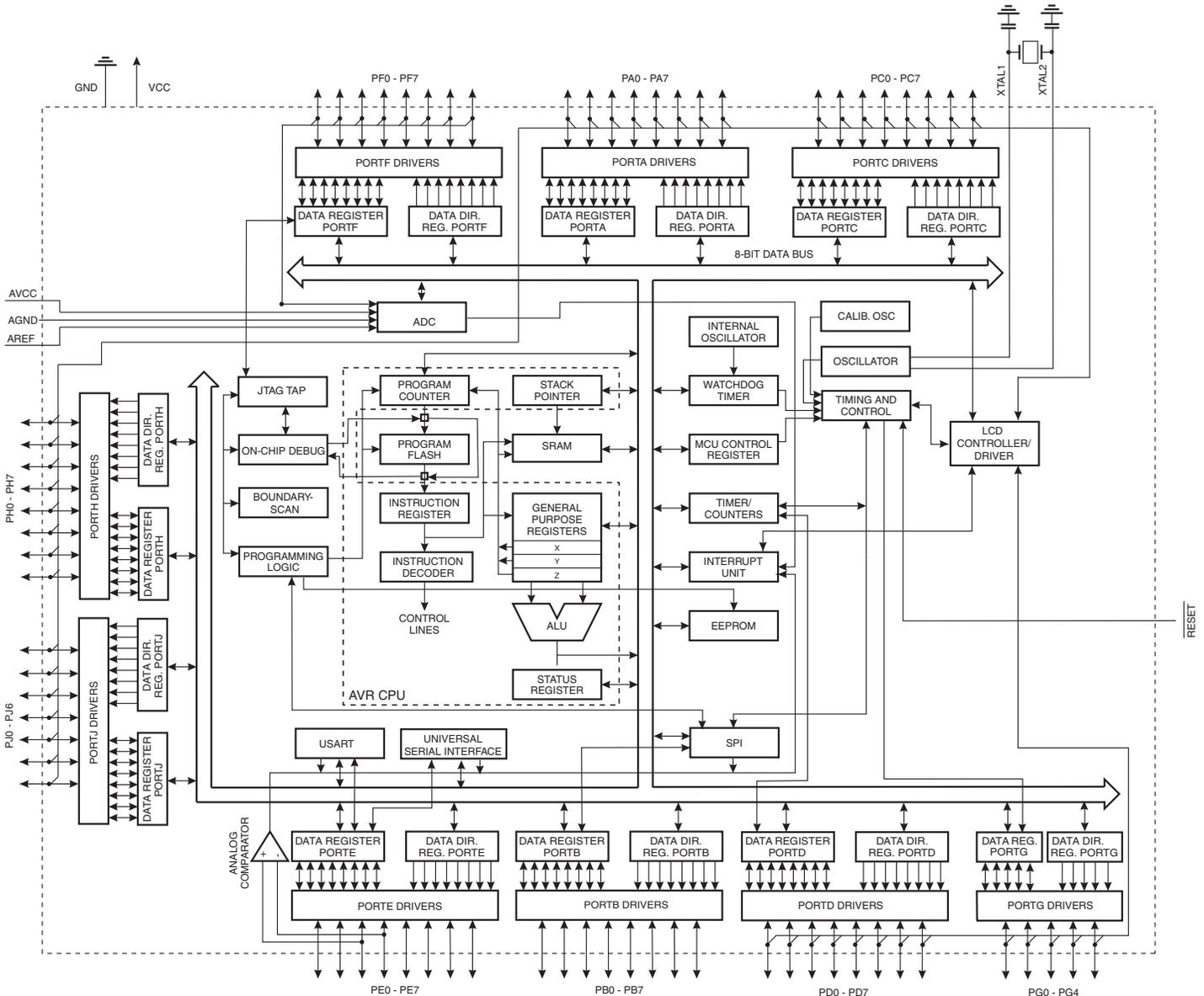
The AVR core combines a rich instruction set with 32 general purpose working registers. All the 32 registers are directly connected to the Arithmetic Logic Unit (ALU), allowing two independent registers to be accessed in one single instruction executed in one clock cycle. The resulting
