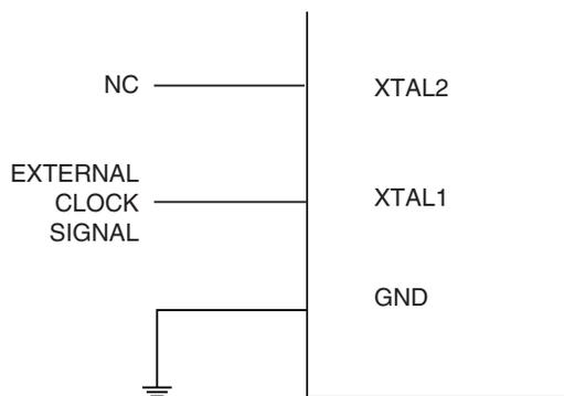
When this clock source is selected, start-up times are determined by the SUT Fuses as shown in [Table 9-13](#).
