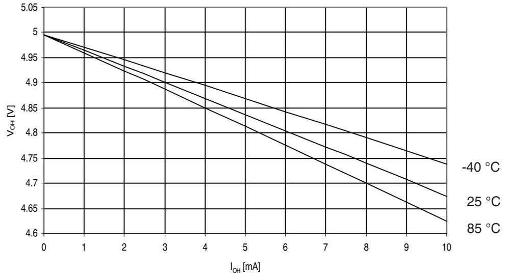
**Figure 30-147.** ATmega329A: I/O Pin Output Voltage vs. Source Current, Ports A, C, D, E, F, G
