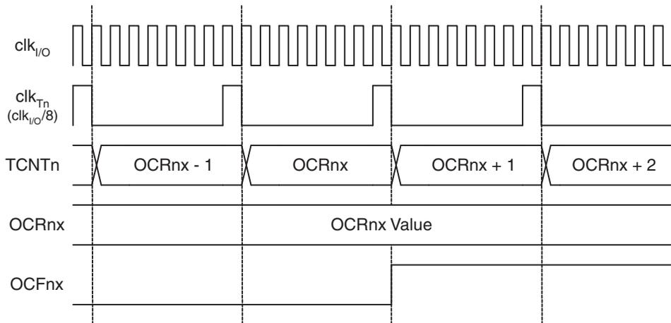
Figure 18-11 on page 158 shows the setting of OCF2A and the clearing of TCNT2 in CTC mode.
