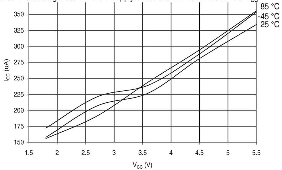
**Figure 30-117.** ATmega169PA: Active Supply Current with ADC at 1MHz vs.  $V_{CC}$
