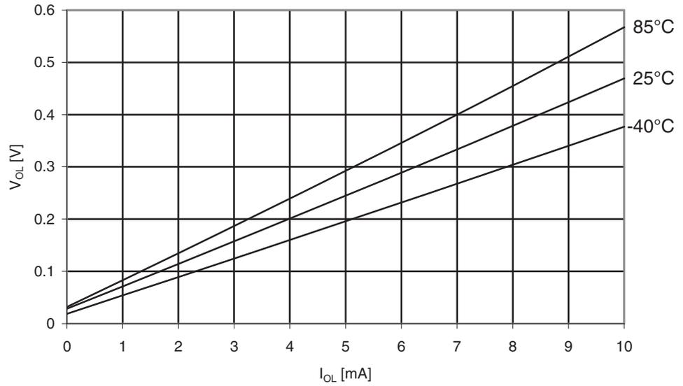
**Figure 30-213.** ATmega329PA: I/O Pin Output Voltage vs. Sink Current, Ports A, C, D, E, F, G
