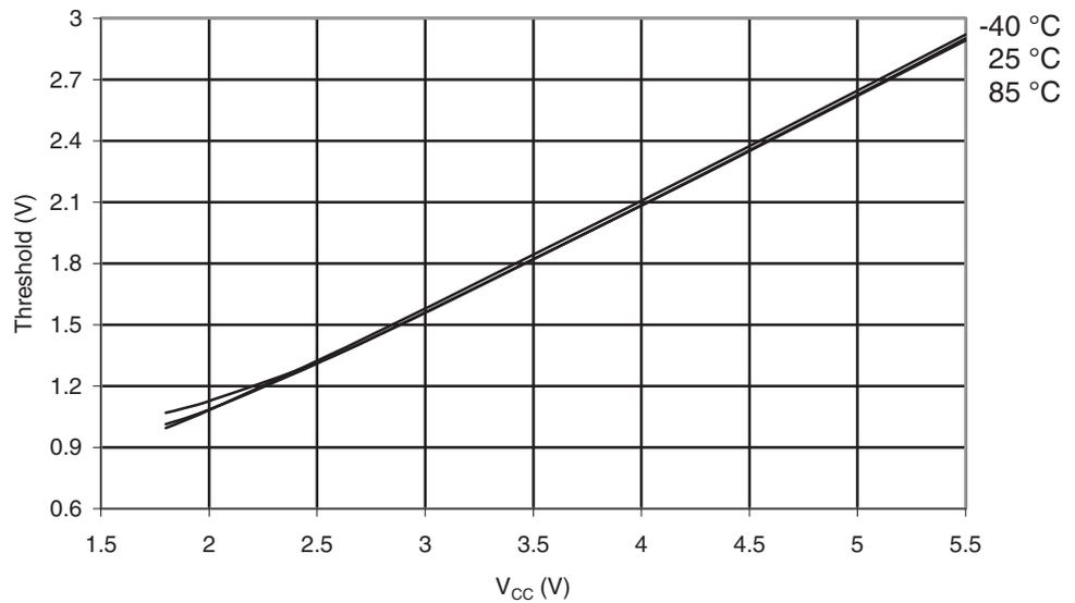
**Figure 30-279.** ATmega3290A: I/O Pin Input Threshold Voltage vs.  $V_{CC}$  ( $V_{IL}$ , I/O Pin Read as "0")
