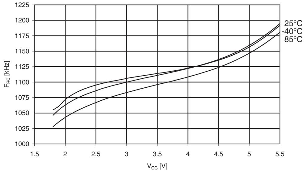
**Figure 30-350.** ATmega3290PA: Watchdog Oscillator Frequency vs. Temperature
