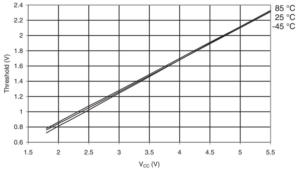
**Figure 30-101.** ATmega169PA: Reset Input Pin Hysteresis vs.  $V_{CC}$
