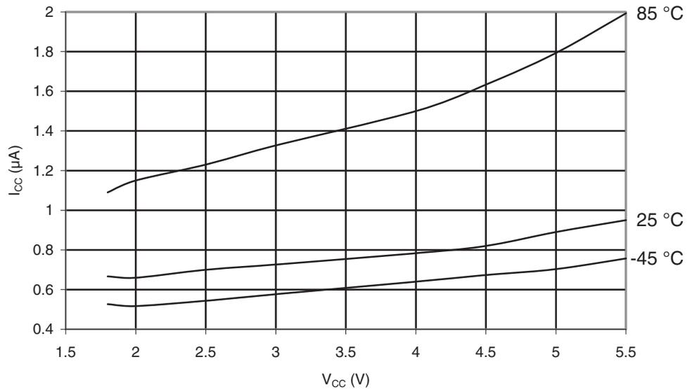
**Figure 30-15.** ATmega169A: Standby Supply Current vs.  $V_{CC}$  (Xtall and Resonator, Watchdog Timer Disabled)
