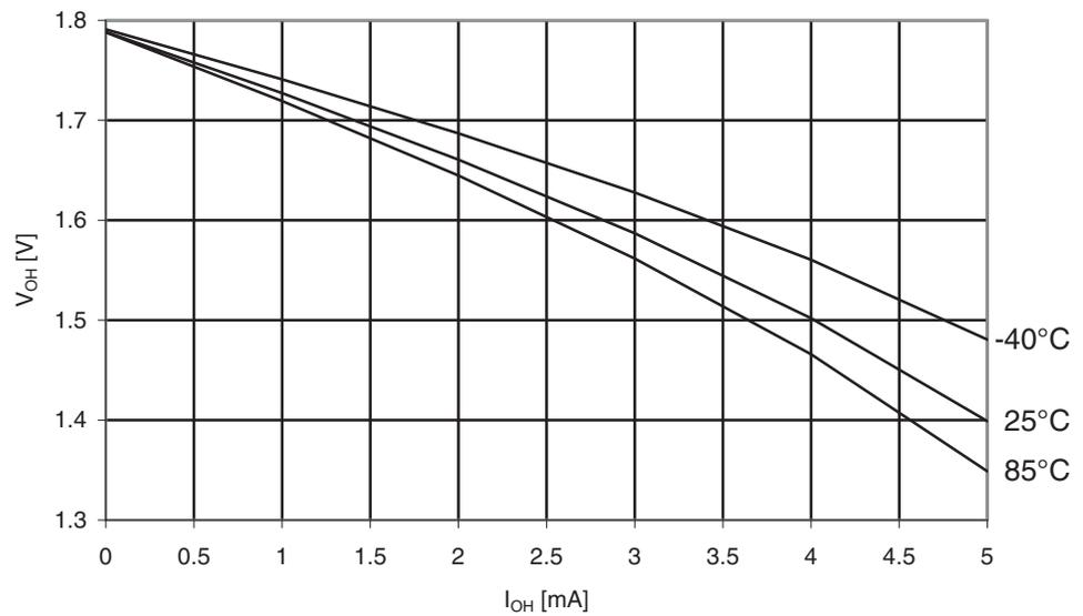
**Figure 30-212.** ATmega329PA: I/O Pin Output Voltage vs. Sink Current, Ports A, C, D, E, F, G
