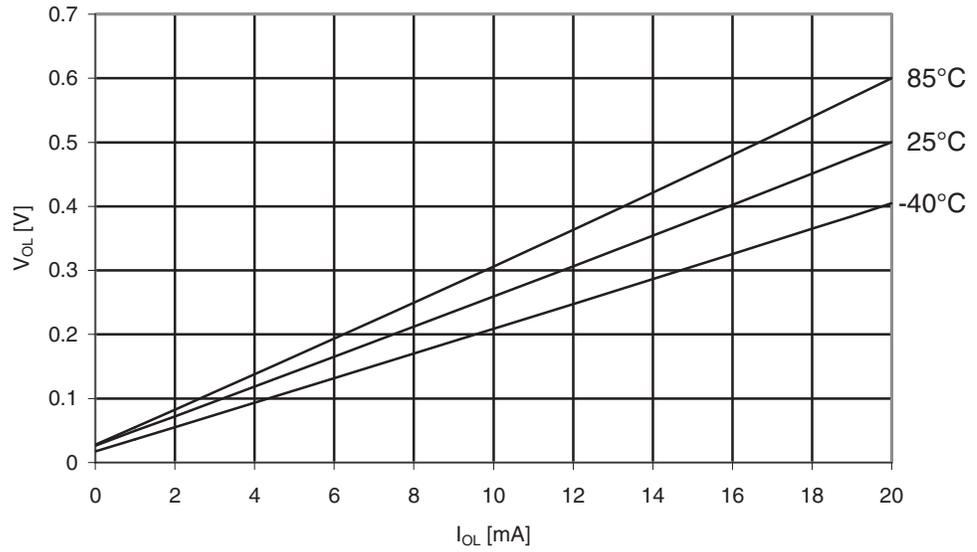
**Figure 30-336.** ATmega3290PA: I/O Pin Output Voltage vs. Sink Current, Port B ( $V_{CC} = 2.7V$ )
