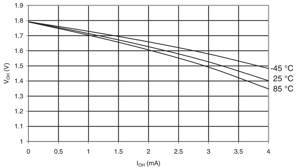
**Figure 30-87.** ATmega169PA: I/O Pin Output Voltage vs. Source Current, Port B ( $V_{CC} = 5V$ )
