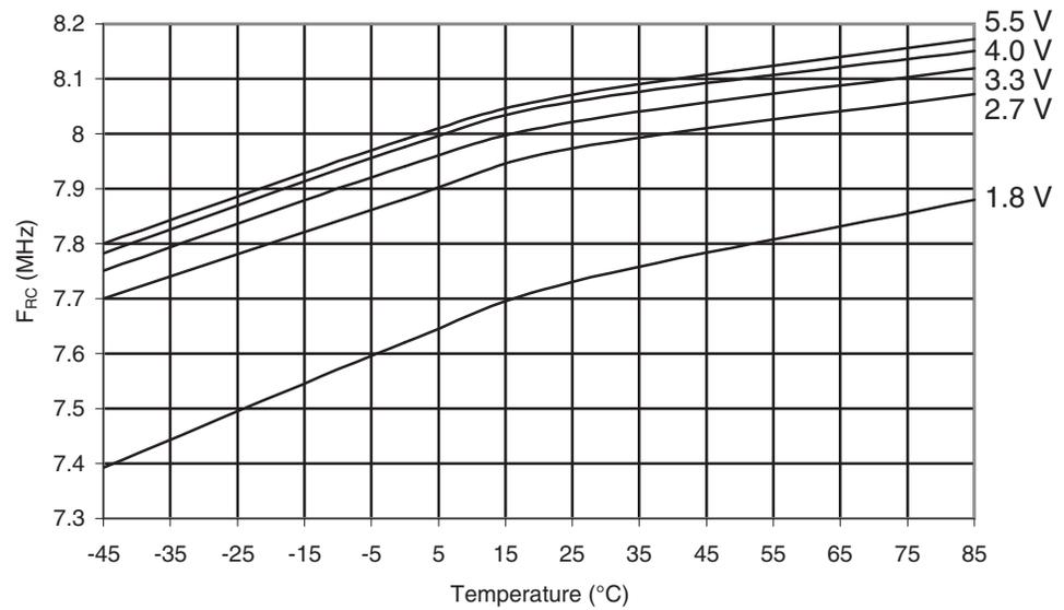
**Figure 30-413.** ATmega649A: Calibrated 8MHz RC Oscillator Frequency vs.  $V_{CC}$
