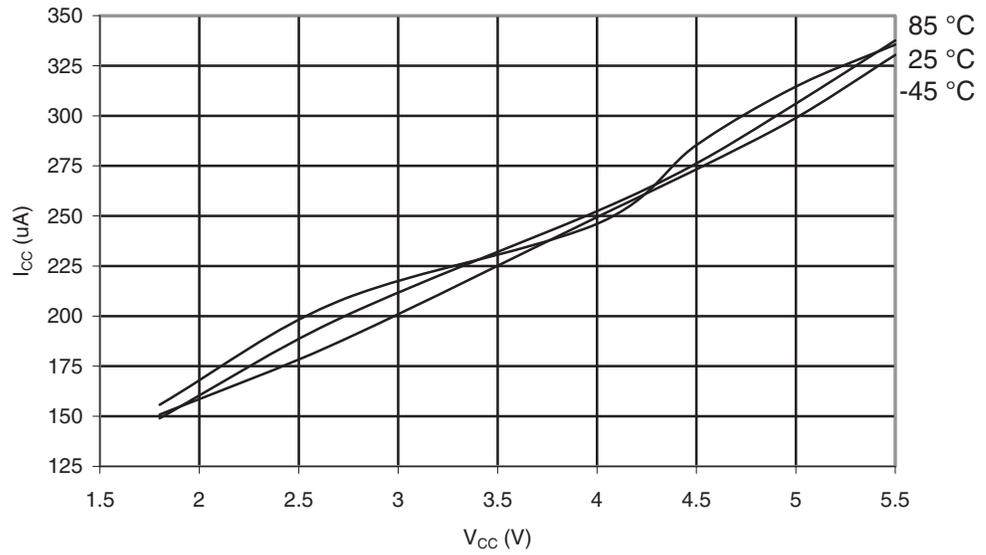
**Figure 30-118.** ATmega169PA: AREF External Reference Current vs.  $V_{CC}$
