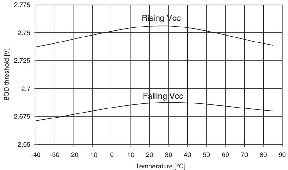
**Figure 30-226.** ATmega329PA: BOD Thresholds vs. Temperature (BOD Level is 1.8V)
