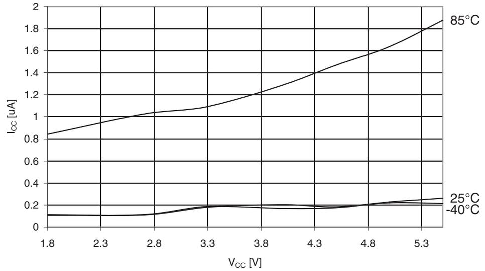
**Figure 30-316.** ATmega3290PA: Power-down Supply Current vs.  $V_{CC}$  (Watchdog Timer Enabled)
