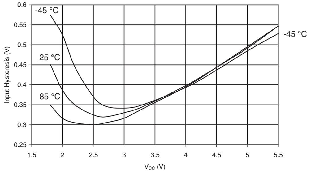
**Figure 30-463.** ATmega649P: Reset Input Threshold Voltage vs.  $V_{CC}$  ( $V_{IH}$ , Reset Pin Read as "1")
