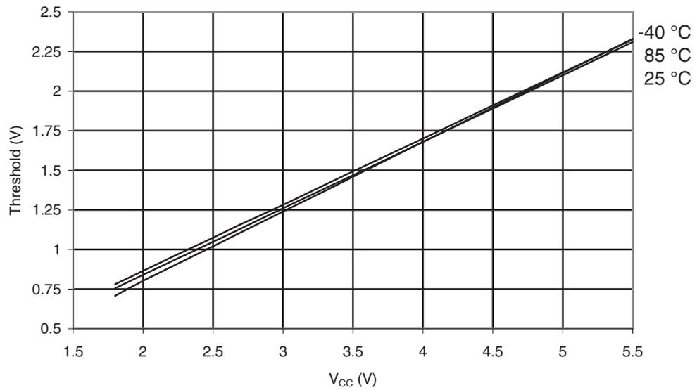
**Figure 30-283.** ATmega3290A: Reset Input Pin Hysteresis vs.  $V_{CC}$
