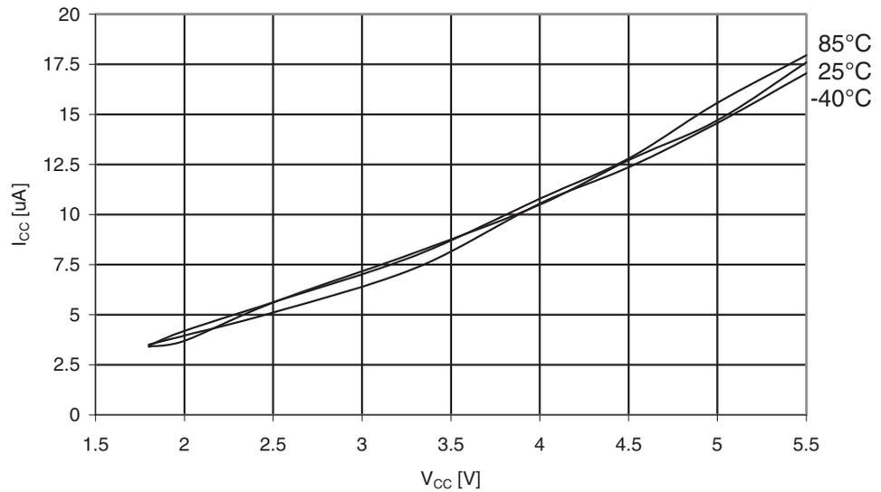
Figure 30-360. ATmega3290PA: Analog Comparator Current vs.  $V_{CC}$
