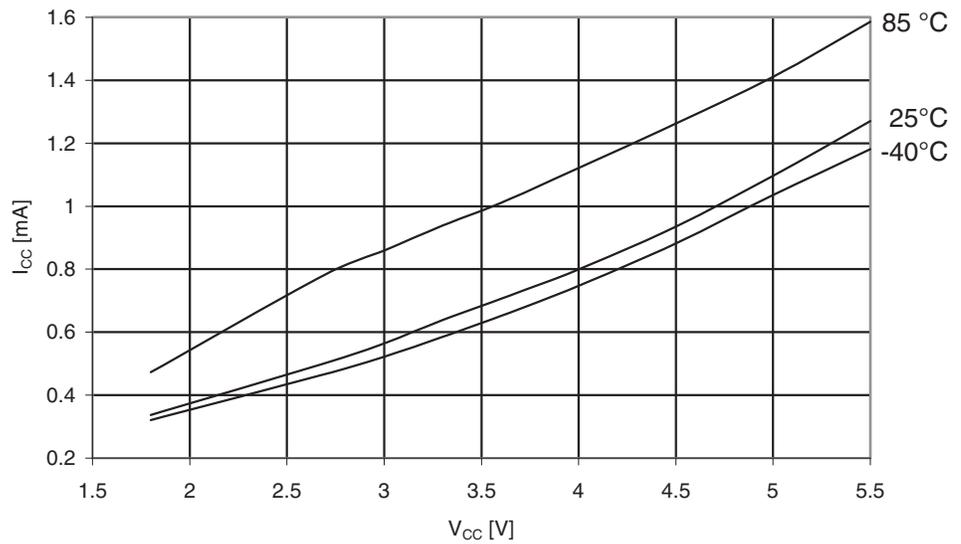
**Figure 30-309.** ATmega3290PA: Active Supply Current vs.  $V_{CC}$  (32kHz Watch Crystal)
