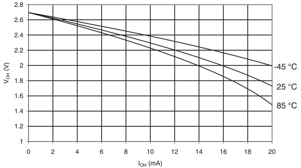
**Figure 30-27.** ATmega169A: I/O Pin Output Voltage vs. Source Current, Port B ( $V_{CC} = 1.8V$ )
