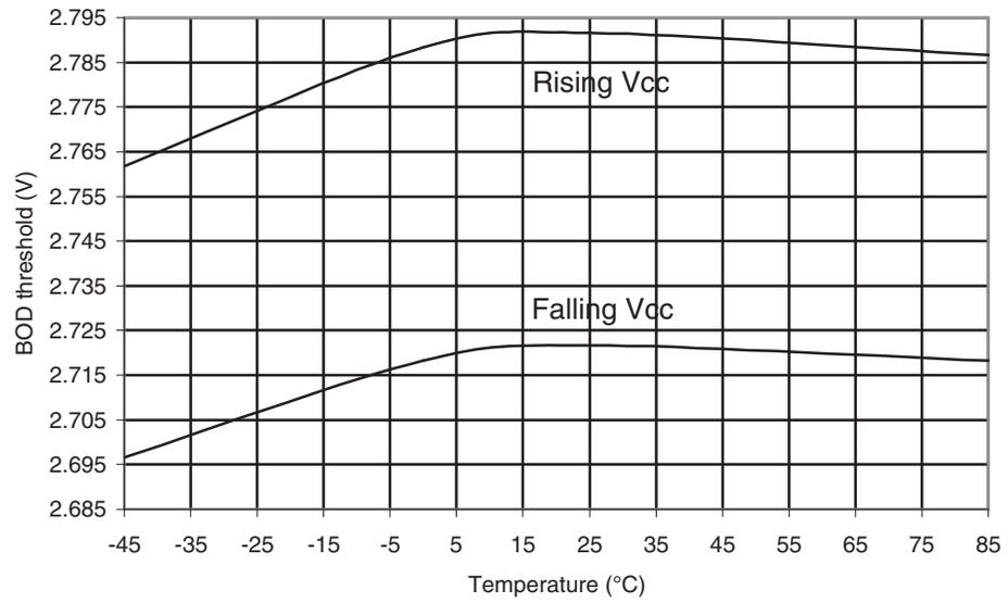
**Figure 30-529.** ATmega6490A: BOD Thresholds vs. Temperature (BOD Level is 1.8V)
