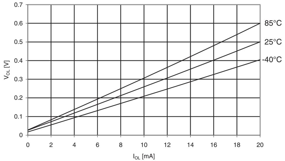
**Figure 30-276.** ATmega3290A: I/O Pin Output Voltage vs. Sink Current, Port B ( $V_{CC} = 2.7V$ )
