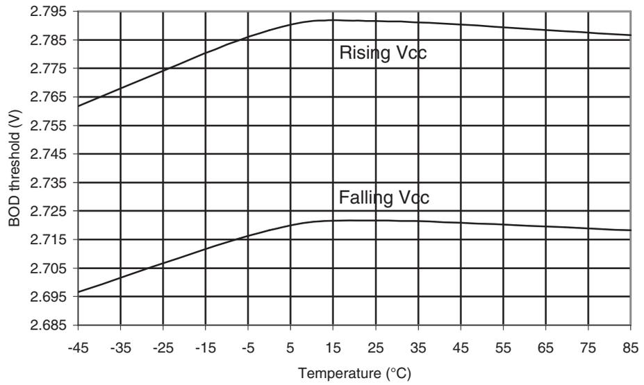
**Figure 30-468.** ATmega649P: BOD Thresholds vs. Temperature (BOD Level is 1.8V)
