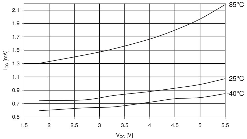
**Figure 30-199.** ATmega329PA Standby Supply Current vs.  $V_{CC}$  (Xtall and Resonator, Watchdog Timer Disabled)
