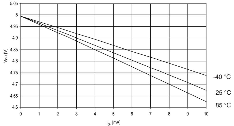
**Figure 30-267.** ATmega3290A: I/O Pin Output Voltage vs. Source Current, Ports A, C, D, E, F, G
