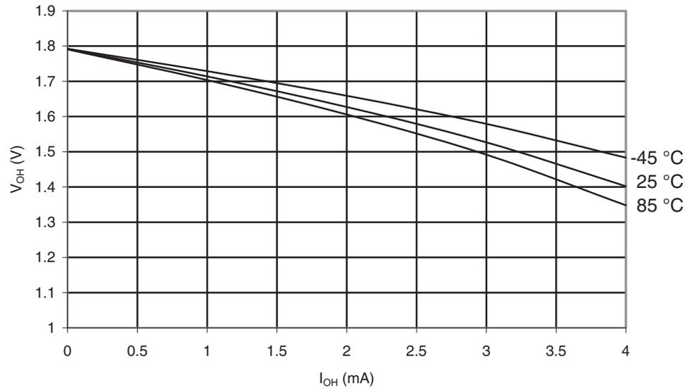
**Figure 30-25.** ATmega169A: I/O Pin Output Voltage vs. Source Current, Port B ( $V_{CC} = 5V$ )
