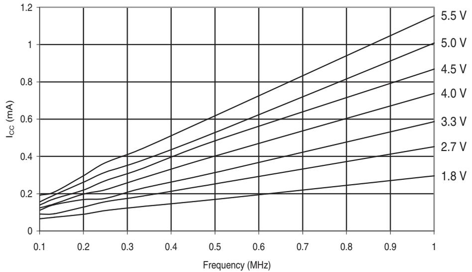
**Figure 30-366.** ATmega649A: Active Supply Current vs. Frequency (1 - 20MHz)
