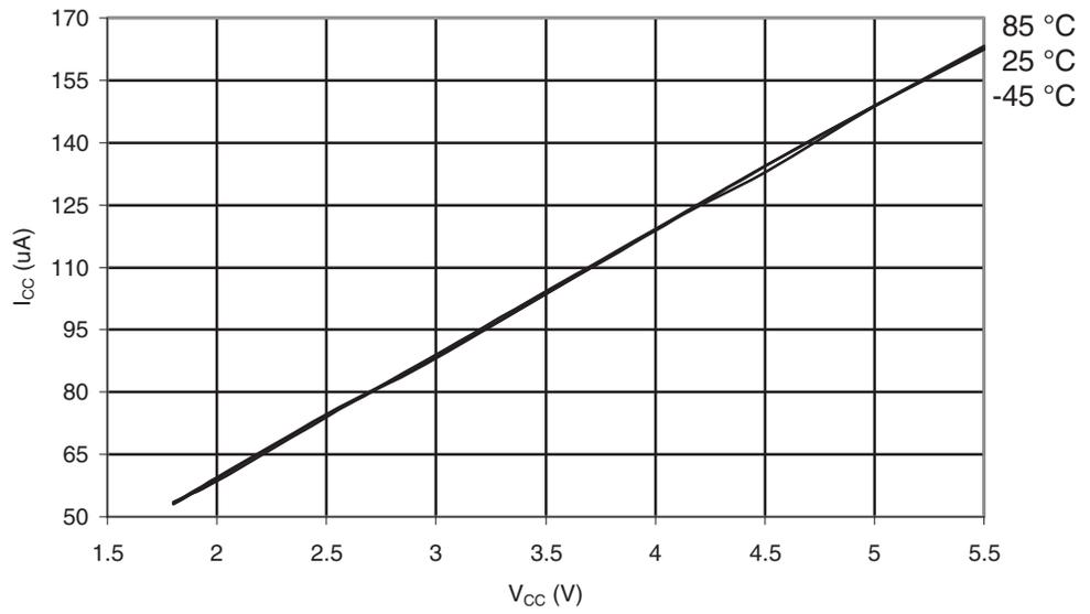
**Figure 30-542.** ATmega6490A: Watchdog Timer Current vs.  $V_{CC}$
