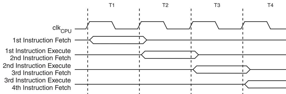
Figure 7-5 shows the internal timing concept for the Register File. In a single clock cycle an ALU operation using two register operands is executed, and the result is stored back to the destination register.
