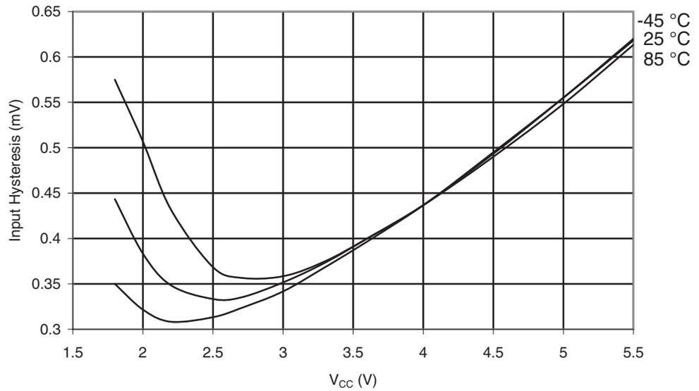
**Figure 30-99.** ATmega169PA: Reset Input Threshold Voltage vs.  $V_{CC}$  ( $V_{IH}$ , Reset Pin Read as "1")
