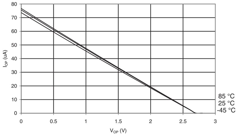
**Figure 30-18.** ATmega169A: I/O Pin Pull-up Resistor Current vs. Input Voltage ( $V_{CC} = 1.8V$ )
