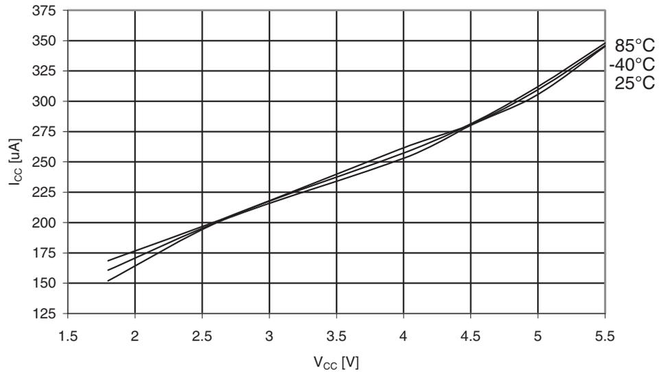
**Figure 30-297.** ATmega3290A: Active Supply Current with ADC at 1MHz vs.  $V_{CC}$
