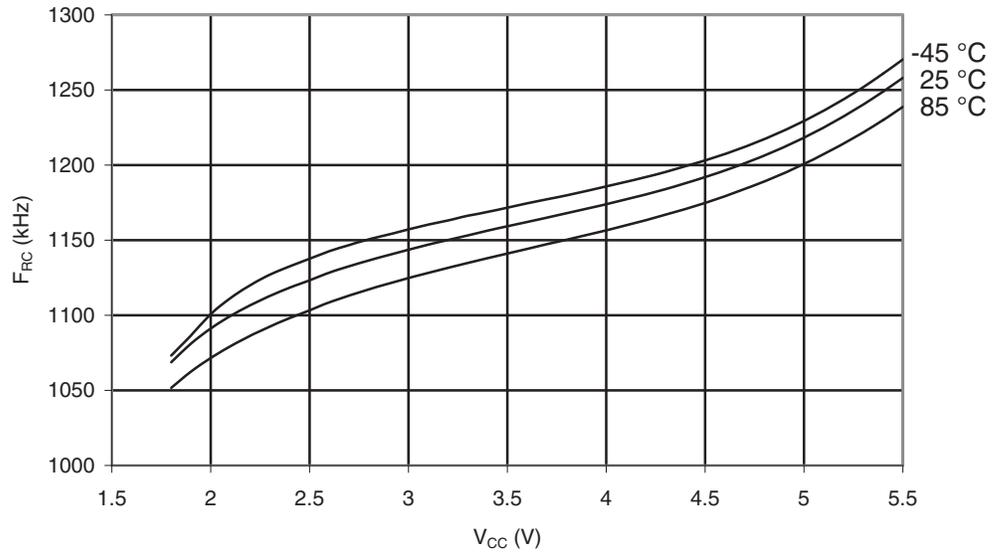
**Figure 30-110.** ATmega169PA: Watchdog Oscillator Frequency vs. Temperature
