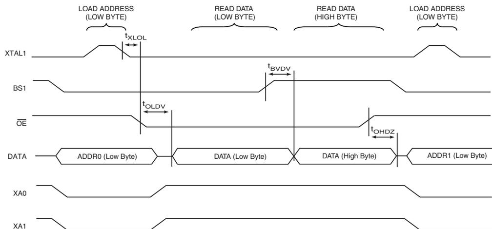
Note: 1. The timing requirements shown in Figure 28-7 on page 323 (i.e.,  $t_{DVXH}$ ,  $t_{XHXL}$ , and  $t_{XLDX}$ ) also apply to reading operation.
