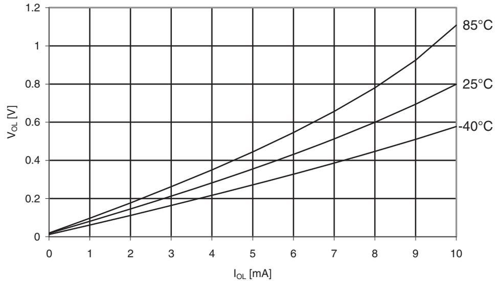
**Figure 30-334.** ATmega3290PA: I/O Pin Output Voltage vs. Sink Current, Ports A, C, D, E, F, G ( $V_{CC} = 1.8V$ )
