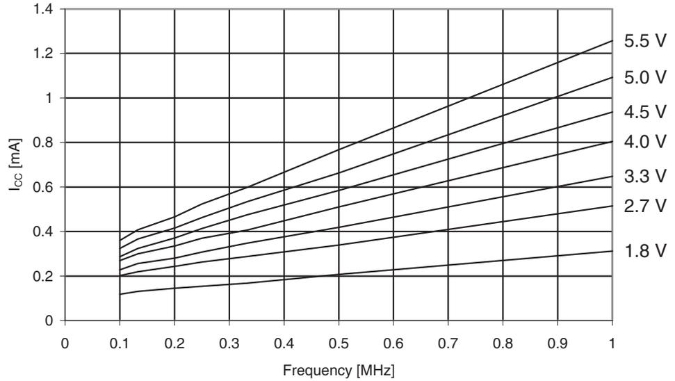
**Figure 30-126.** ATmega329A: Active Supply Current vs. Frequency (1 - 20MHz)
