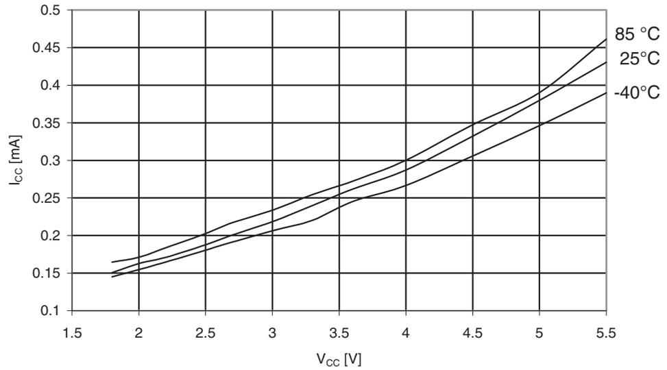
**Figure 30-194.** ATmega329PA: Idle Supply Current vs.  $V_{CC}$  (32kHz Watch Crystal)
