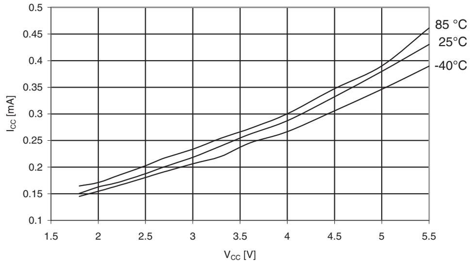
**Figure 30-134.** ATmega329A: Idle Supply Current vs.  $V_{CC}$  (32kHz Watch Crystal)
