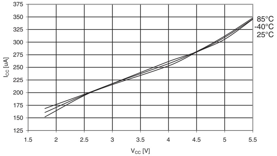
**Figure 30-357.** ATmega3290PA: Active Supply Current with ADC at 1MHz vs.  $V_{CC}$
