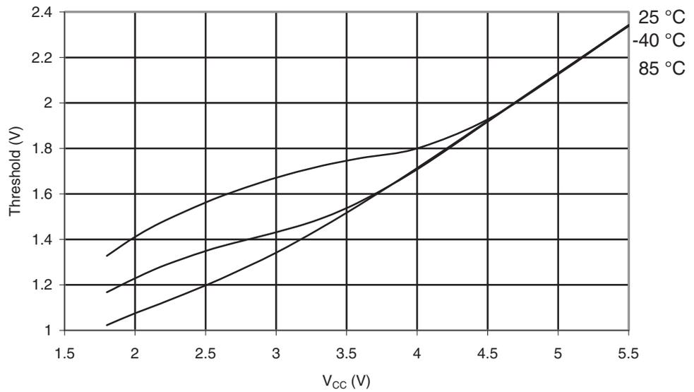
**Figure 30-222.** ATmega329PA: Reset Input Threshold Voltage vs.  $V_{CC}$  ( $V_{IL}$ , Reset Pin Read as "0")
