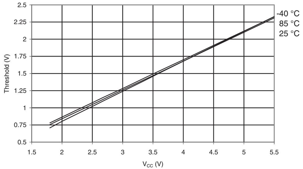
**Figure 30-163.** ATmega329A: Reset Pin Input Hysteresis vs.  $V_{CC}$
