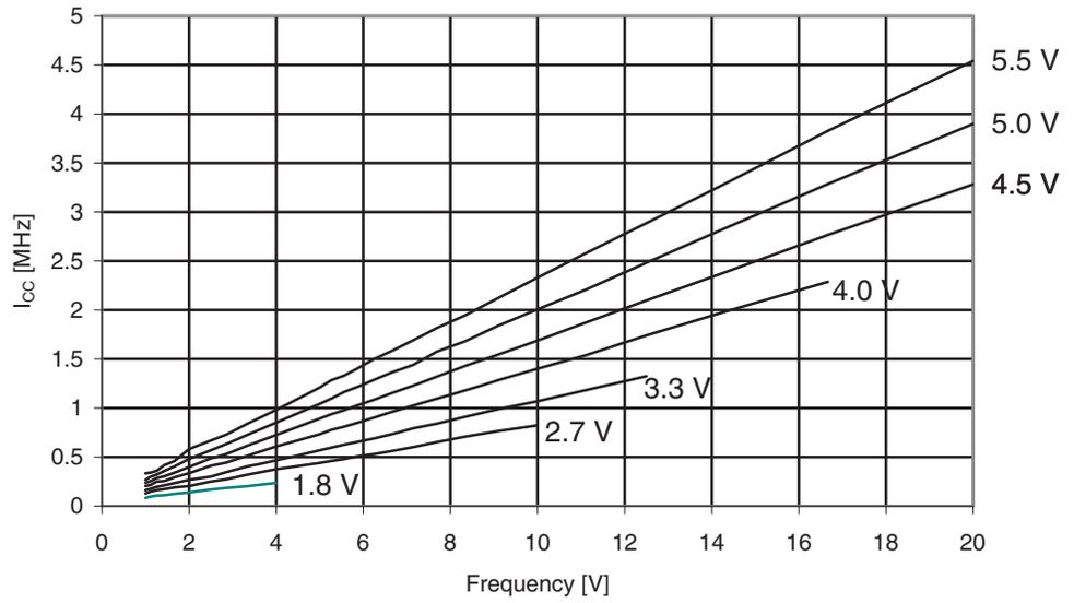
**Figure 30-252.** ATmega3290A: Idle Supply Current vs.  $V_{CC}$  (Internal RC Oscillator, 8MHz)
