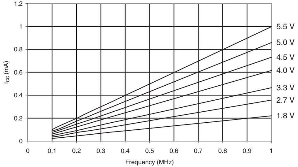
**Figure 30-64.** ATmega169PA: Active Supply Current vs. Frequency (1 - 16MHz)
