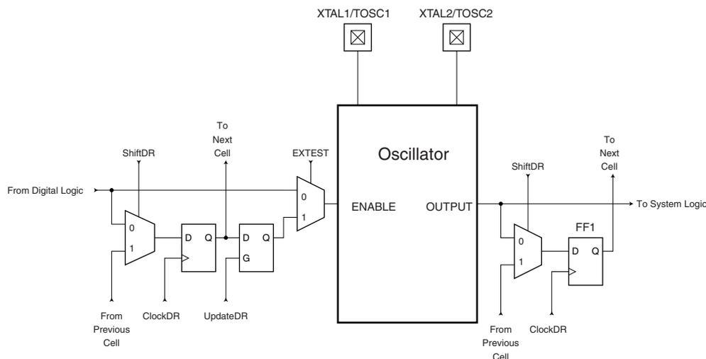
Table 26-2 summarizes the scan registers for the external clock pin XTAL1, oscillators with XTAL1/XTAL2 connections as well as 32kHz Timer Oscillator.
