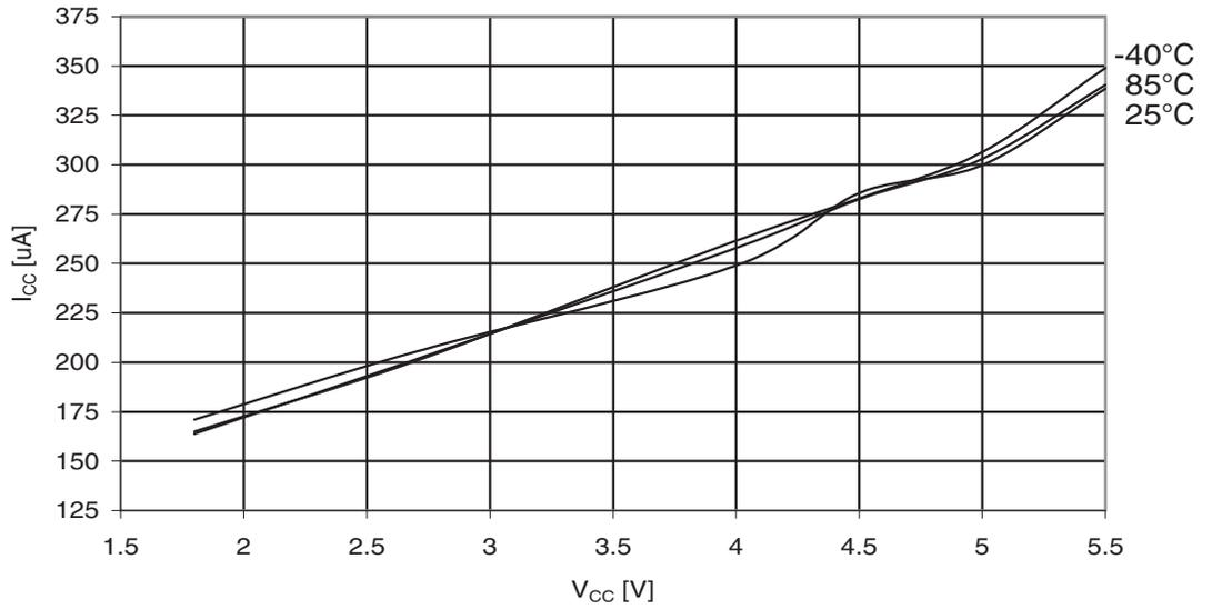
**Figure 30-298.** ATmega3290A: AREF External Reference Current vs.  $V_{CC}$
