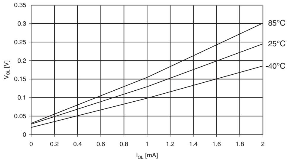
**Figure 30-275.** ATmega3290A: I/O Pin Output Voltage vs. Sink Current, Port B ( $V_{CC} = 5V$ )
