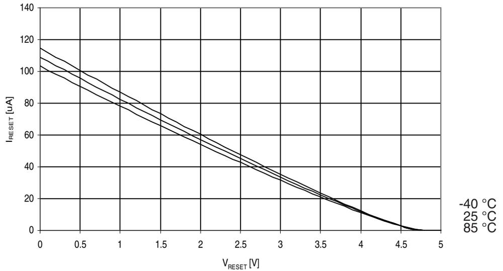
**Figure 30-264.** ATmega3290A: Reset Pull-up Resistor Current vs. Reset Pin Voltage ( $V_{CC}=2.7V$ )
