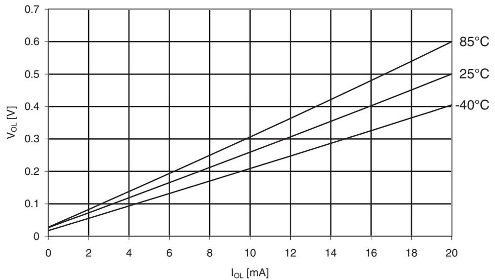
**Figure 30-216.** ATmega329PA: I/O Pin Output Voltage vs. Sink Current, Port B ( $V_{CC} = 2.7V$ )
