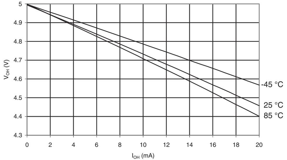
**Figure 30-391.** ATmega649A: I/O Pin Output Voltage vs. Source Current, Port B ( $V_{CC} = 2.7V$ )
