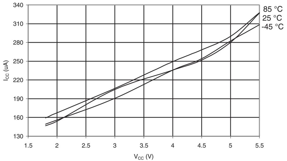
Figure 30-602. ATmega6490P: AREF External Reference Current vs.  $V_{CC}$
