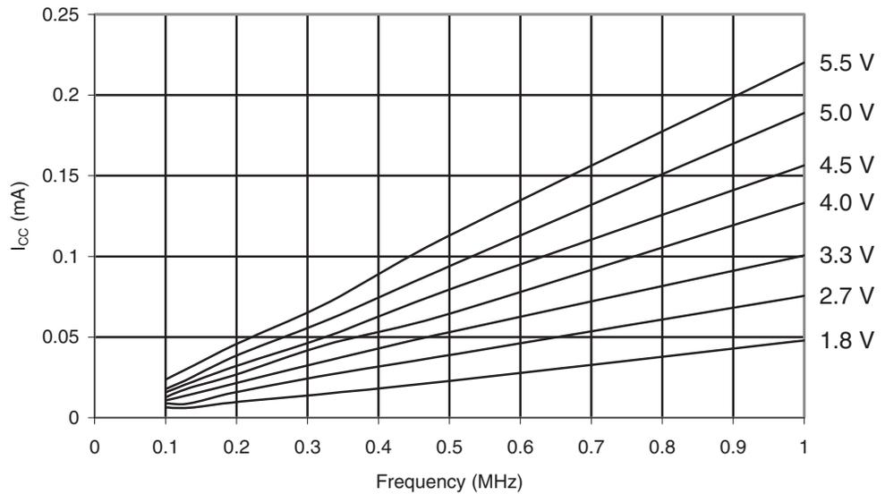
**Figure 30-69.** ATmega169PA: Idle Supply Current vs. Frequency (1 - 16MHz)
