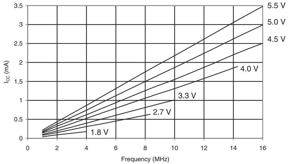
**Figure 30-70.** ATmega169PA: Idle Supply Current vs.  $V_{CC}$  (Internal RC Oscillator, 8MHz)
