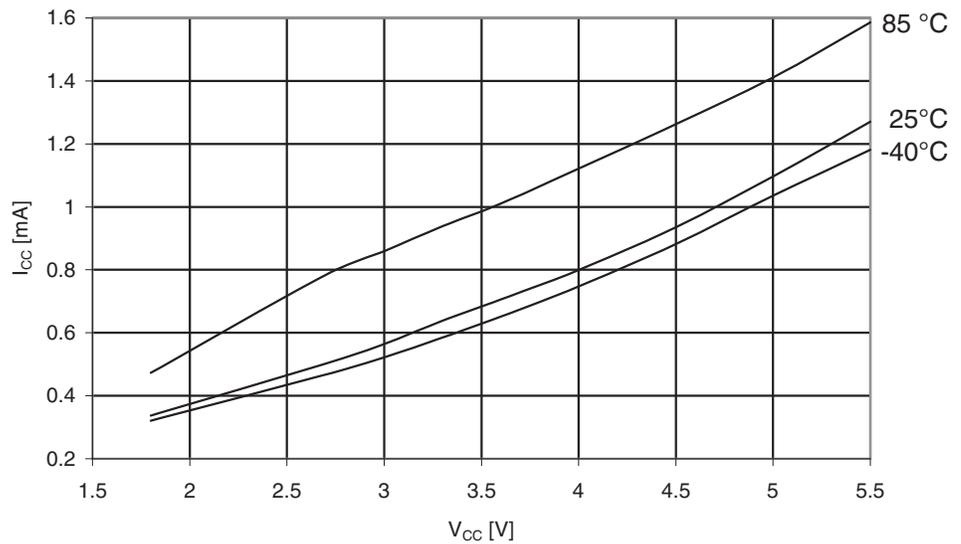
**Figure 30-129.** ATmega329A: Active Supply Current vs.  $V_{CC}$  (32kHz Watch Crystal)
