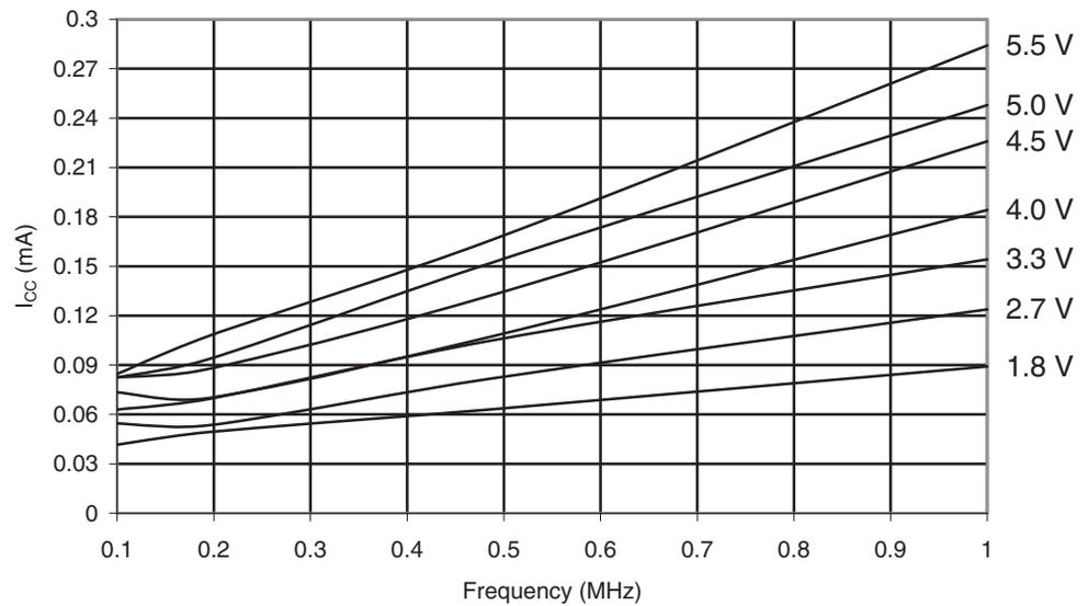
**Figure 30-432.** ATmega649P: Idle Supply Current vs. Frequency (1 - 20MHz)
