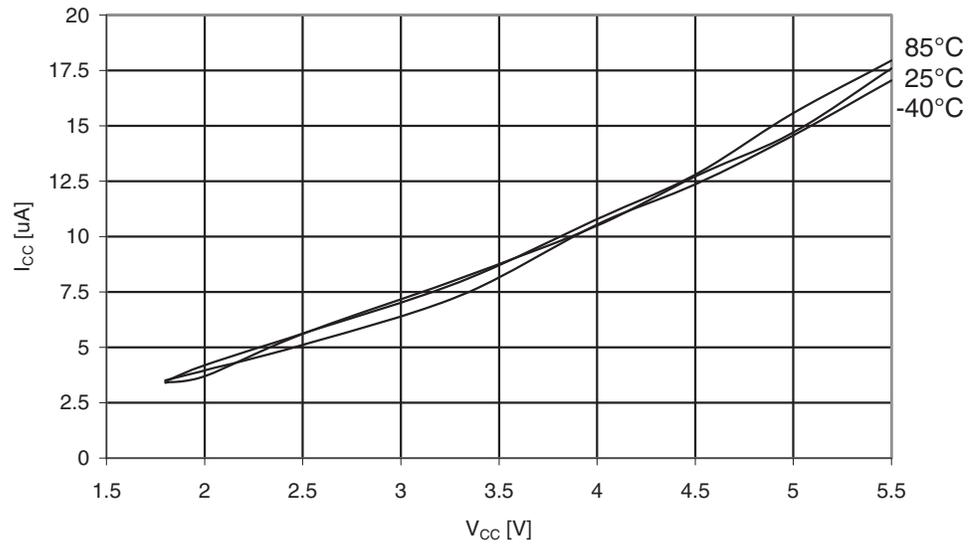
**Figure 30-300.** ATmega3290A: Analog Comparator Current vs.  $V_{CC}$
