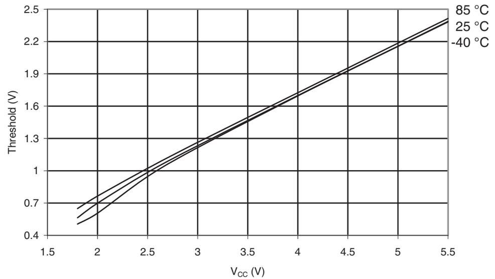
**Figure 30-160.** ATmega329A: I/O Pin Input Hysteresis vs.  $V_{CC}$
