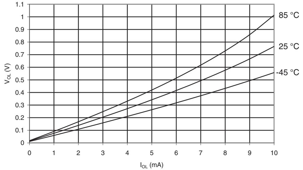
**Figure 30-92.** ATmega169PA: I/O Pin Output Voltage vs. Sink Current, Ports A, C, D, E, F, G
