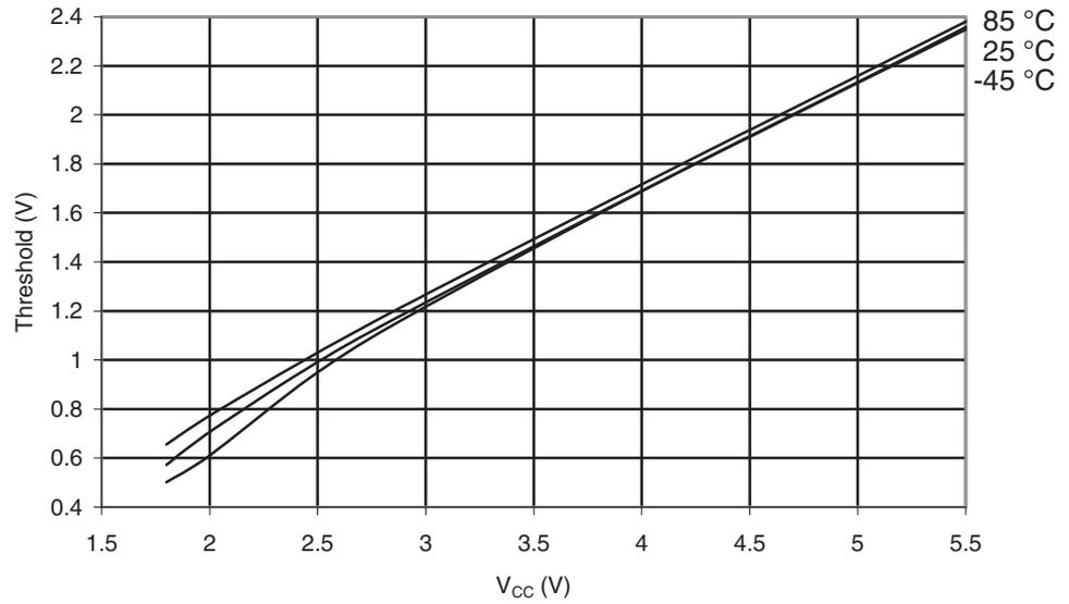
**Figure 30-401.** ATmega649A: I/O Pin Input Hysteresis vs.  $V_{CC}$
