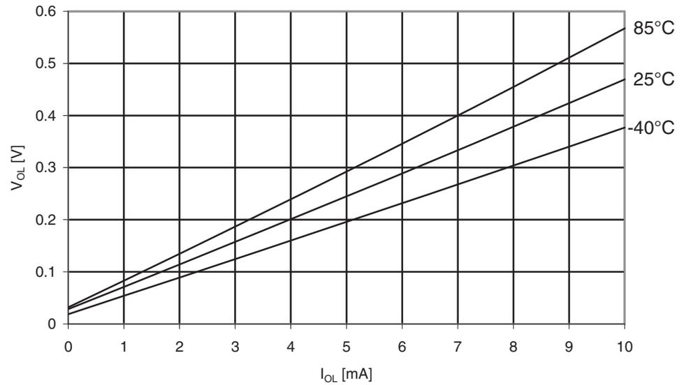
**Figure 30-273.** ATmega3290A. I/O Pin Output Voltage vs. Sink Current, Ports A, C, D, E, F, G
