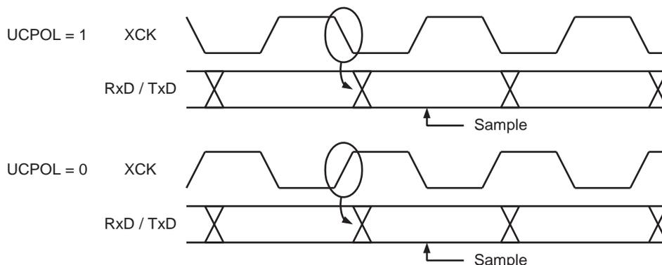
The UCPOLn bit UCRSC selects which XCK clock edge is used for data sampling and which is used for data change. As [Figure 20-3](#) shows, when UCPOLn is zero the data will be changed at rising XCK edge and sampled at falling XCK edge. If UCPOLn is set, the data will be changed at falling XCK edge and sampled at rising XCK edge.
