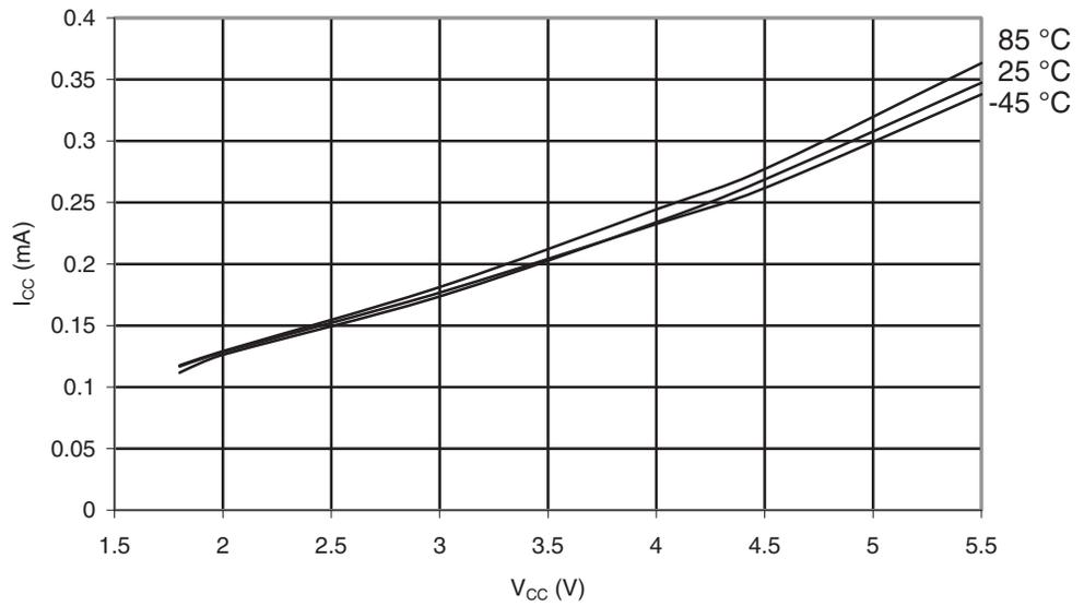
**Figure 30-72.** ATmega169PA: Idle Supply Current vs.  $V_{CC}$  (32kHz Watch Crystal)
