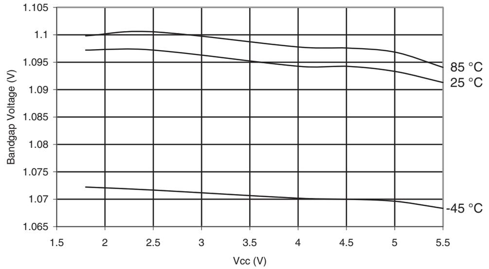
**Figure 30-106.** ATmega169PA: Bandgap Voltage vs. Temperature
