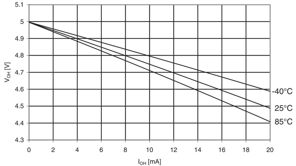
**Figure 30-210.** ATmega329PA: I/O Pin Output Voltage vs. Source Current, Port B ( $V_{CC} = 2.7V$ )
