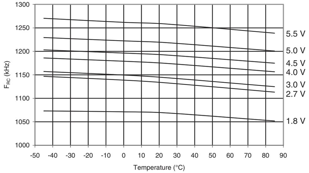
**Figure 30-49.** ATmega169A: Calibrated 8MHz RC Oscillator Frequency vs. Temperature
