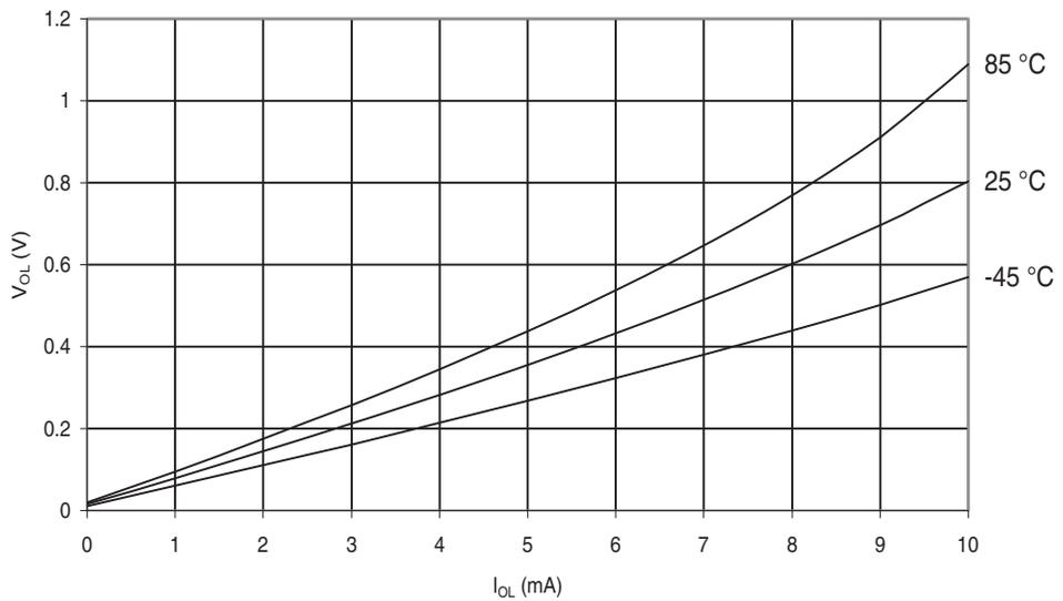
**Figure 30-456.** ATmega649P: I/O Pin Output Voltage vs. Sink Current, Ports A, C, D, E, F, G ( $V_{CC} = 1.8V$ )
