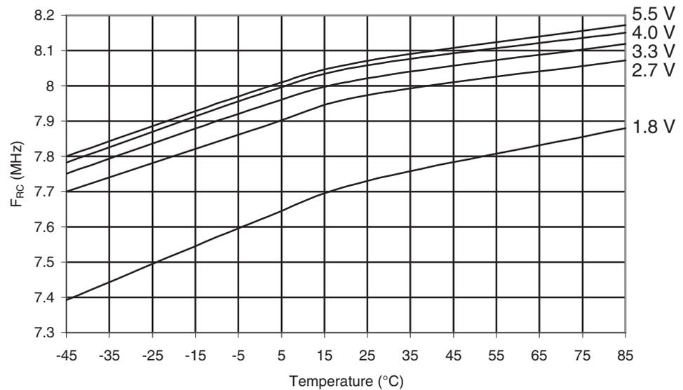
**Figure 30-596.** ATmega6490P: Calibrated 8MHz RC Oscillator Frequency vs.  $V_{CC}$
