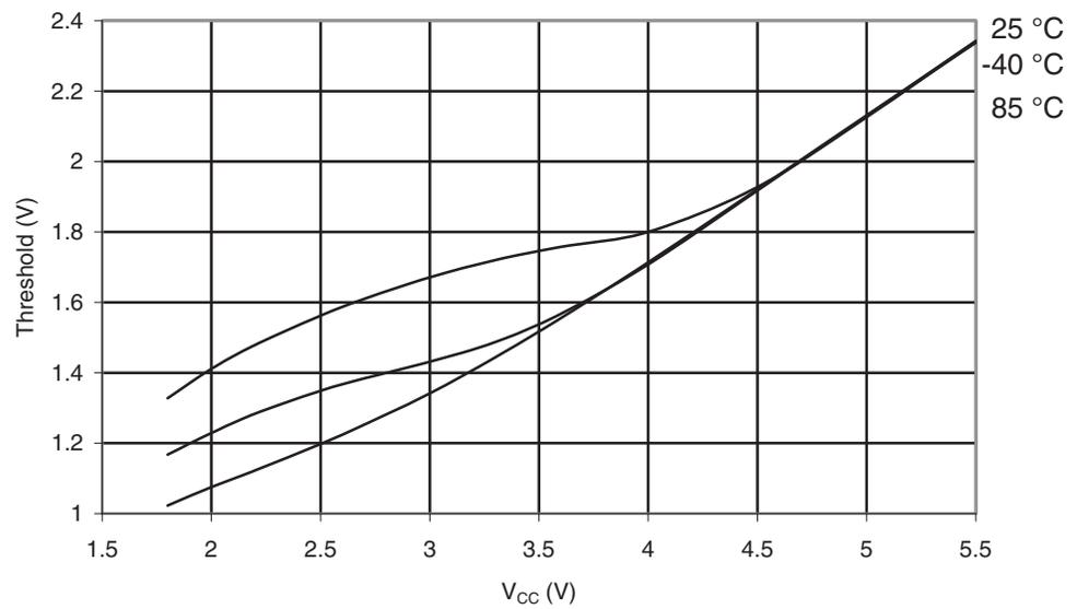
**Figure 30-162.** ATmega329A: Reset Input Threshold Voltage vs.  $V_{CC}$  ( $V_{IL}$ , Reset Pin Read as "0")
