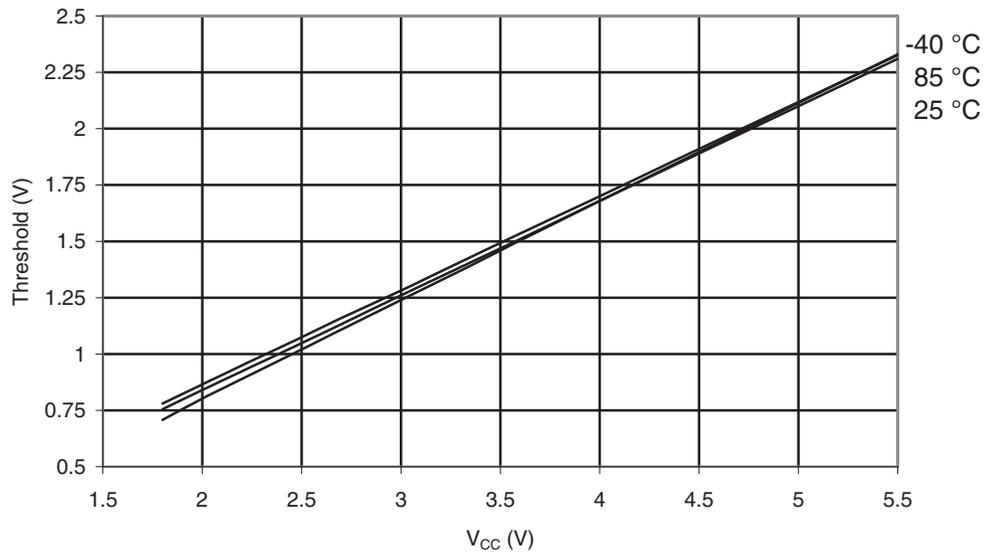
**Figure 30-343.** ATmega3290PA: Reset Input Pin Hysteresis vs.  $V_{CC}$
