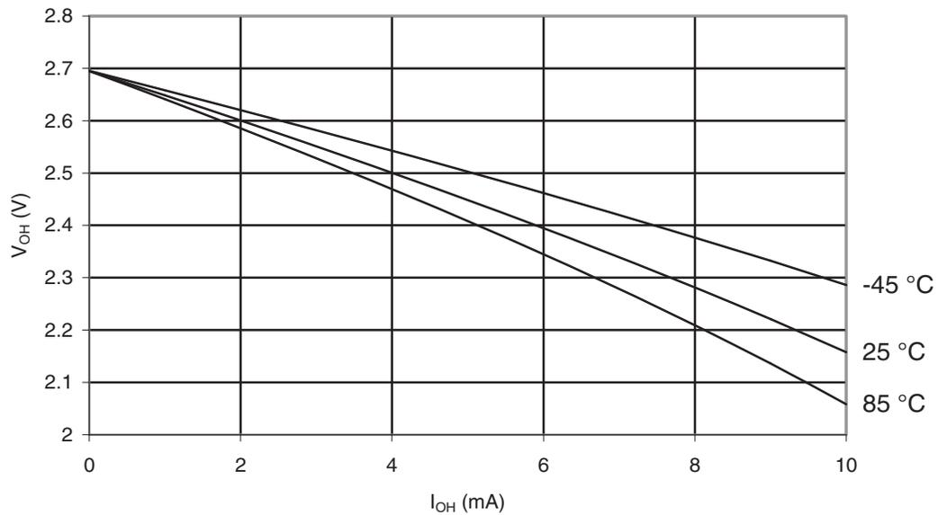
**Figure 30-24.** ATmega169A: I/O Pin Output Voltage vs. Source Current, Ports A, C, D, E, F, G ( $V_{CC} = 1.8V$ )
