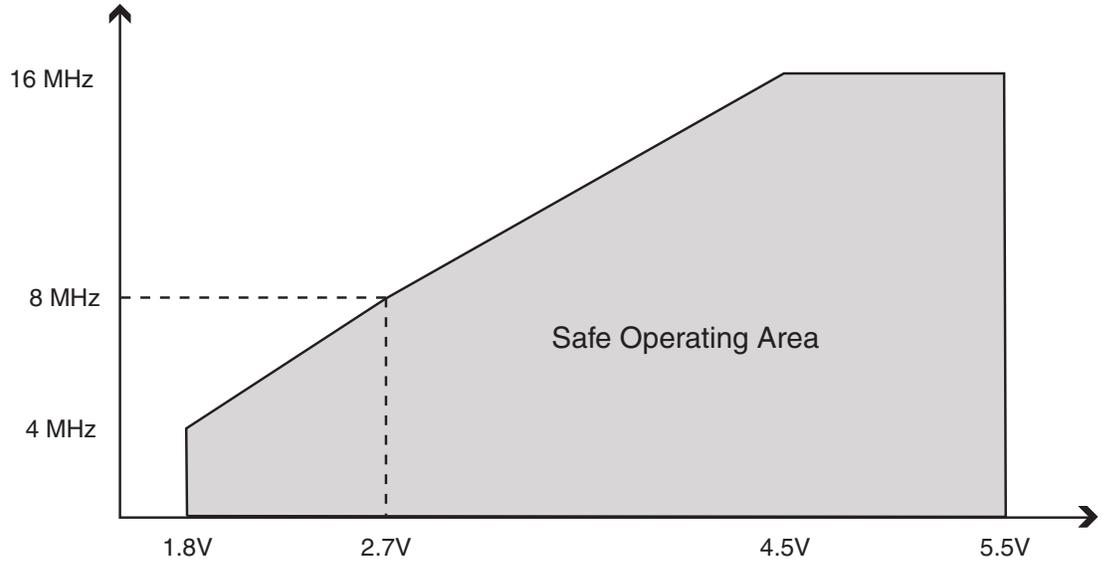
**Figure 29-2.** Maximum Frequency vs.  $V_{CC}$  (0 - 20MHz)
