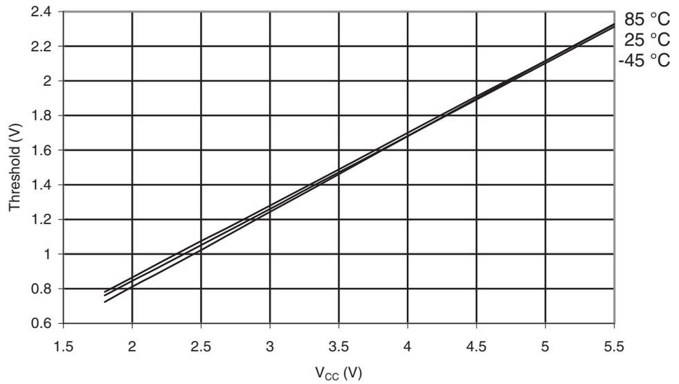
**Figure 30-39.** ATmega169A: Reset Input Pin Hysteresis vs.  $V_{CC}$
