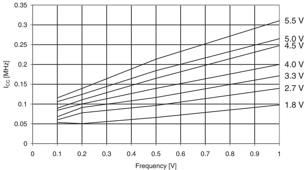
**Figure 30-131.** ATmega329A: Idle Supply Current vs. Frequency (1 - 20MHz)
