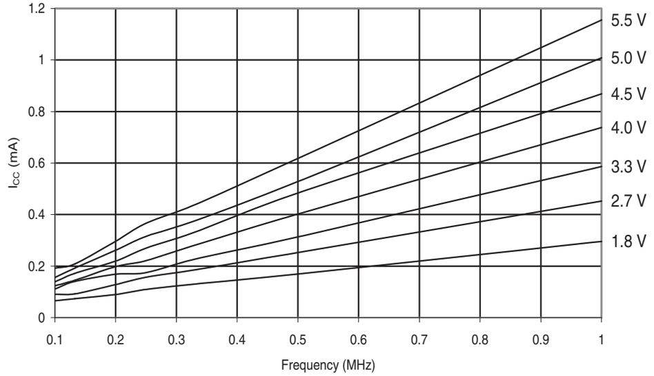
**Figure 30-427.** ATmega649P: Active Supply Current vs. Frequency (1 - 20MHz)
