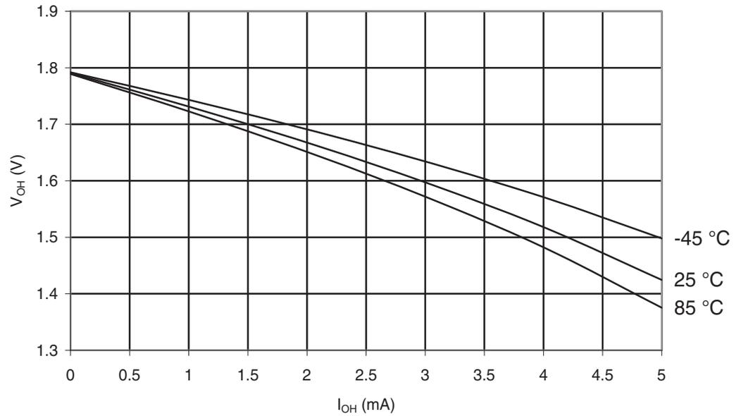
**Figure 30-90.** ATmega169PA: I/O Pin Output Voltage vs. Sink Current, Ports A, C, D, E, F, G ( $V_{CC} = 5V$ )
