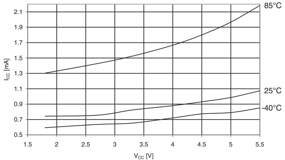
**Figure 30-259.** ATmega3290A: Standby Supply Current vs.  $V_{CC}$  (Xtall and Resonator, Watchdog Timer Disabled)
