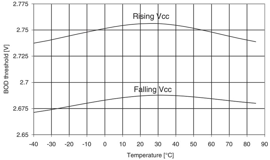
**Figure 30-286.** ATmega3290A: BOD Thresholds vs. Temperature (BOD Level is 1.8V)
