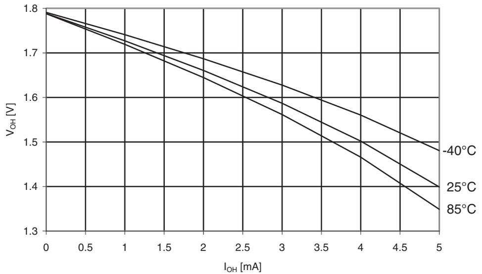
**Figure 30-152.** ATmega329A: I/O Pin Output Voltage vs. Sink Current, Ports A, C, D, E, F, G
