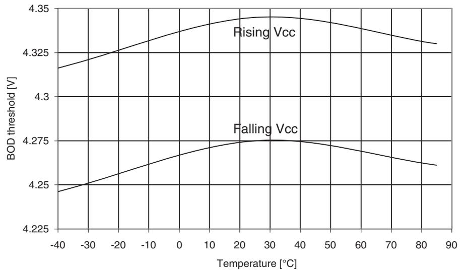
**Figure 30-285.** ATmega3290A: BOD Thresholds vs. Temperature (BOD Level is 2.7V)
