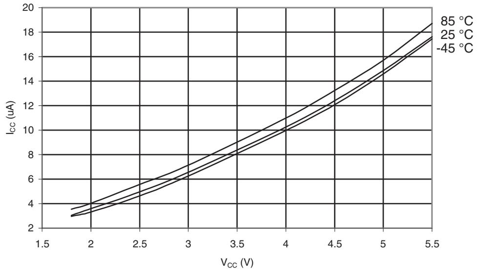
**Figure 30-438.** ATmega649P: Power-down Supply Current vs.  $V_{CC}$  (32kHz Watch Crystal)
