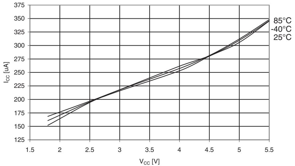
**Figure 30-237.** ATmega329PA: Active Supply Current with ADC at 1MHz vs.  $V_{CC}$
