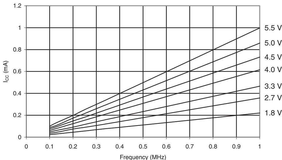
**Figure 30-2.** ATmega169A: Active Supply Current vs. Frequency (1 - 16MHz)
