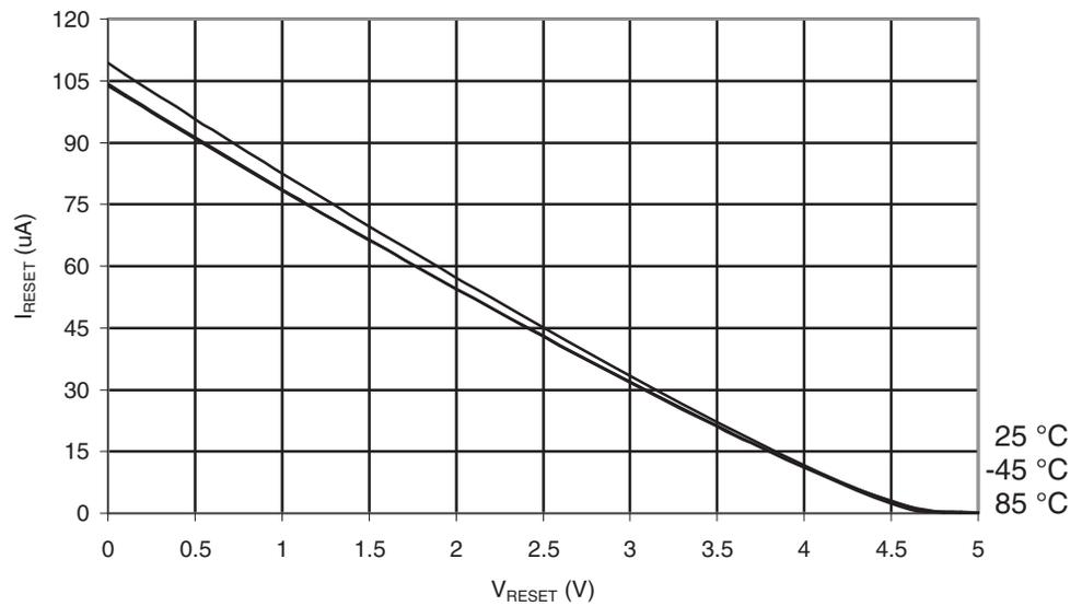
**Figure 30-568.** ATmega6490P: Reset Pull-up Resistor Current vs. Reset Pin Voltage ( $V_{CC} = 2.7V$ )
