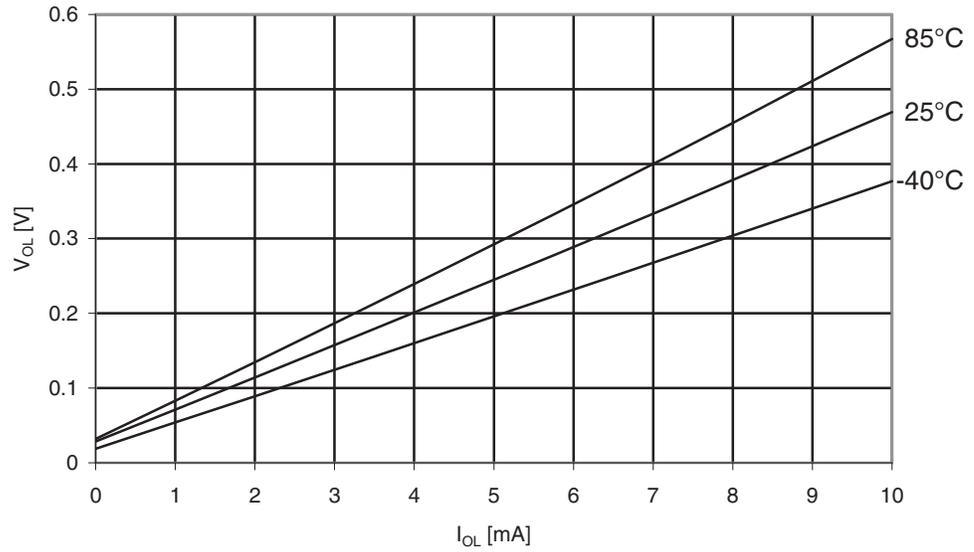
**Figure 30-333.** ATmega3290PA: I/O Pin Output Voltage vs. Sink Current, Ports A, C, D, E, F, G
