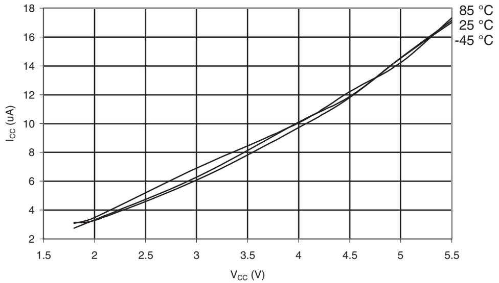
**Figure 30-543.** ATmega6490A: Analog Comparator Current vs.  $V_{CC}$
