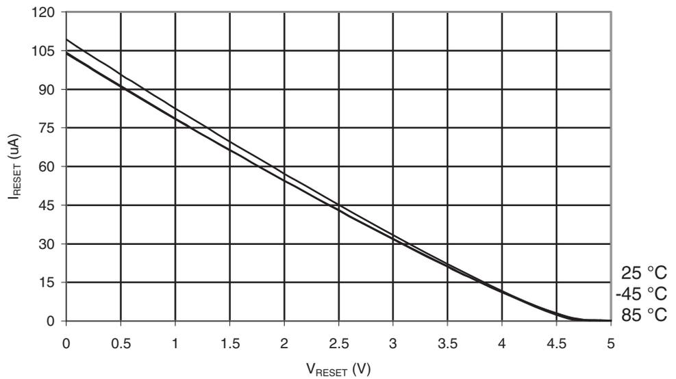
**Figure 30-507.** ATmega6490A: Reset Pull-up Resistor Current vs. Reset Pin Voltage ( $V_{CC} = 2.7V$ )
