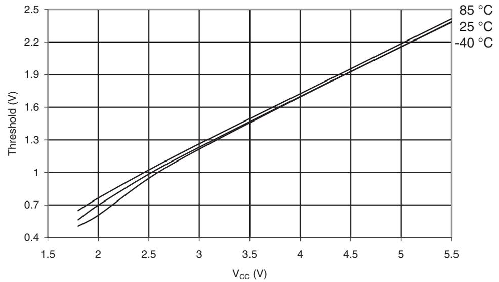
**Figure 30-220.** ATmega329PA: I/O Pin Input Hysteresis vs.  $V_{CC}$
