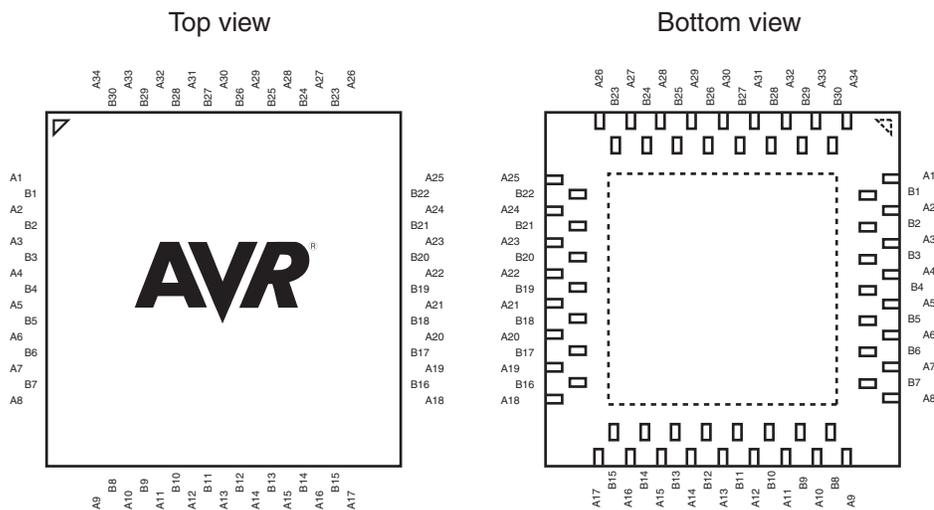
Table 1-1. DRQFN-64 Pinout ATmega169A/ATmega169PA
