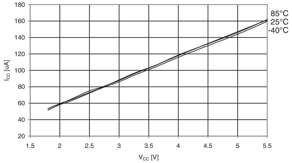
Figure 30-179. ATmega329A: Watchdog Timer Current vs.  $V_{CC}$
