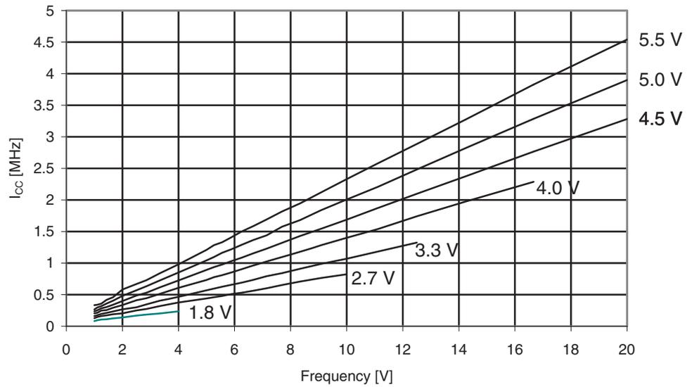
**Figure 30-132.** ATmega329A: Idle Supply Current vs.  $V_{CC}$  (Internal RC Oscillator, 8MHz)
