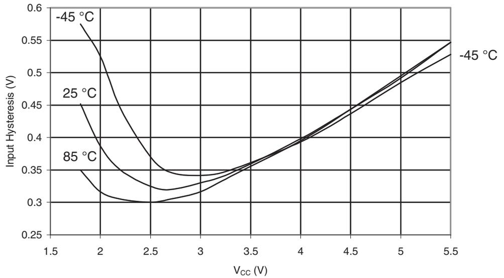
**Figure 30-585.** ATmega6490P: Reset Input Threshold Voltage vs.  $V_{CC}$  ( $V_{IH,Reset}$  Pin Read as "1")
