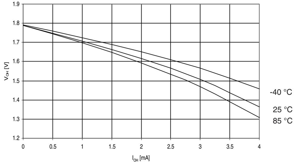
**Figure 30-329.** ATmega3290PA: I/O Pin Output Voltage vs. Source Current, Port B ( $V_{CC} = 5V$ )
