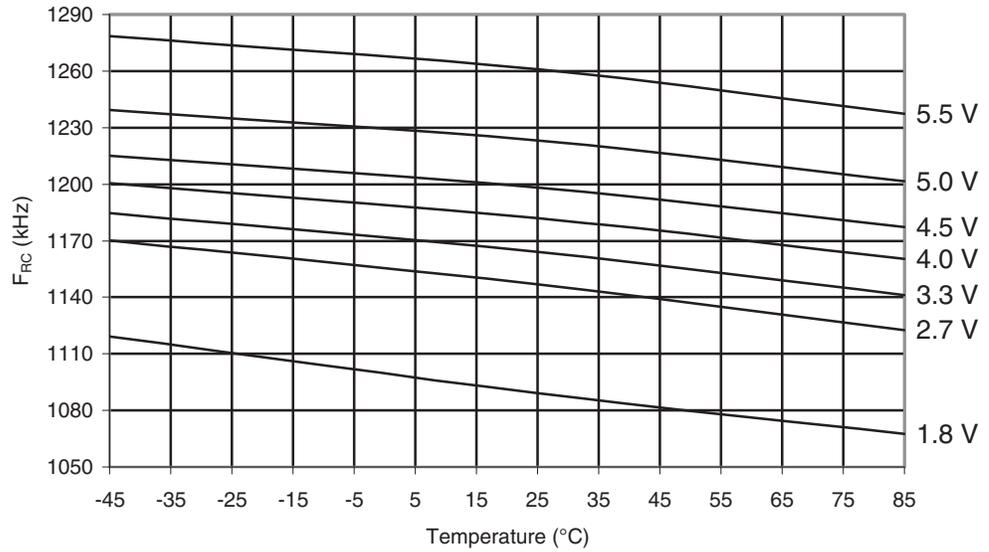
**Figure 30-534.** ATmega6490A: Calibrated 8MHz RC Oscillator Frequency vs. Temperature
