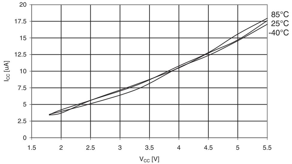
**Figure 30-180.** ATmega329A: Analog Comparator Current vs.  $V_{CC}$
