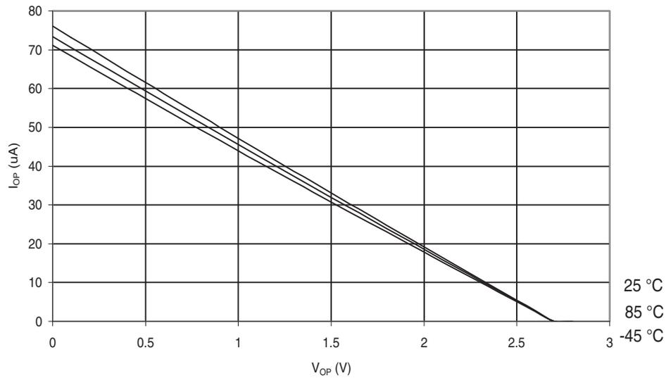
**Figure 30-444.** ATmega649P: I/O Pin Pull-up Resistor Current vs. Input Voltage ( $V_{CC} = 1.8V$ )
