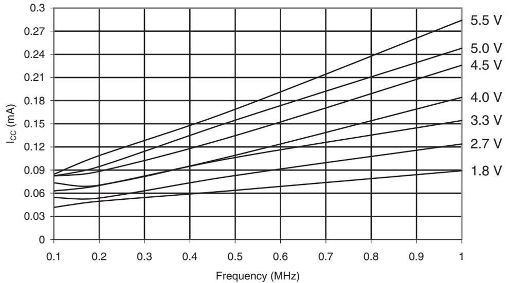
**Figure 30-371.** ATmega649A: Idle Supply Current vs. Frequency (1 - 20MHz)
