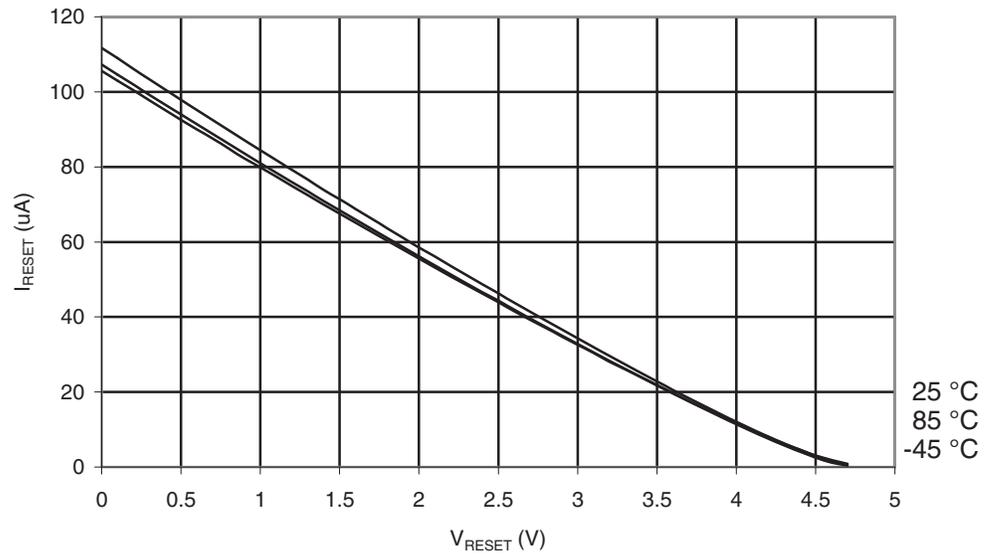
**Figure 30-82.** ATmega169PA: Reset Pull-up Resistor Current vs. Reset Pin Voltage ( $V_{CC} = 2.7V$ )
