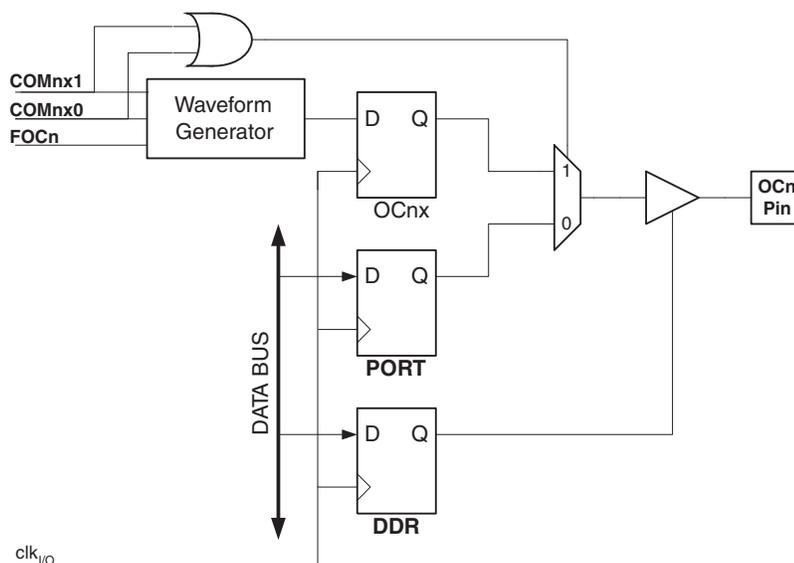
The general I/O port function is overridden by the Output Compare (OC0A) from the Waveform Generator if either of the COM0A1:0 bits are set. However, the OC0A pin direction (input or output) is still controlled by the Data Direction Register (DDR) for the port pin. The Data Direction Register bit for the OC0A pin (DDR\_OC0A) must be set as output before the OC0A value is visible on the pin. The port override function is independent of the Waveform Generation mode.
