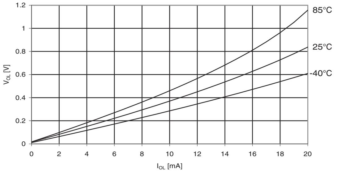
**Figure 30-337.** ATmega3290PA: I/O Pin Output Voltage vs. Sink Current, Port B ( $V_{CC} = 1.8V$ )
