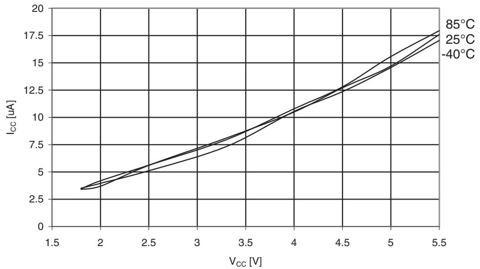
**Figure 30-240.** ATmega329PA: Analog Comparator Current vs.  $V_{CC}$
