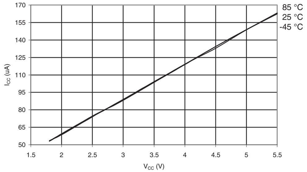
Figure 30-603. ATmega6490P: Watchdog Timer Current vs.  $V_{CC}$
