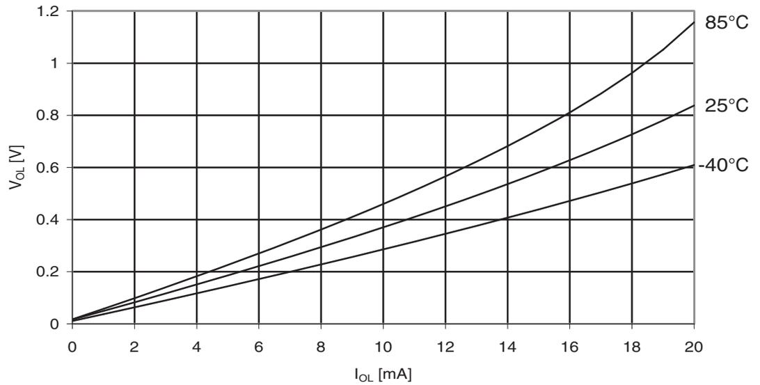
**Figure 30-277.** ATmega3290A: I/O Pin Output Voltage vs. Sink Current, Port B ( $V_{CC} = 1.8V$ )
