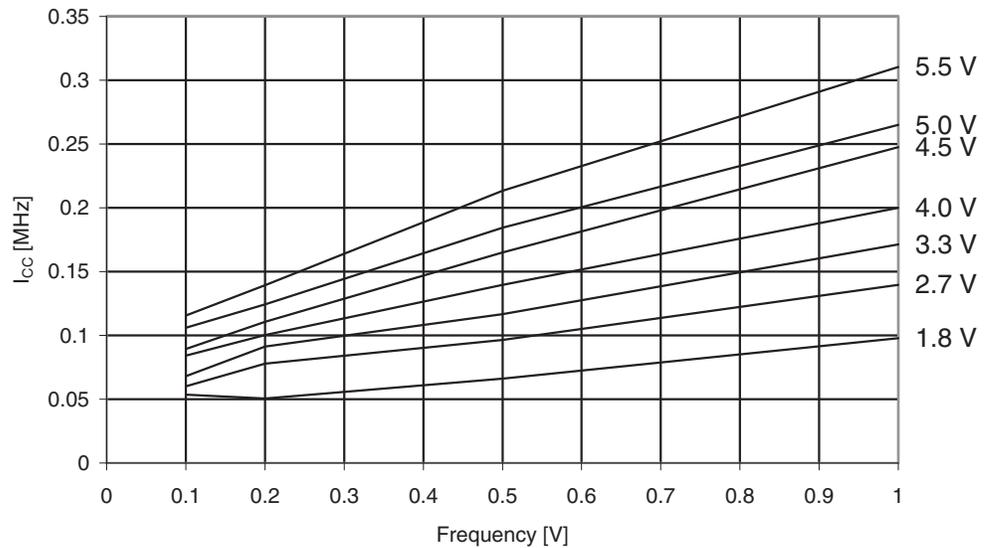
**Figure 30-191.** ATmega329PA: Idle Supply Current vs. Frequency (1 - 20MHz)
