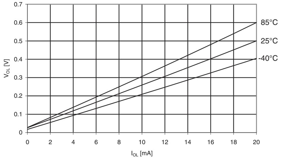
**Figure 30-156.** ATmega329A: I/O Pin Output Voltage vs. Sink Current, Port B ( $V_{CC} = 2.7V$ )
