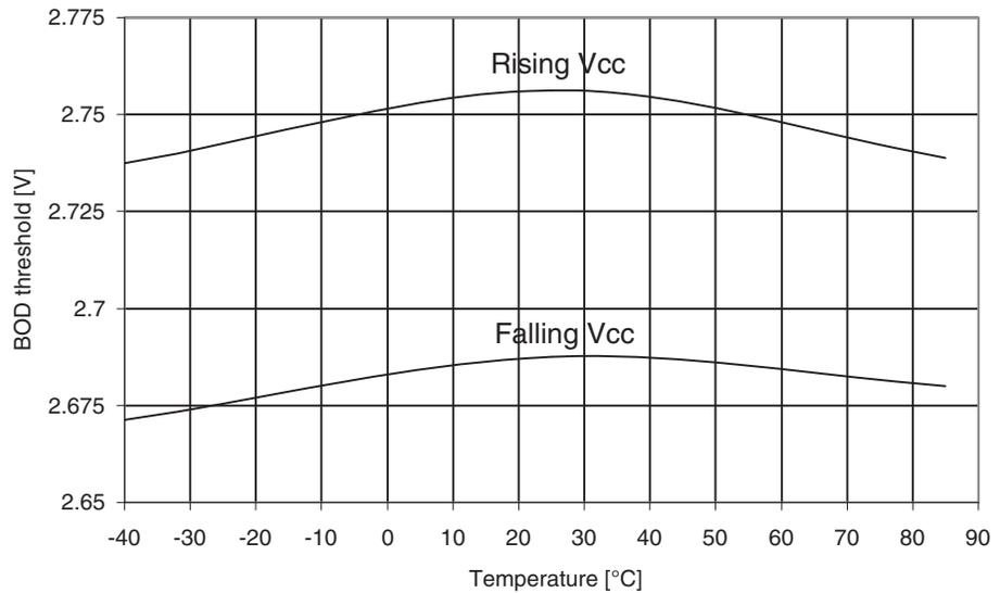
**Figure 30-166.** ATmega329A: BOD Thresholds vs. Temperature (BOD Level is 1.8V)
