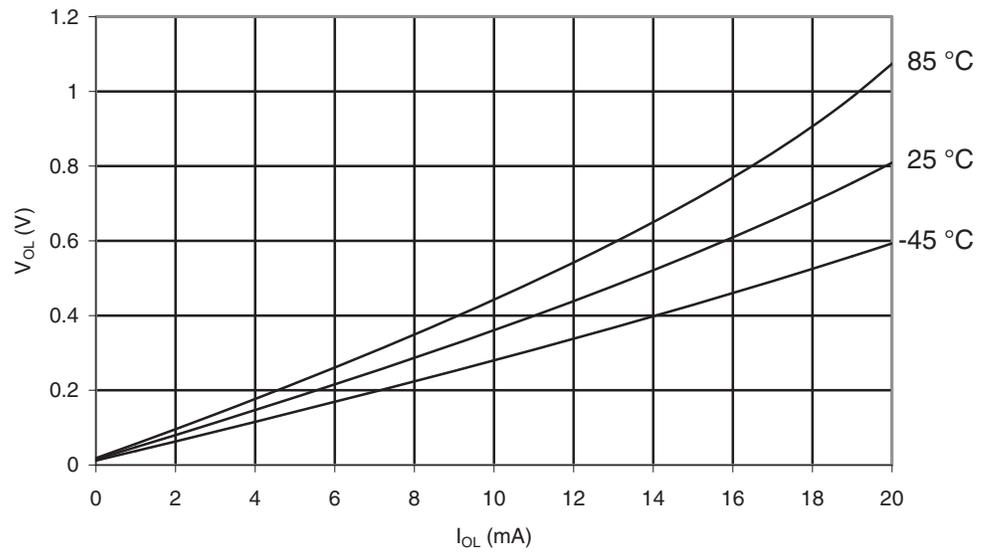
**Figure 30-95.** ATmega169PA: I/O Pin Output Voltage vs. Sink Current, Port B ( $V_{CC} = 1.8V$ )
