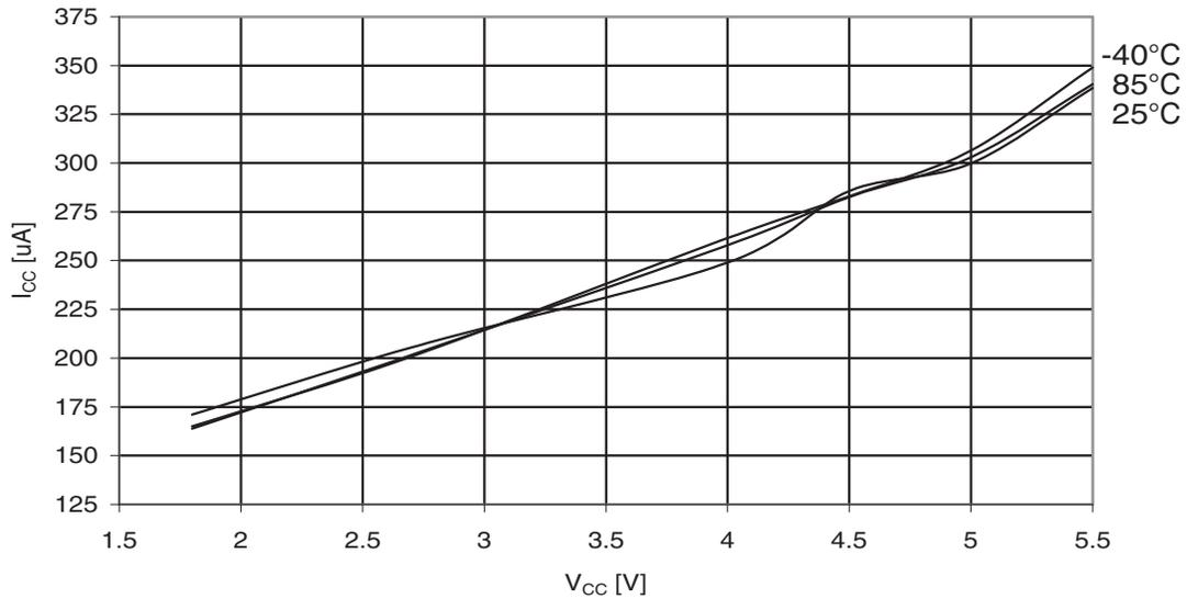
Figure 30-238. ATmega329PA: AREF External Reference Current vs.  $V_{CC}$
