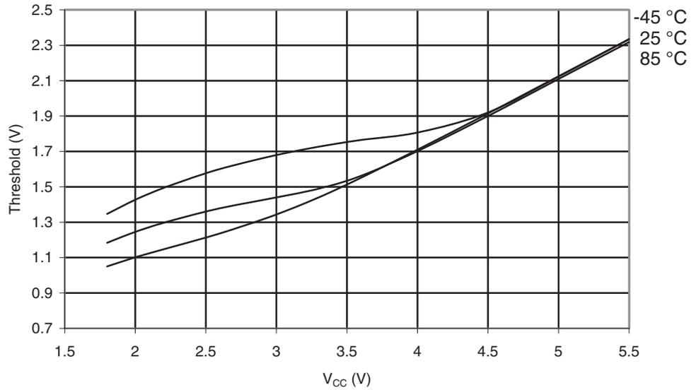
**Figure 30-38.** ATmega169A: Reset Input Threshold Voltage vs.  $V_{CC}$  ( $V_{IL}$ , Reset Pin Read as "0")
