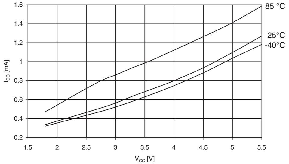
**Figure 30-189.** ATmega329PA: Active Supply Current vs.  $V_{CC}$  (32kHz Watch Crystal)
