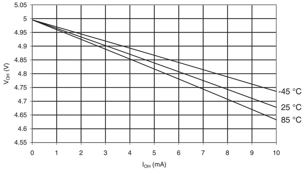
**Figure 30-85.** ATmega169PA: I/O Pin Output Voltage vs. Source Current, Ports A, C, D, E, F, G
