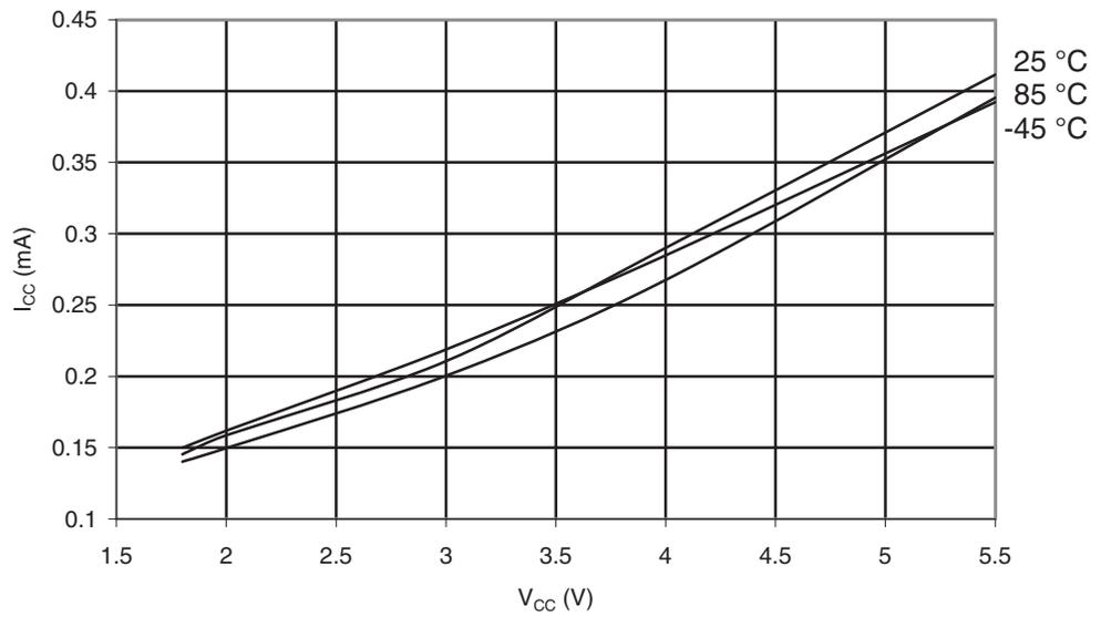
**Figure 30-491.** ATmega6490A: Active Supply Current vs.  $V_{CC}$  (32kHz Watch Crystal)
