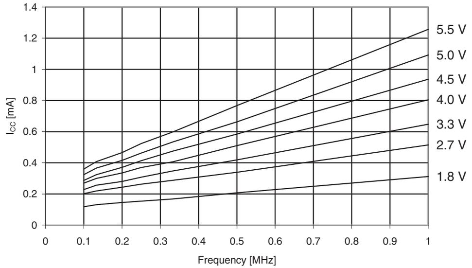
**Figure 30-246.** ATmega3290A: Active Supply Current vs. Frequency (1 - 20MHz)
