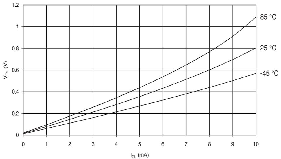
**Figure 30-395.** ATmega649A: I/O Pin Output Voltage vs. Sink Current, Ports A, C, D, E, F, G ( $V_{CC} = 1.8V$ )
