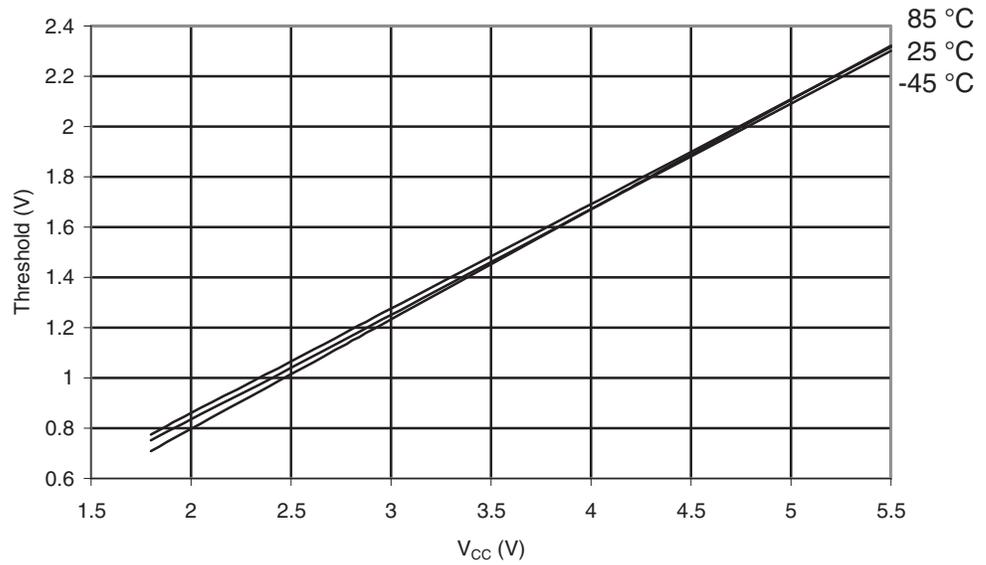
**Figure 30-526.** ATmega6490A: Reset Input Pin Hysteresis vs.  $V_{CC}$
