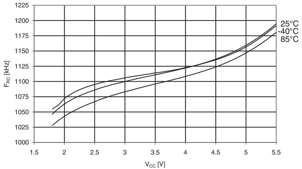
**Figure 30-290.** ATmega3290A: Watchdog Oscillator Frequency vs. Temperature
