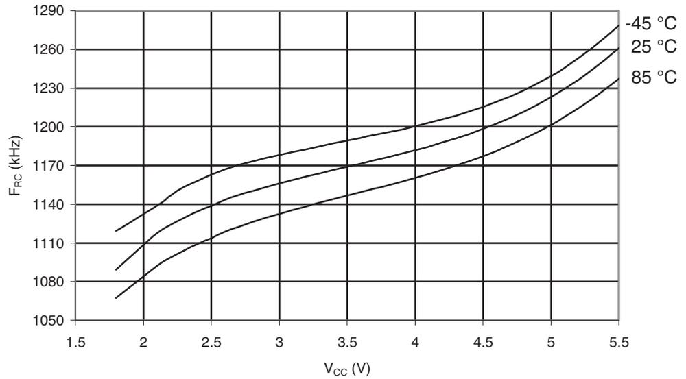
**Figure 30-594.** ATmega6490P: Watchdog Oscillator Frequency vs. Temperature
