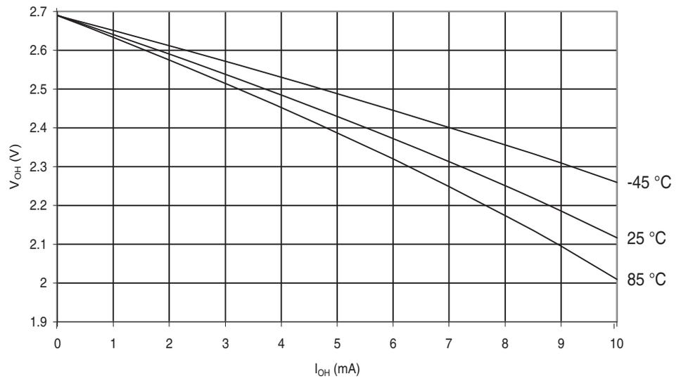
**Figure 30-572.** ATmega6490P: I/O Pin Output Voltage vs. Source Current, Ports A, C, D, E, F, G ( $V_{CC}=1.8V$ )
