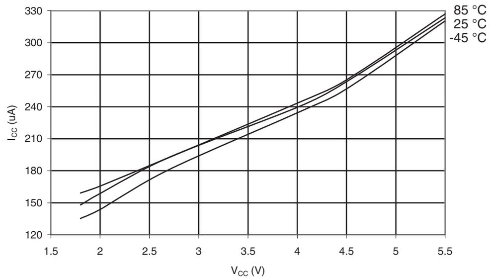
**Figure 30-417.** ATmega649A: Active Supply Current with ADC at 200kHz vs.  $V_{CC}$
