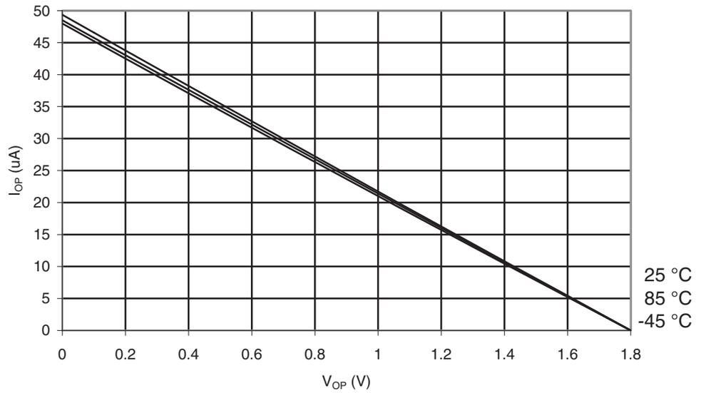
**Figure 30-19.** ATmega169A: Reset Pull-up Resistor Current vs. Reset Pin Voltage ( $V_{CC} = 5V$ )
