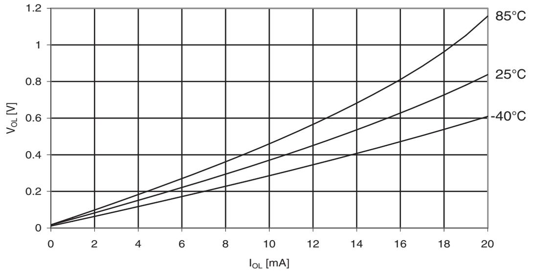
**Figure 30-217.** ATmega329PA: I/O Pin Output Voltage vs. Sink Current, Port B ( $V_{CC} = 1.8V$ )
