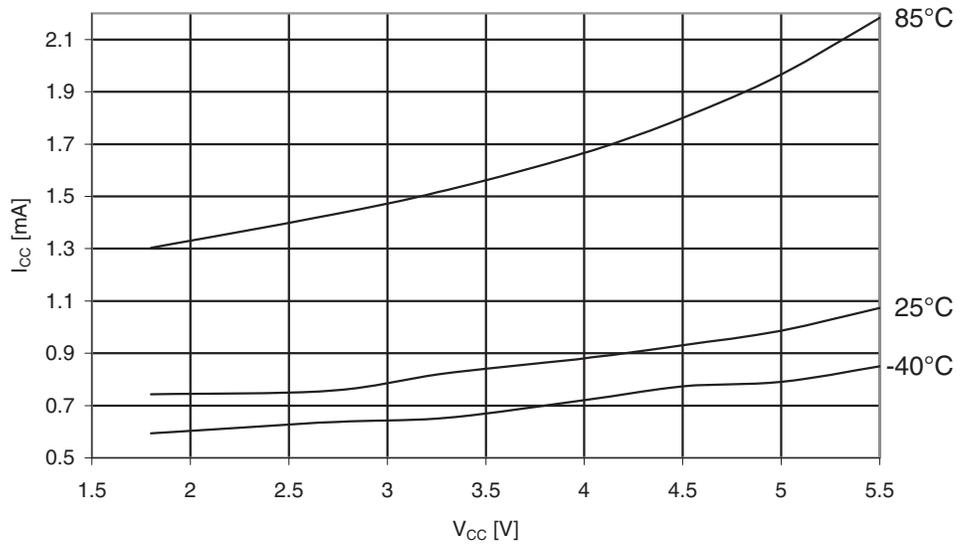
**Figure 30-319.** ATmega3290PA: Standby Supply Current vs.  $V_{CC}$  (Xtall and Resonator, Watchdog Timer Disabled)
