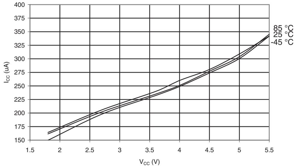
**Figure 30-54.** ATmega169A: Active Supply Current with ADC at 200kHz vs.  $V_{CC}$
