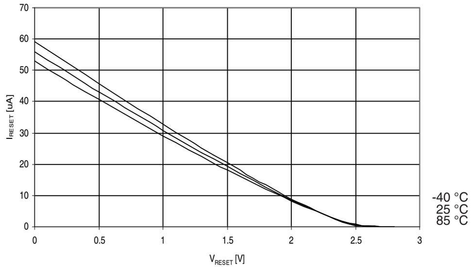
**Figure 30-145.** ATmega329A: Reset Pull-up Resistor Current vs. Reset Pin Voltage ( $V_{CC} = 1.8V$ )
