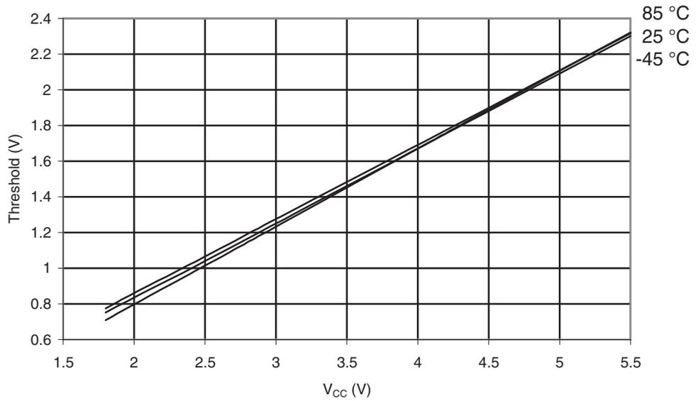
**Figure 30-404.** ATmega649A: Reset Input Pin Hysteresis vs.  $V_{CC}$
