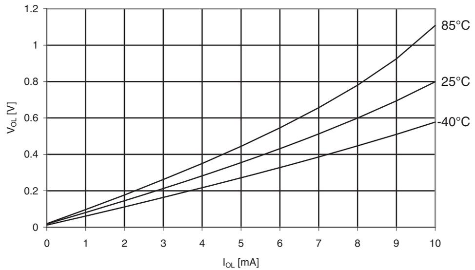
**Figure 30-154.** ATmega329A: I/O Pin Output Voltage vs. Sink Current, Ports A, C, D, E, F, G ( $V_{CC} = 1.8V$ )
