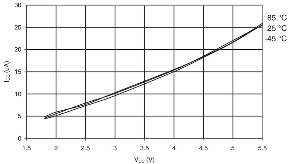
**Figure 30-58.** ATmega169A: Analog Comparator Current vs.  $V_{CC}$
