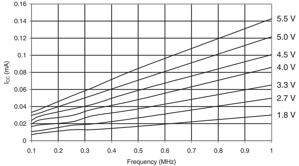
**Figure 30-607.** ATmega6490P: Reset Supply Current vs.  $V_{CC}$  (1 - 20MHz, Excluding Current Through The Reset Pull-up)
