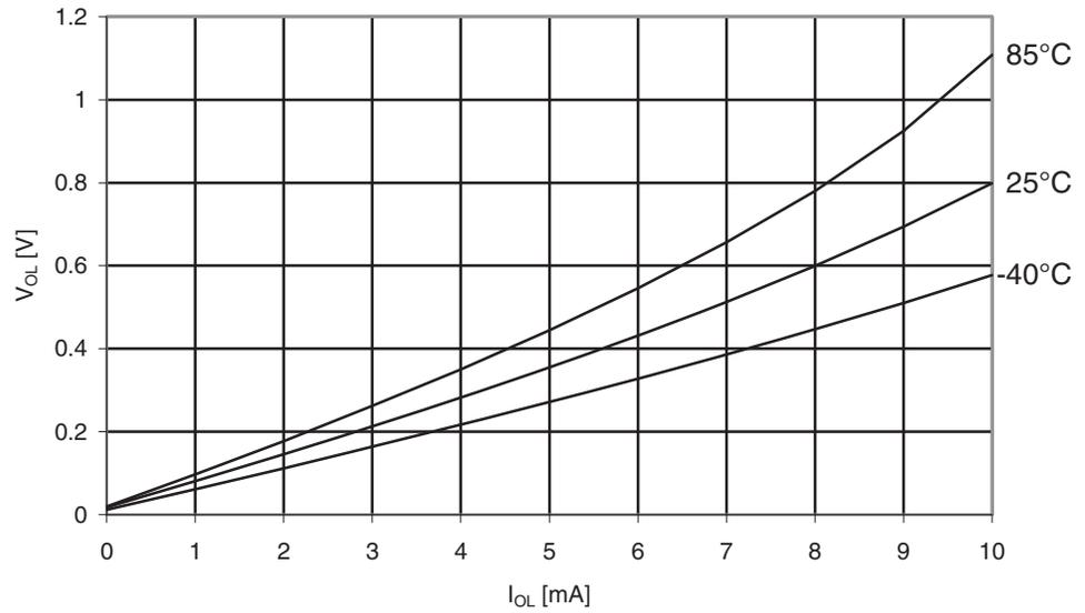
**Figure 30-274.** ATmega3290A: I/O Pin Output Voltage vs. Sink Current, Ports A, C, D, E, F, G
