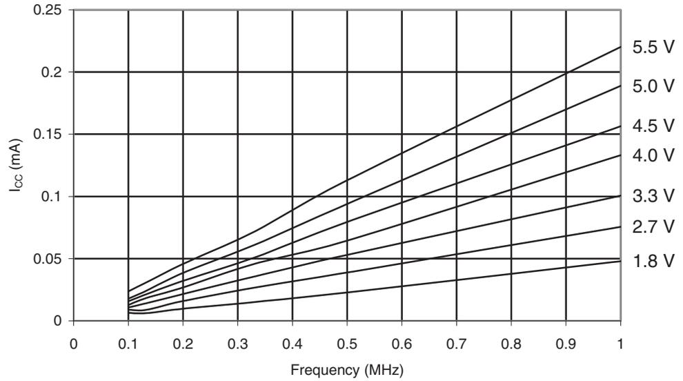
**Figure 30-7.** ATmega169A: Idle Supply Current vs. Frequency (1 - 16MHz)
