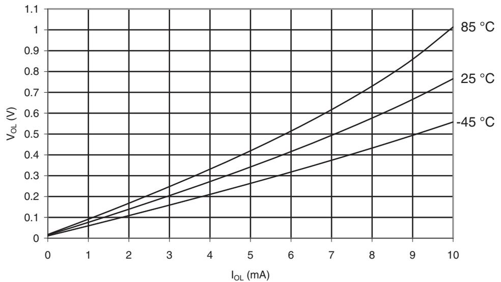
**Figure 30-91.** ATmega169PA. I/O Pin Output Voltage vs. Sink Current, Ports A, C, D, E, F, G
