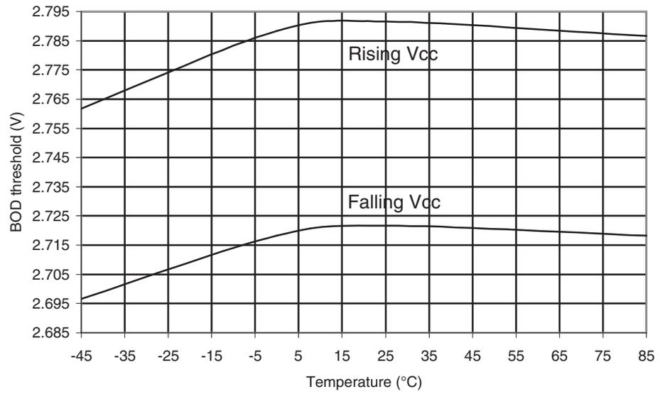
**Figure 30-590.** ATmega6490P: BOD Thresholds vs. Temperature (BOD Level is 1.8V)
