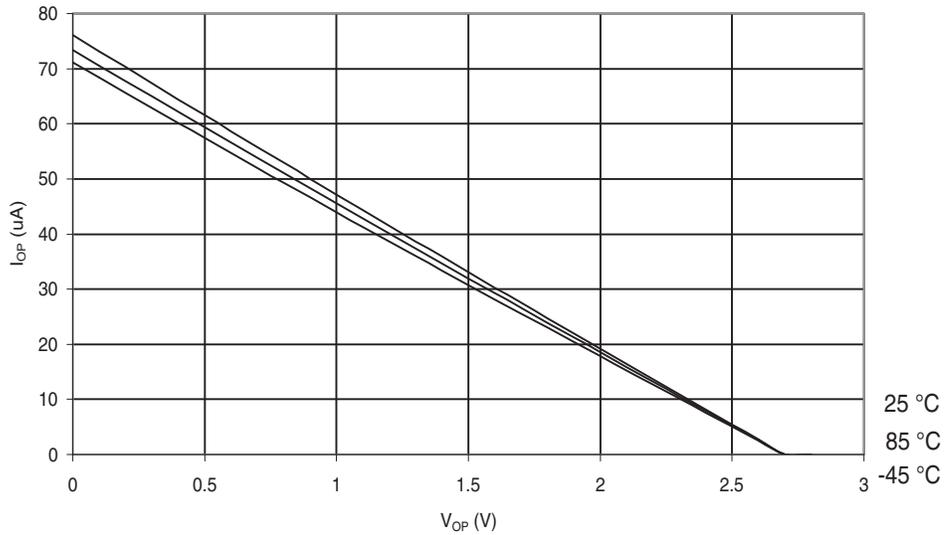
**Figure 30-566.** ATmega6490P: I/O Pin Pull-up Resistor Current vs. Input Voltage ( $V_{CC} = 1.8V$ )
