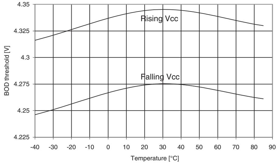
**Figure 30-165.** ATmega329A: BOD Thresholds vs. Temperature (BOD Level is 2.7V)
