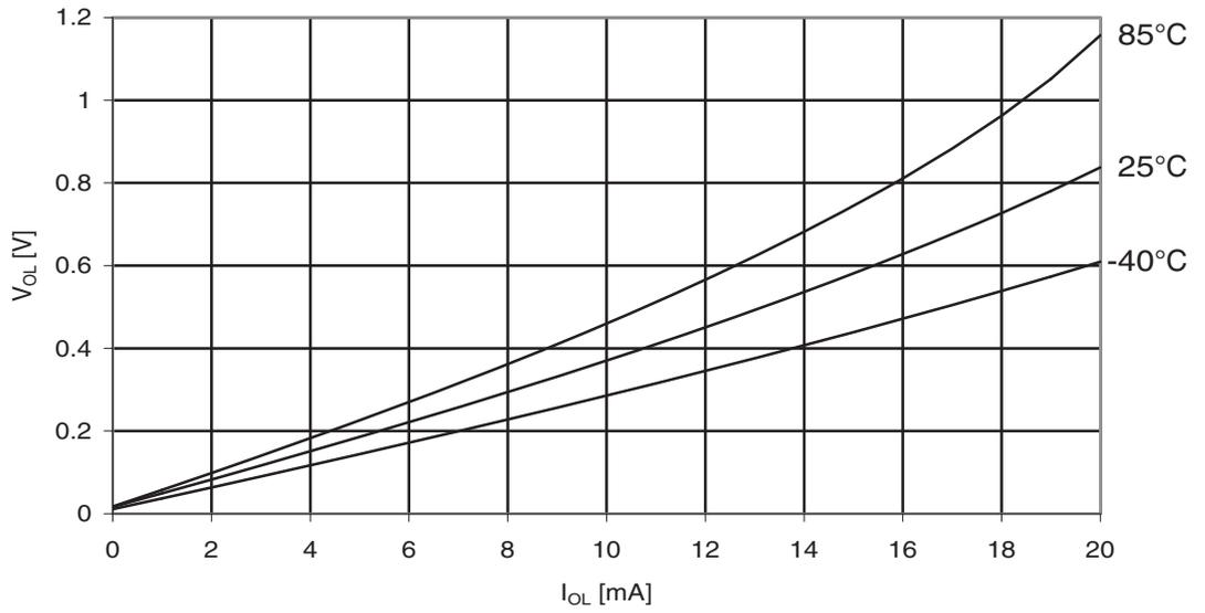
**Figure 30-157.** ATmega329A: I/O Pin Output Voltage vs. Sink Current, Port B ( $V_{CC} = 1.8V$ )
