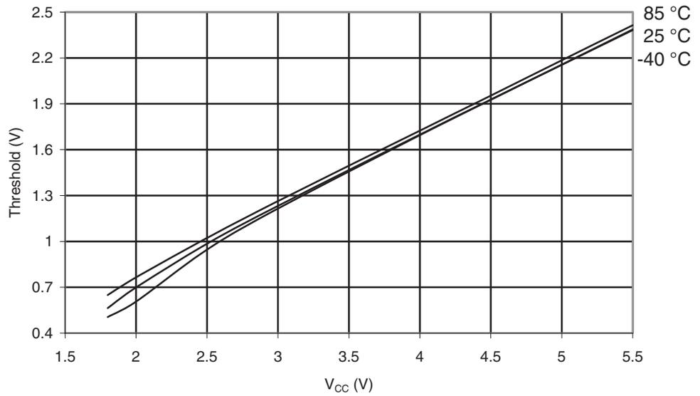
**Figure 30-280.** ATmega3290A: I/O Pin Input Hysteresis vs.  $V_{CC}$
