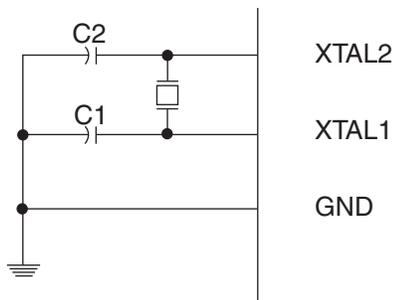
The Oscillator can operate in three different modes, each optimized for a specific frequency range. The operating mode is selected by the fuses CKSEL3..1 as shown in [Table 9-5](#).
