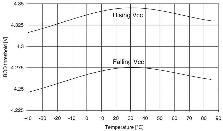
Figure 30-225. ATmega329PA: BOD Thresholds vs. Temperature (BOD Level is 2.7V)
