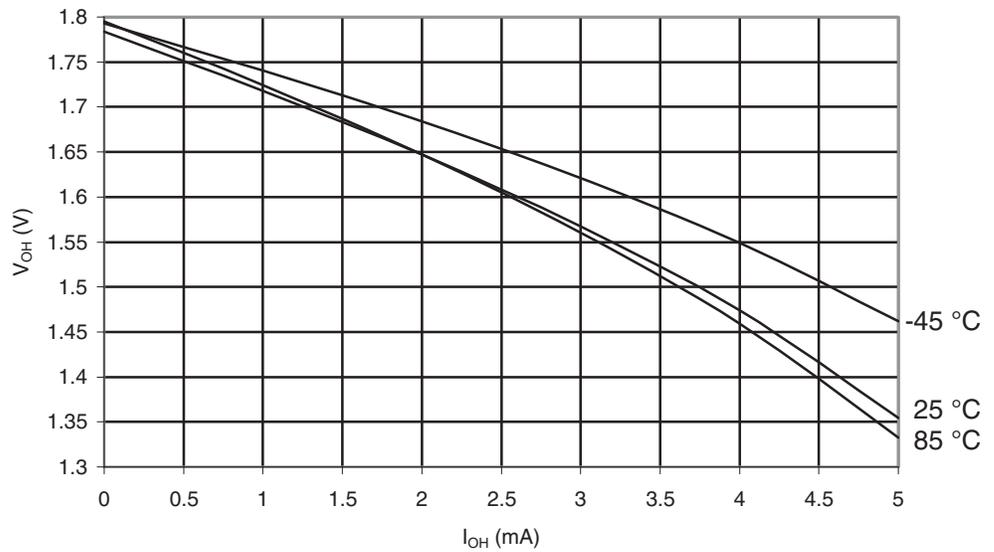
**Figure 30-576.** ATmega6490P: I/O Pin Output Voltage vs. Sink Current, Ports A, C, D, E, F, G ( $V_{CC} = 5V$ )
