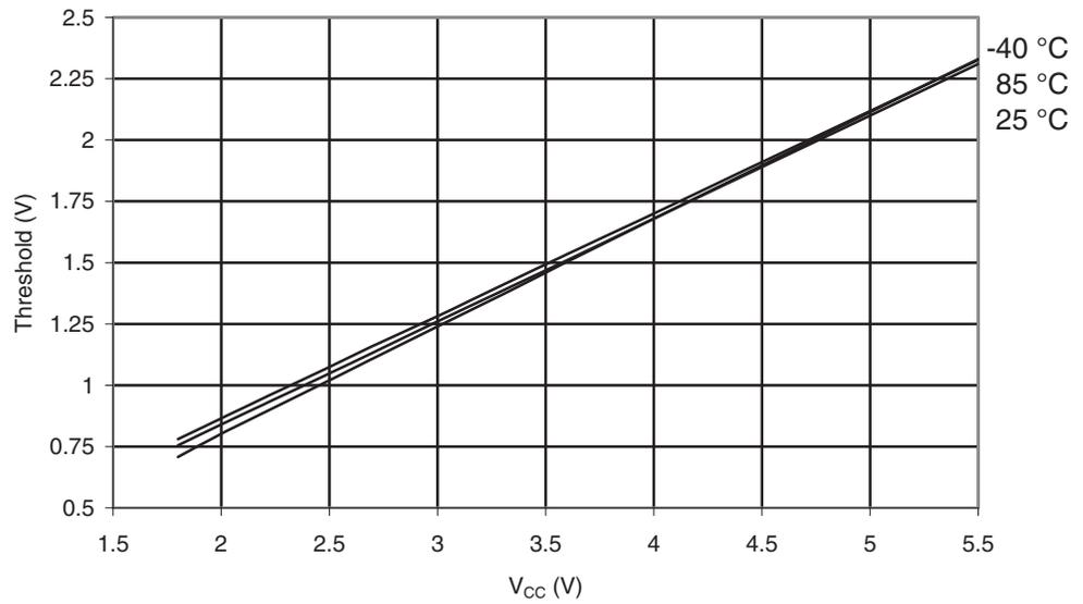
**Figure 30-223.** ATmega329PA: Reset Input Pin Hysteresis vs.  $V_{CC}$
