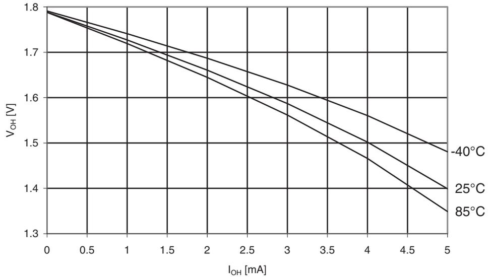
**Figure 30-332.** ATmega3290PA: I/O Pin Output Voltage vs. Sink Current, Ports A, C, D, E, F, G
