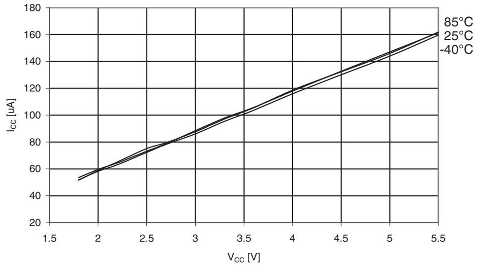
Figure 30-239. ATmega329PA: Watchdog Timer Current vs.  $V_{CC}$
