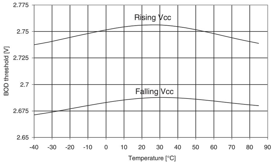
**Figure 30-346.** ATmega3290PA: BOD Thresholds vs. Temperature (BOD Level is 1.8V)
