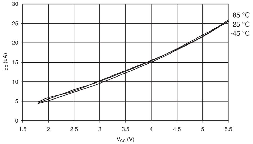
**Figure 30-120.** ATmega169PA: Analog Comparator Current vs.  $V_{CC}$
